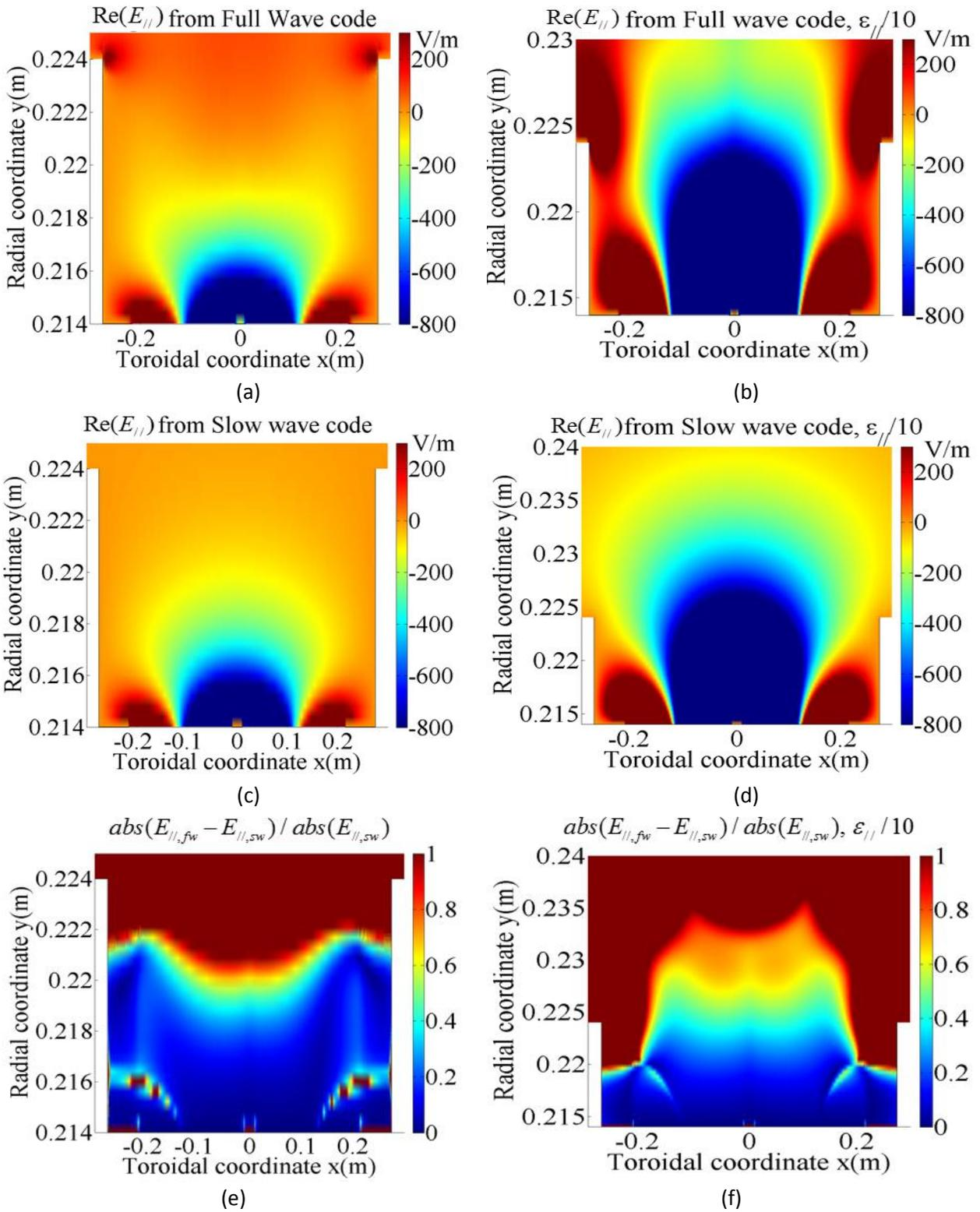
Figure 5.2. Comparison of  $E_{||}$  obtained from two codes. (a), (c), (e) with normal  $\epsilon_{||}$ . (b), (d), (f) uses  $\epsilon_{||}/10$ . (b) and (d) use the field map from (a) and (c) respectively.
