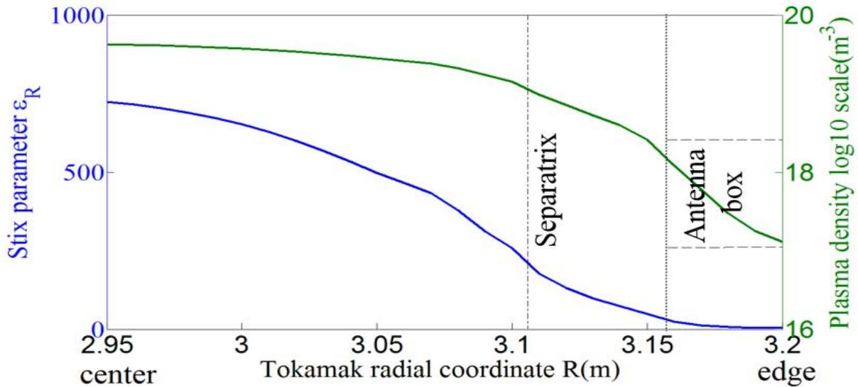
Figure 2.2. Evolution of Stix parameter  $\varepsilon_R$  and plasma density profile from Tore Supra shot 40574 along the radial distance to the Tokamak center. Magnetic tilt angle  $\theta = 0^\circ$  and Tore Supra parameters are used,  $n_x=9.14$ ,  $f=w/2\pi=48\text{MHz}$ ,  $B_0(R_0=2.4)=3.1\text{T}$ , full Deterium plasma
