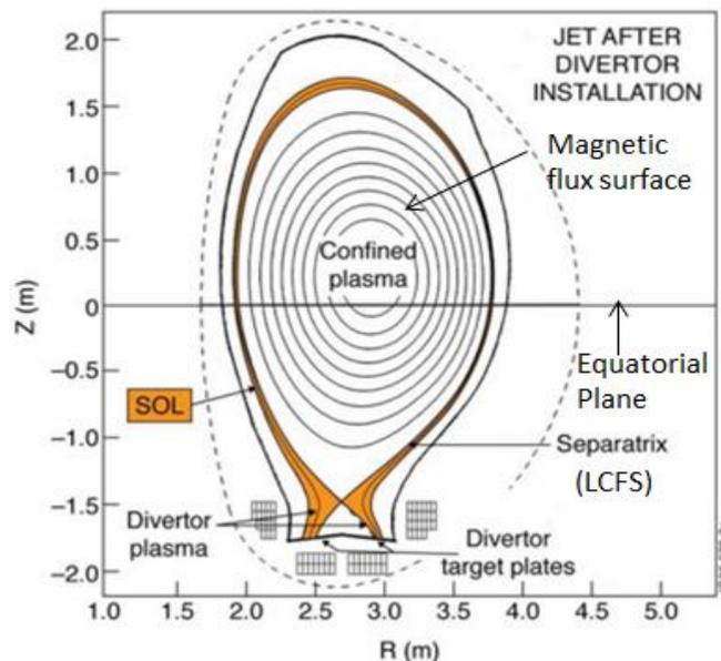
*Figure 1.6. Magnetic flux surface in JET Tokamak*
