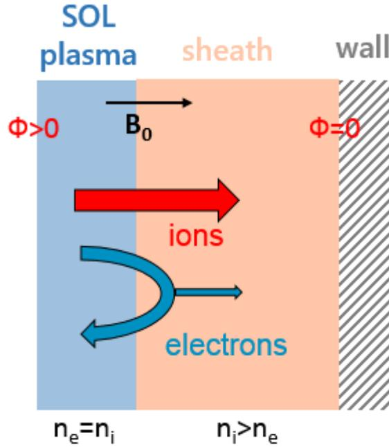
Figure 2.12. A diagram of DC sheath formation
