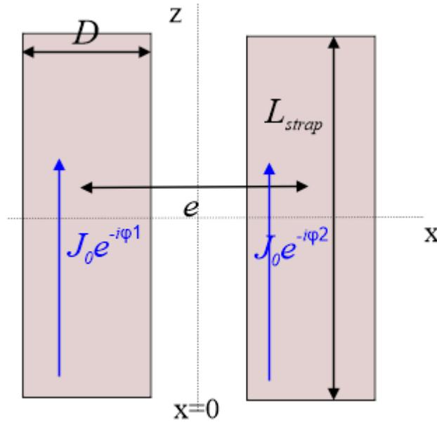
Figure 2.5. A sketch of phased array straps
