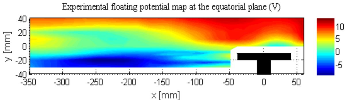
*Figure 5.28. Floating potential map measured by the probe in Aline discharge [Faudot 2016],  $B_0=0.023\text{T}$ ,  $w_0=2.2 \times 10^8 \text{rad/s}$ , gas pressure  $10^{-2} \text{mbar}$ , antenna is grounded as it is in Tokamak*
