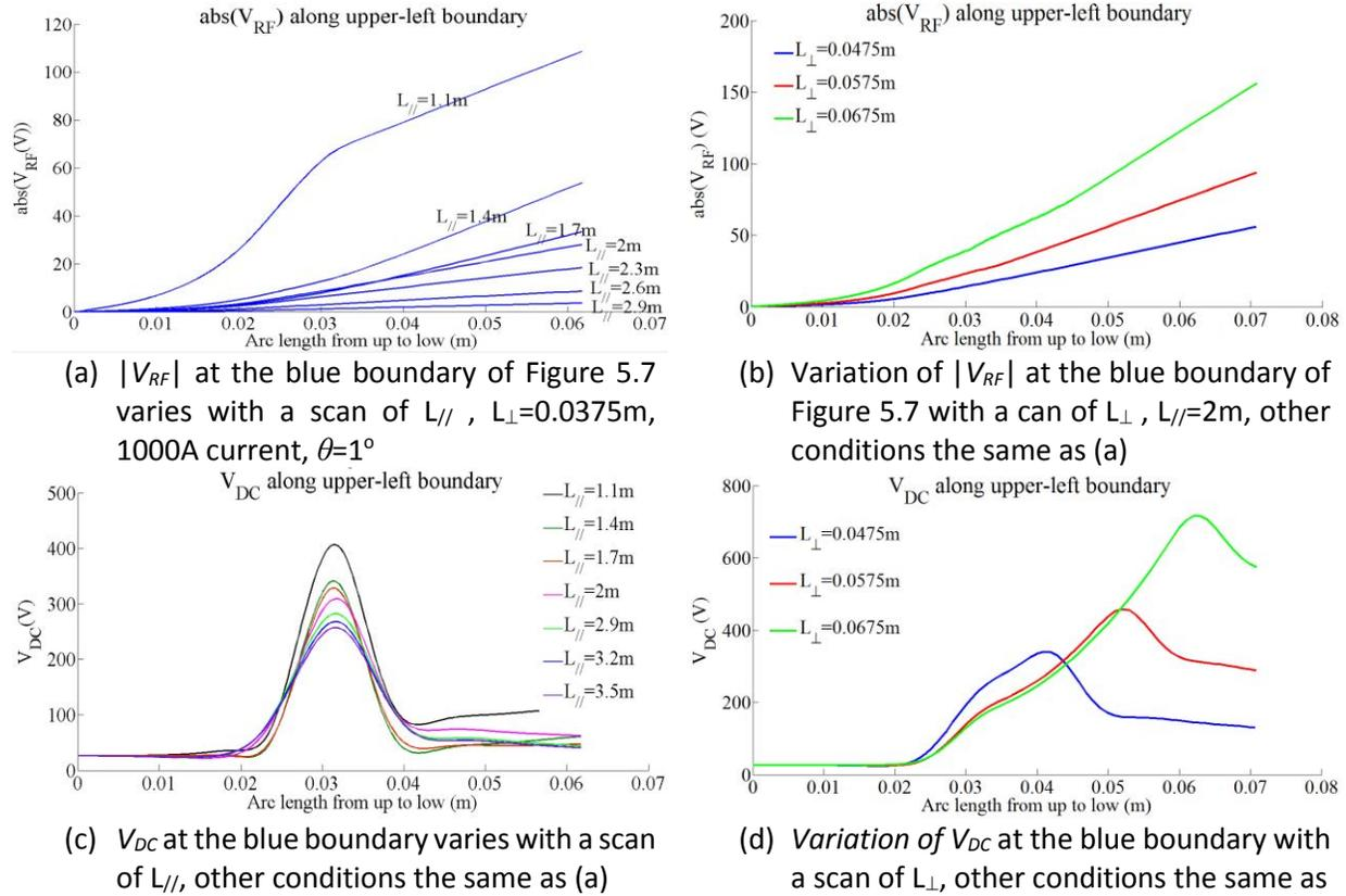
Figure 5.8.  $V_{RF}$  and  $V_{DC}$  behavior with different dimensional lengths; Data were picked up along the blue boundary of Figure 5.7. A constant density  $9 \times 10^{18} \text{m}^{-3}$  at SOL region,  $f_0 = \omega_0 / 2\pi = 48 \text{MHz}$ ,  $B_0(y=0.214\text{m}) = 2.3\text{T}$ ,  $\theta = 1^{\circ}$
