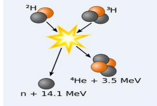
Figure 1.2. A diagram of nuclear fusion reaction
