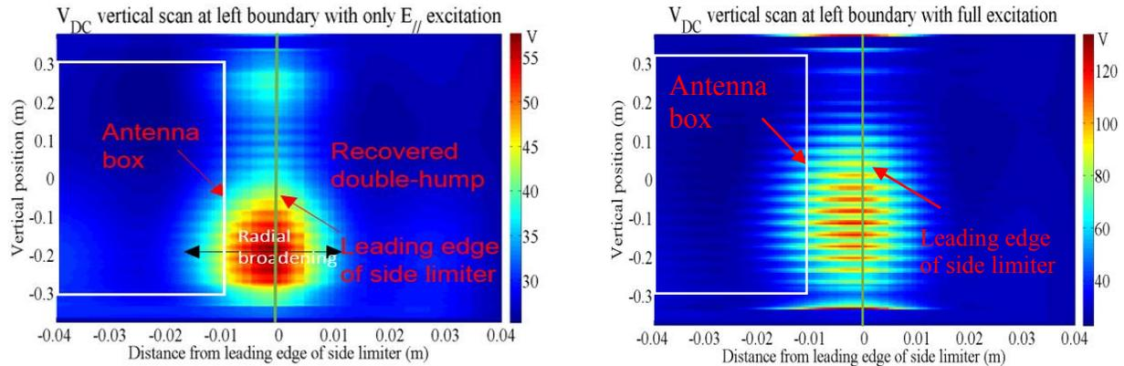
Figure E.2. Vertical-radial map of  $V_{DC}$  at the edge of the left side limiter by SSWICH-FW/RAPLICASOL simulations using multiple-2D approach, with only  $E_{\parallel}$  excitation (left), with full excitation (right). The simulation did not include the 3D effect
