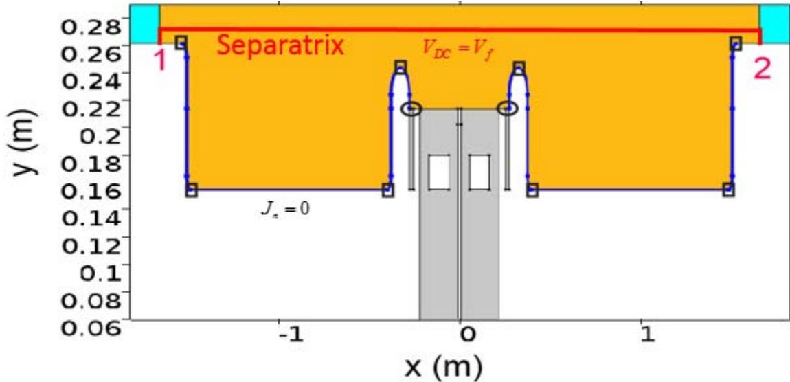
*Figure 4.5. Simulation geometry in  $V_{RF}$  and  $V_{DC}$  modules.  $V_{RF}$  solved along 1D sheath boundaries, whereas  $V_{DC}$  solved in the 2D SOL domain. The orange color indicates the plasma region; Grey is the vacuum region. Rectangle and ellipse are the boundary points where the RF sheath boundary condition applied in the two approaches; The two identities are the DC sheath boundary condition imposed at the corresponding lines*
