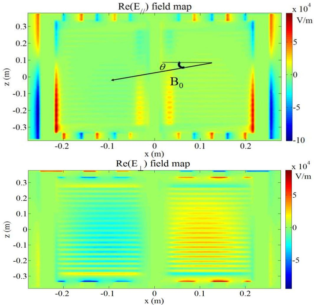
*Figure 5.16. 2D field map generated at the Faraday screen of the 3D RPLICASOL code; Up: the real part of the parallel component; Bottom: the real part of the perpendicular component (the one perpendicular to the radial direction).*
