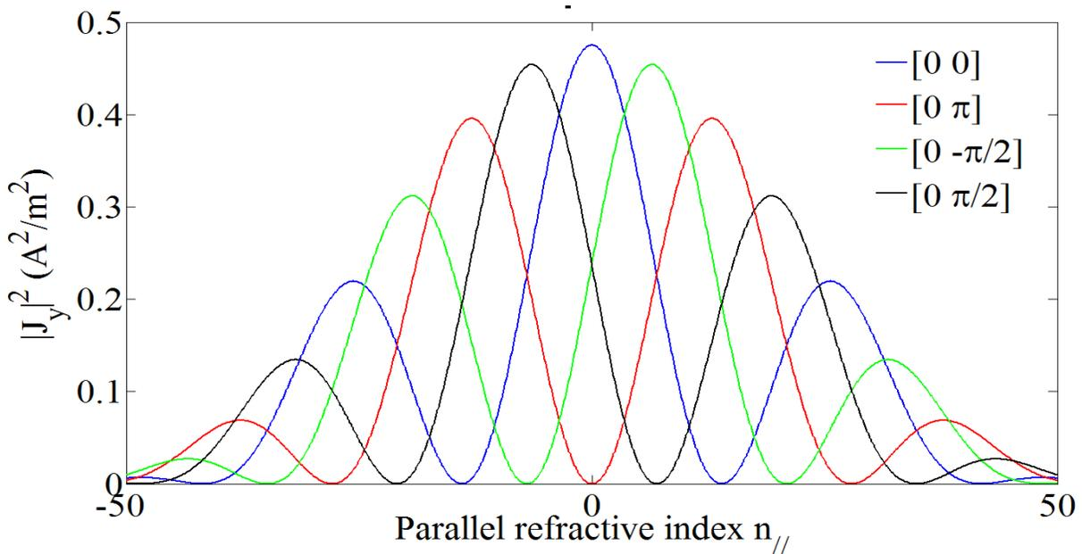
*Figure 2.6. Current spectrum with different current phasings. Tore Supra classical antenna parameters are used,  $D=0.109\text{m}$ ,  $e=0.224\text{m}$ , wave frequency  $f=\omega/2\pi=48\times 10^6\text{Hz}$ ,  $J_0=10\text{A/m}$*
