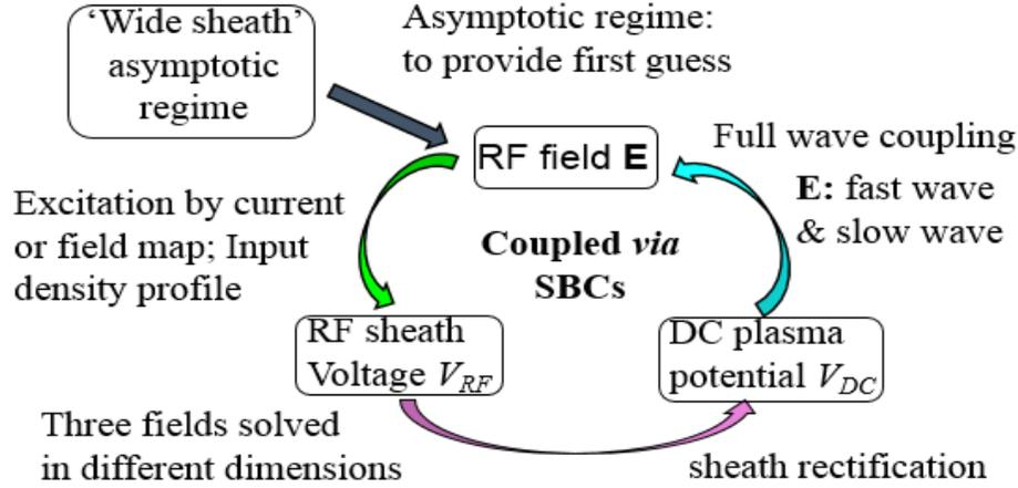
Figure 4.4. Work flow of the 2D SSWICH-FW code
