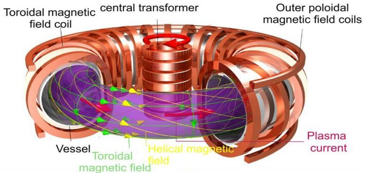
*Figure 1.3. Tokamak structure and its magnetic field configuration*
