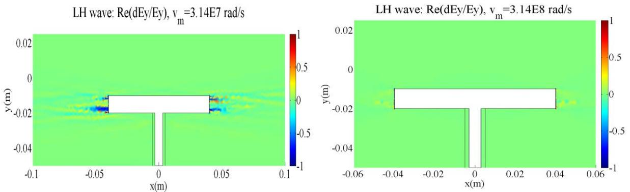
Figure 5.26. Relative variations of  $E_y$  of the LH wave with different dissipation,  $dE_y/E_y = (E_y(1\text{mm}) - E_y(2\text{mm}))/E_y(2\text{mm})$ , zoom in the antenna region; Left: collision frequency  $\nu_m = 3.14 \times 10^7$  rad/s; Right  $\nu_m = 3.14 \times 10^8$  rad/s
