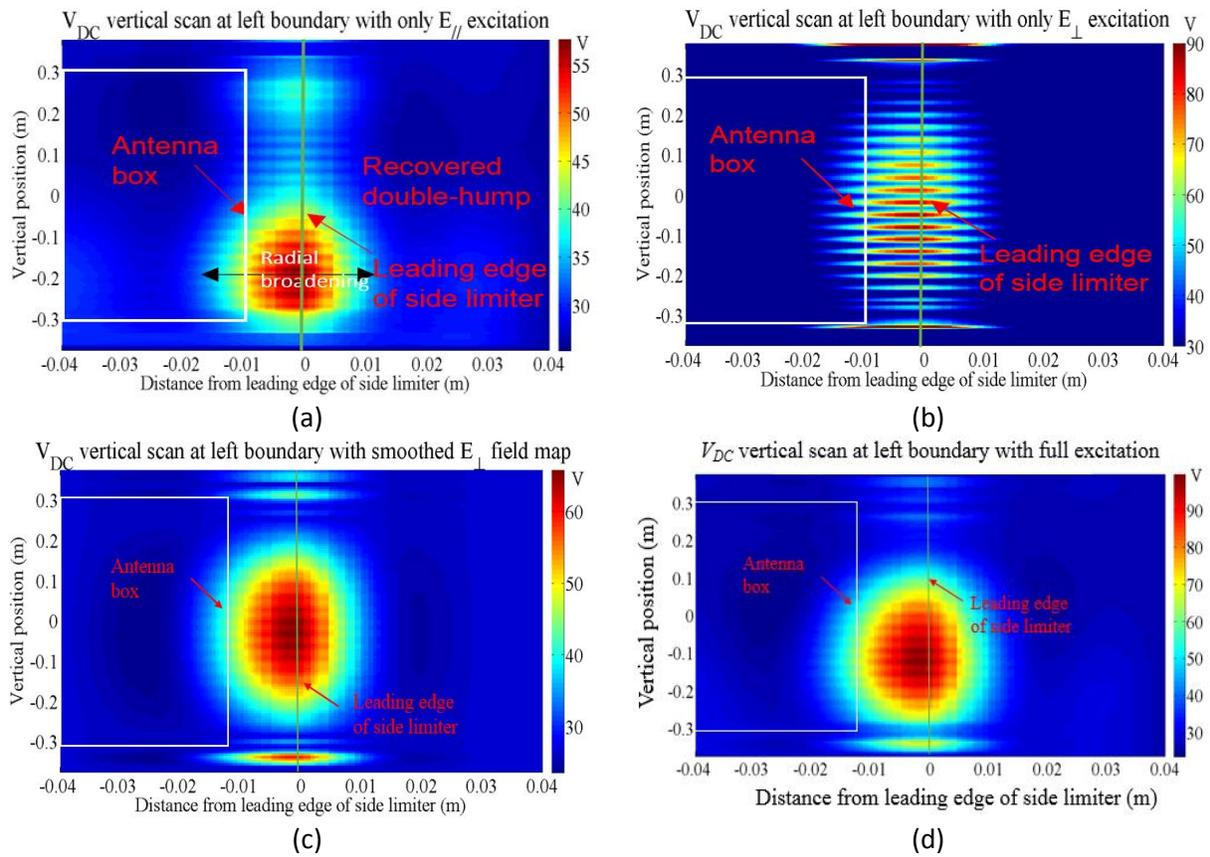
*Figure 5.17.  $V_{DC}$  vertical scan using field map containing  $E_{//}$  only (a),  $E_{\perp}$  only (b), smoothed  $E_{\perp}$  only (c) and both  $E_{//}$  and non-smoothed  $E_{\perp}$  (d). Data picked up at the green line of [Figure 5.15](#) (Left)*
