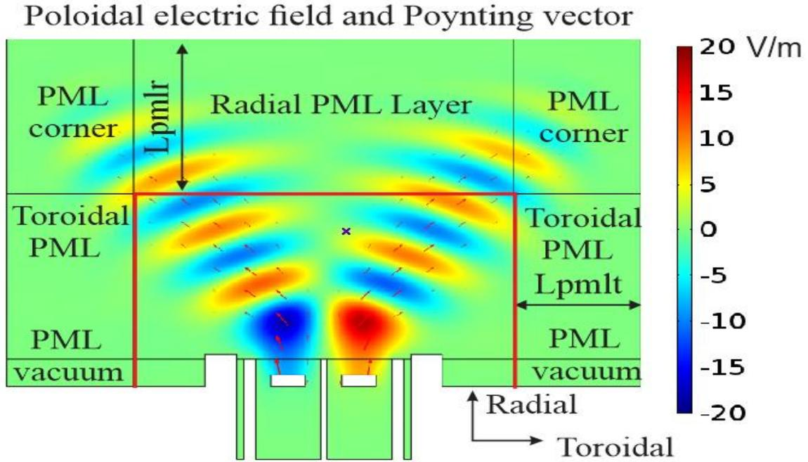
Figure 3.5. 2D map of real part of poloidal electric field in dipole phasing with  $\theta=0^\circ$ . Arrows represent the Poynting Vector. Density 0 is used in the antenna box. Red lines are defined for the power measurement propose.  $L_{pmlt}=L_{pmlr}=0.4m$ .
