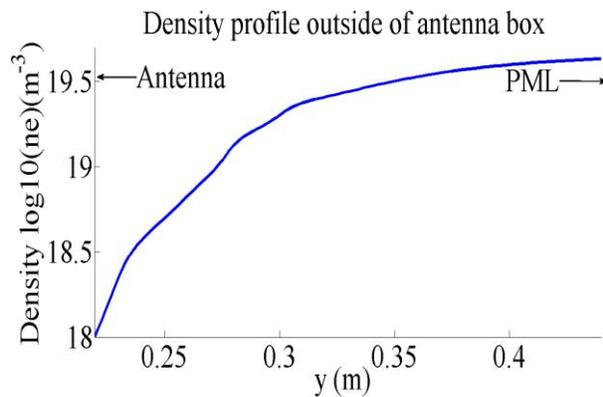
*Figure 3.3. Density profiles above the antenna, from TS 40574*
