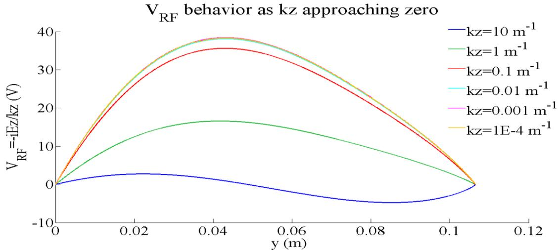
*Figure 5.18. Convergence of  $V_{RF}$  with tapered  $kz$ . Data are picked up at the left far SOL boundary,  $\theta=7^\circ$ ,  $\text{freq}=57\text{MHz}$ , central magnetic field  $B_0=3.87\text{T}$ , a constant density  $n_e=1.6\times 10^{19}\text{ m}^{-3}$  is used below the Separatrix*
