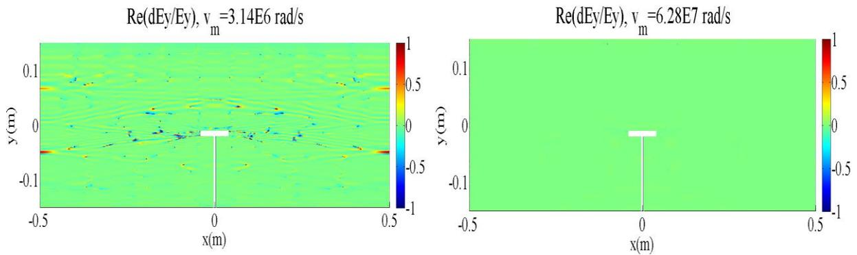
Figure 5.25. Relative variations of  $E_y$  of the Helicon wave with different dissipation;  $dE_y/E_y = (E_y(1\text{mm}) - E_y(2\text{mm}))/E_y(2\text{mm})$ ; Left: collision frequency  $\nu_m = 3.14 \times 10^6$  rad/s; Right  $\nu_m = 6.28 \times 10^7$  rad/s
