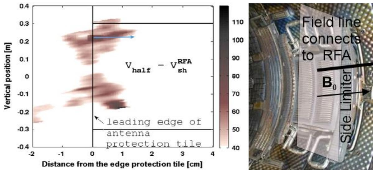
*Figure 2.18. Left: Measurement from retarding field analyzer in Tore Supra, cite from [Kubic 2013] Right: ICRF antenna front face, and field line trajectory from the leading edge of the side limiter to RFA. Shading parallelogram is the plane where the 2D measurement (left) represents for.*
