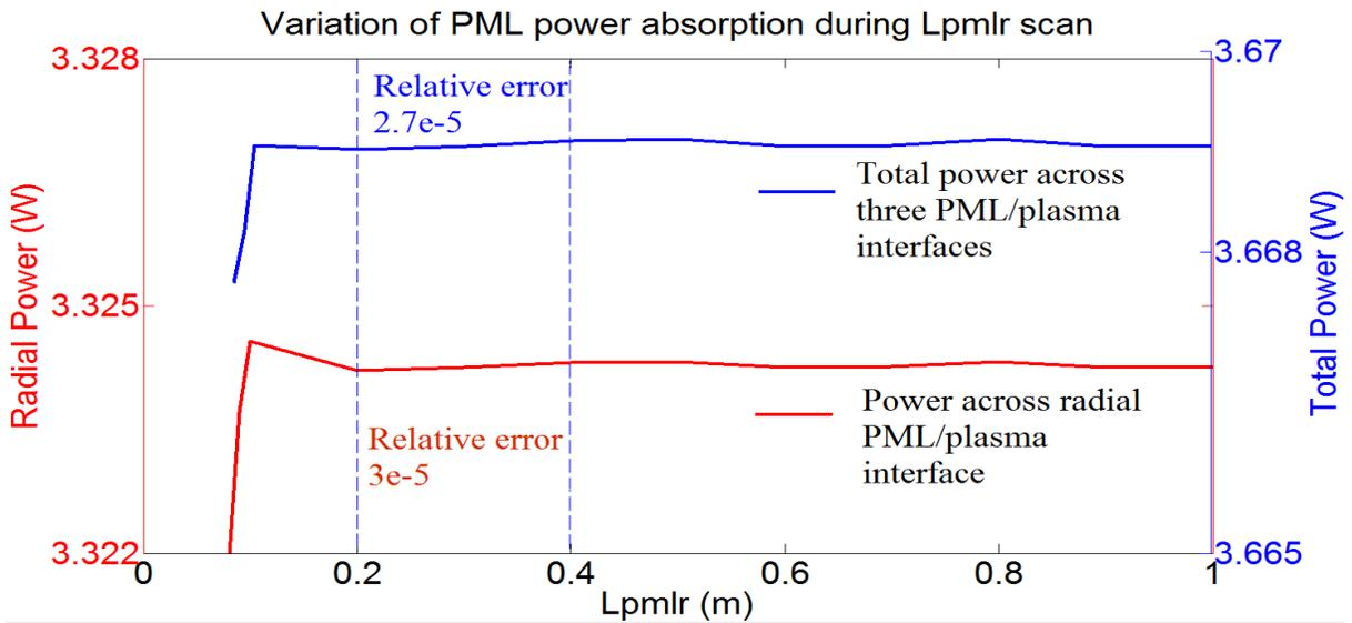
Figure 3.6. A scan of radial PML depth with  $\theta=7^\circ$ , toroidal PML depth at 0.4m. Criterion PML depth is found at 0.4m, where relative error goes below  $1 \times 10^{-4}$
