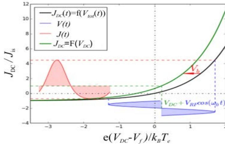
Figure 2.16. An illustration of DC sheath rectification
