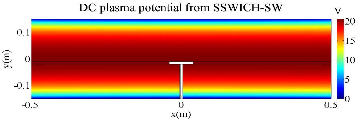
Figure 5.29. DC plasma potential map from 2D SSWICH-SW simulation, density Figure 5.22,  $T_e=5\text{eV}$ ,  $T_i=0.026\text{eV}$ ,  $\nu_m=10^7\text{ rad/s}$ ,  $\nu_i=5.2\times 10^5\text{ rad/s}$ ,  $B_0=0.023\text{T}$ ,  $\omega_0=2.2\times 10^8\text{ rad/s}$
