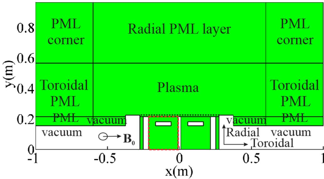
Figure 3.2. Schematic view of 2D RAPLICASOL code in the case of a tilted  $B_0$  in poloidal ( $z$ ) direction. The computational area is shown in green. Dashed line is the antenna mouth. The red dashed rectangle represents one of the two individual boxes that consists the antenna box.
