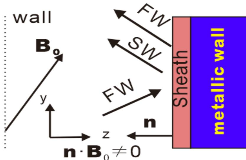
*Figure 2.19. Mode conversion mechanism under tilted magnetic configuration*
