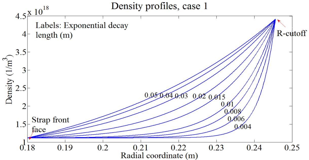
Figure 3.21. A scan of density profiles in the evanescence region,  $\theta = 0^\circ$ , dipole phasing, plasma filled antenna,  $n_{ref} = 1.1164 \times 10^{18} \text{ m}^{-3}$  and  $y_{ref} = 0.18 \text{ m}$
