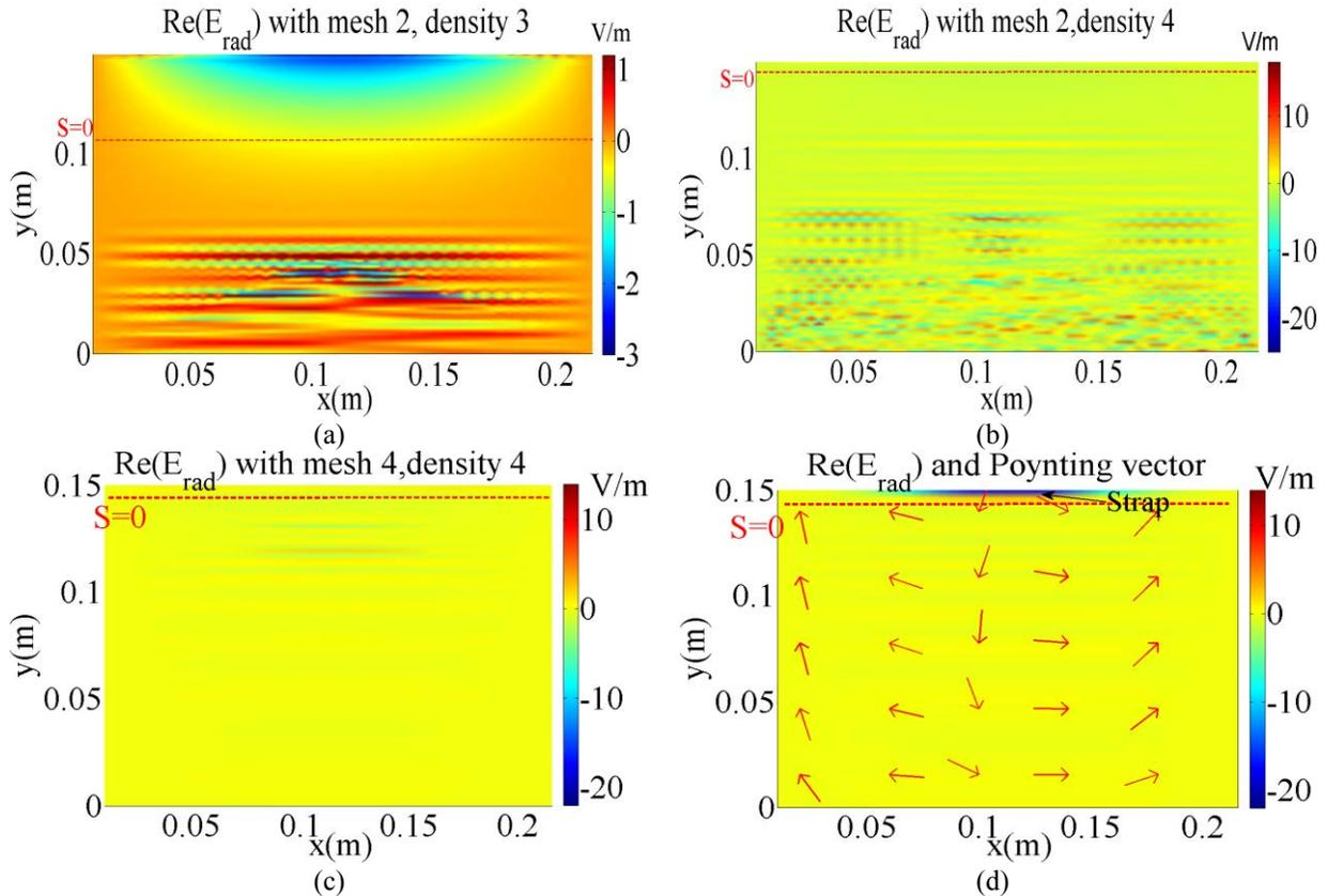
**Figures 3.16.** (a)-(b). Real part of the radial electric field with different density profiles, but the same mesh. Dipole phasing,  $\theta = 0^\circ$ . (c). the same simulation as (b) but with mesh 4. (d) Radial electric field, using density 4, the same mesh size as mesh 4 but with square grid, instead of triangle. Red arrows indicate the normalized real part of the Poynting vector
