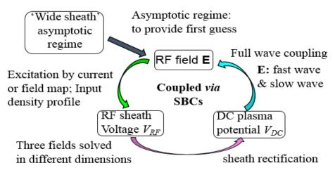
Figure 4.4. Work flow of the 2D SSWICH-FW code
