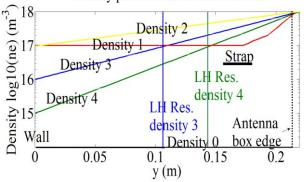
Figure 3.4. Density profiles inside the antenna box. Vertical solid lines indicate the locations of the LH resonance. Vertical dot line specifies the edge of the antenna box.
