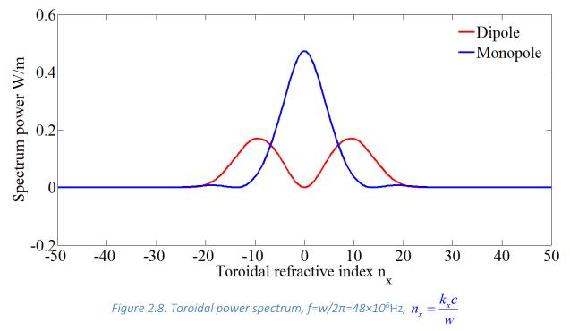
A graph of the power spectrum of the monopole phasing and dipole phasing is shown in *Figure 2.8*. The electromagnetic fields are taken from the plasma stands radially 50cm away from the straps. The
