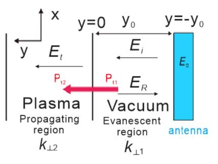
Figure 2.7. A simple three-wave coupling model
