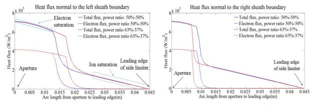
Figure 5.20. Heat flux at the curved boundaries of the private SOL, data picked up at the red boundaries of Figure 5.15 (Left),  $\theta = 7^{\circ}$ , z=-0.2m
