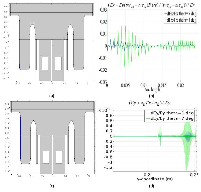
Figure 4.12. Test of the accuracy of the sheath boundary condition at the boundaries. (a) an example of curved boundary; (b) relative error of COMSOL returned Ex at boundary (a) with Ex required by the sheath boundary condition that is imposed at boundary (a) under two magnetic tilt angles; (c) an example of flat boundary; (d) relative error of COMSOL returned Ex at boundary (c) with Ex required by the sheath boundary condition that is imposed at boundary (c) under two magnetic tilt angles
