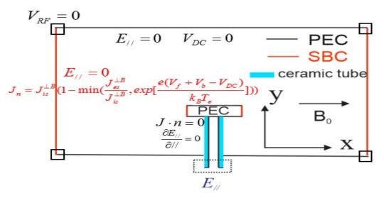
Figure 4.14. Boundary conditions used in SSWICH-SW simulation for Aline
