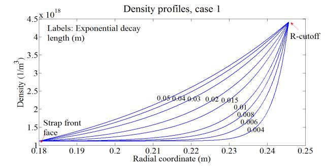
Figure 3.21. A scan of density profiles in the evanescence region, theta= $0^{\circ}$ , dipole phasing, plasma filled antenna, n\_ref =1.1164e18m<sup>-3</sup> and y\_ref =0.18m
