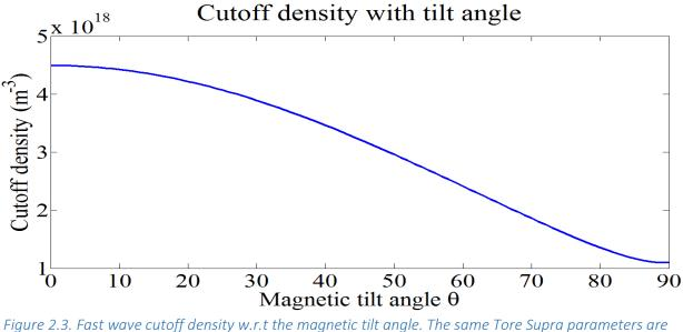
e 2.3. Fast wave cutojj density w.r.t the magnetic tilt angle. The same Tore Supra paramete used as Figure 2.2
