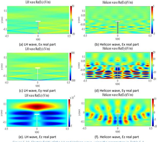
Figure 5.23. Electric fields of the LH and Helicon wave, using the parameters in Table 5-1
