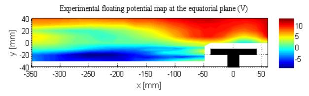
Figure 5.28. Floating potential map measured by the probe in Aline discharge [Faudot 2016],  $B_0$ =0.023T,  $w_0$ =2.2×10<sup>8</sup>rad/s, gas pressure 10<sup>-2</sup>mbar, antenna is grounded as it is in Tokamak
