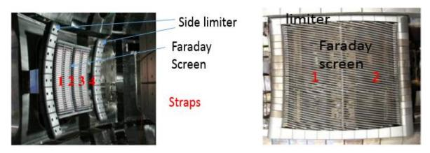
Figure 1.9. 4 straps ICRH antenna in the KSTAR Tokamak (left); 2 straps ICRH antenna in the ASDEX-Upgrade Tokamak (right)
