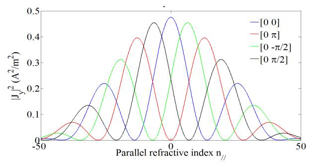
Figure 2.6. Current spectrum with different current phasings. Tore Supra classical antenna parameters are used, D=0.109m, e=0.224m, wave frequency  $f=w/2\pi=48\times10^6$ Hz, J<sub>0</sub>=10 A/m
