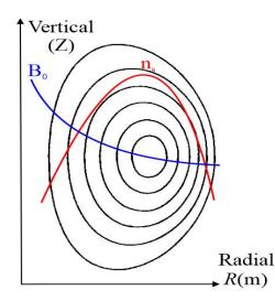
Figure 1.5. Magnetic flux surface in the central plasma, view inside a poloidal cross section. Red curve indicates a typical profile of the plasma density; The blue curve represents the magnetic field profile.
