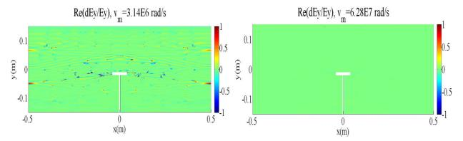
Figure 5.25. Relative variations of Ey of the Helicon wave with different dissipation; dEy/Ey=(Ey(1mm)-Ey(2mm))/Ey(2mm); Left: collision frequency  $v_m=3.14\times10^6$  rad/s; Right  $v_m=6.28\times10^7$  rad/s
