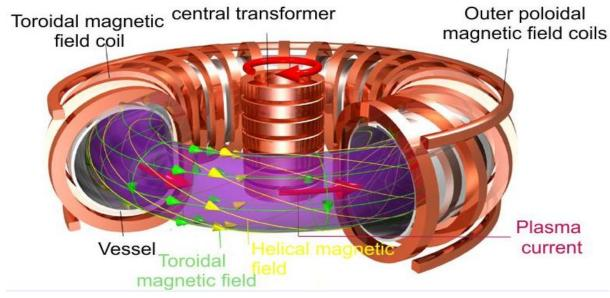
Figure 1.3. Tokamak structure and its magnetic field configuration
