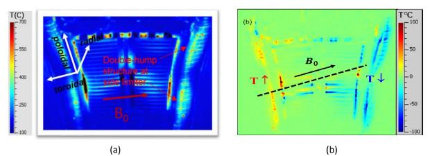
Figure 5.12 (a): infrared picture of active ToreSupra ICRF antenna [Corre 2012] shows a double-hump structure at the side limiters (b) differential IR image from subtraction of two RF pulses, where the RF generator power balance is changed from (50% / 50%) to (63% / 37%)[Colas 2013]
