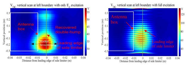
Figure E.2. Vertical-radial map of  $V_{DC}$  at the edge of the left side limiter by SSWICH-FW/RAPLICASOL simulations using multiple-2D approach, with only  $E_{//}$  excitation (left), with full excitation (right). The simulation did not include the 3D effect
