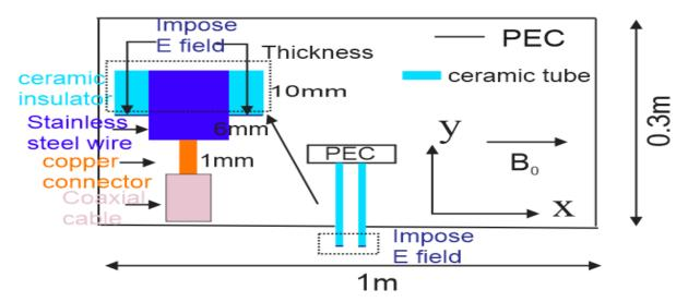
Figure 4.13. 2D SSWICH-FW geometry for Helicon wave Simulations. The feeder structure inserted on the left side is a zoom in the region indicated by the black rectangle;
