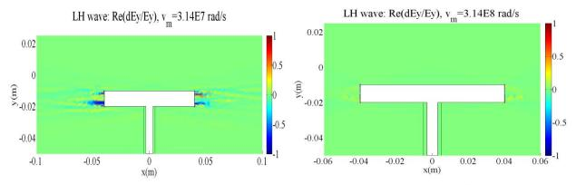
Figure 5.26. Relative variations of Ey of the LH wave with different dissipation, dEy/Ey=(Ey(1mm)-Ey(2mm))/Ey(2mm), zoom in the antenna region; Left: collision frequency  $v_m=3.14\times10^7$  rad/s; Right  $v_m=3.14\times10^8$  rad/s
