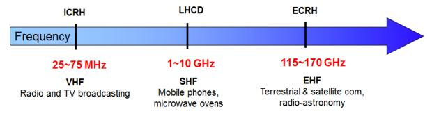
Figure 1.7. Diagram of frequency range of three auxiliary heating and current drive waves
