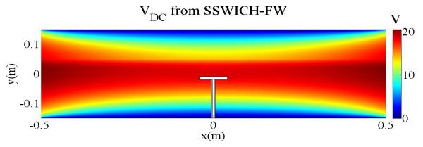
Figure 5.32. DC plasma potential map from 2D SSWICH-FW simulation using spectral approach,  $k_z=0.001m^{-1}, \theta=0.01^{\circ}$ , other plasma parameters are the same as Figure 5.31
