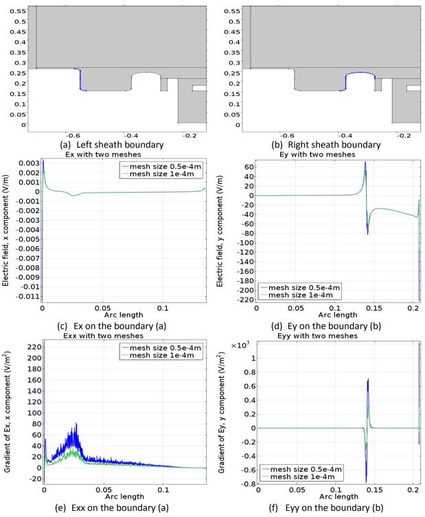
Figure 4.10. A plot of electric field and its derivatives along sheath boundaries, theta=7°; Arc length from left to right
