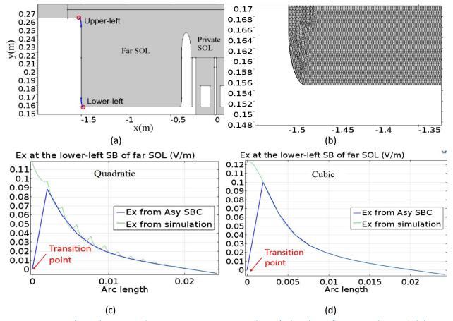
Figure 4.7. Solving the vectorial wave equation using quadratic/cubic shape functions, theta=7°. (a)
