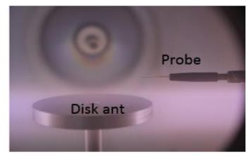
Figure 1.15. Disk antenna and Langmuir probe inside vacuum chamber, cite from [Faudot 2015]
