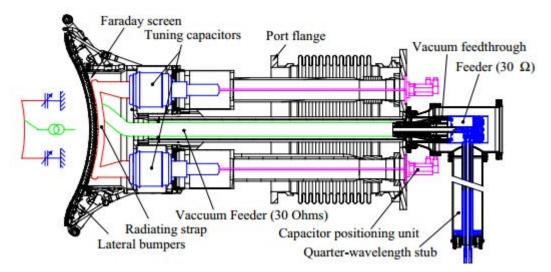
Figure 1.10. Layout of the standard ICRH wave launcher on Tore Supra, cite from [Vulliez 2003]
