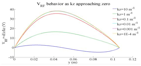
Figure 5.18. Convergence of  $V_{RF}$  with tapered kz. Date are picked up at the left far SOL boundary,  $\theta$ =7°, freq=57MHz, central magnetic field  $B_0$ =3.87T, a constant density ne=1.6×10<sup>19</sup> m<sup>-3</sup> is used below the Separatrix
