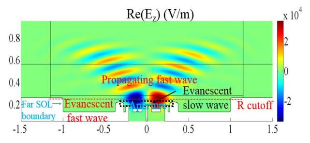
Figure 5.1. The real part of the poloidal electric field obtained in SSWICH-FW under TS configuration. The R-cutoff layer is shown by red dot line. The private SOL is enclosed by black dot rectangle. At its bottom, it is the antenna aperture.
