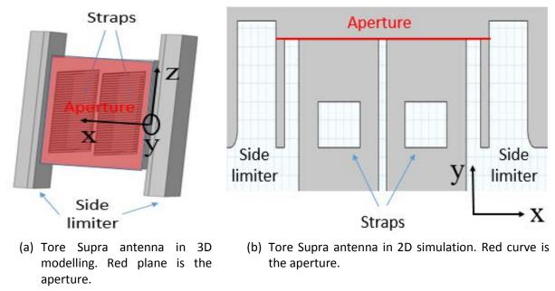
Figure 2.10. Typical choices of the aperture in the 3D and 2D simulation
