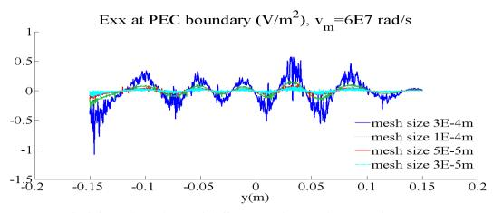
Figure 5.27. Exx at the left PEC boundary with different mesh sizes, the same plasma parameters is used as Figure 5.23(b)
