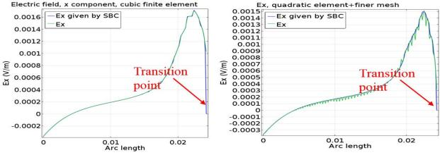
Using cubic finite element, mesh size in sheath region; 1e-3m. Total memory 40Gb, solution time 5mins
