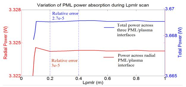
Figure 3.6. A scan of radial PML depth with  $\theta$ =7°, toroidal PML depth at 0.4m. Criterion PML depth is found at 0.4m, where relative error goes below 1×10<sup>-4</sup>
