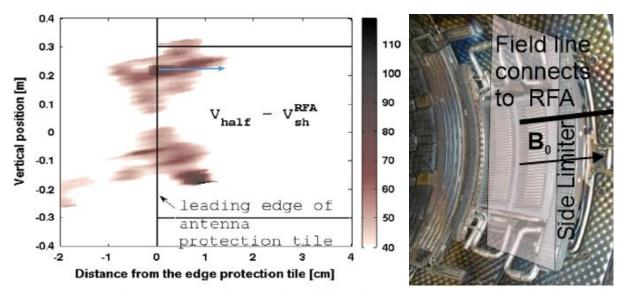
Figure 2.18. Left: Measurement from retarding field analyzer in Tore Supra, cite from [Kubic 2013] Right: ICRF antenna front face, and field line trajectory from the leading edge of the side limiter to RFA. Shading parallelogram is the plane where the 2D measurement (left) represents for.
