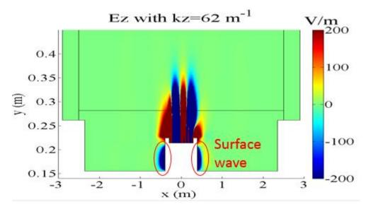
Figure 5.19. Excitation of surface wave in the far SOL under a high kz, other parameters are the same as Figure 5.18
