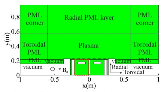
Figure 3.2.Schematic view of 2D RAPLICASOL code in the case of a tilted  $B_0$  in poloidal (z) direction. The computational area is shown in green. Dashed line is the antenna mouth. The red dashed rectangle represents one of the two individual boxes that consists the antenna box.
