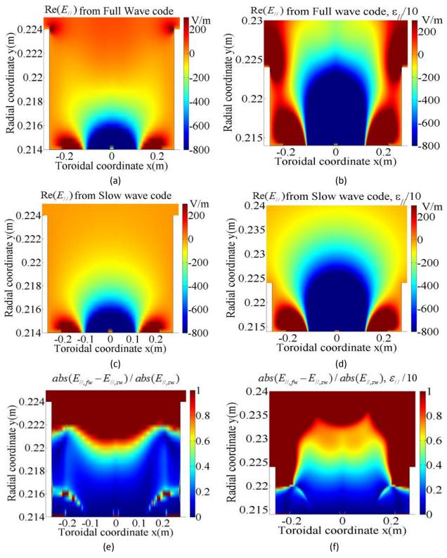
Figure 5.2. Comparison of  $E_{//}$  obtained from two codes. (a) , (c), (e) with normal  $\varepsilon_{_{//}}$  . (b), (d), (f) uses  $\varepsilon_{_{//}} / 10$ . (b) and (d) use the field map from (a) and (c) respectively.
