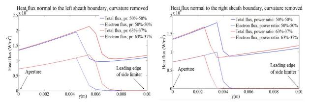
Figure 5.21. Heat flux at the vertical boundaries of the private SOL; Data picked up at the red boundaries of Figure 5.15 (Right),  $\theta = 7^{\circ}$ , z=-0.2m
