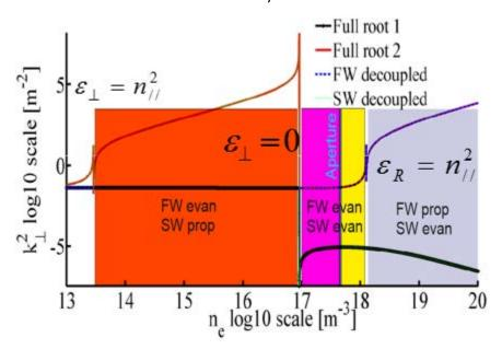
Figure 2.4. A drawing of the dispersion relations of the fast wave and the slow wave in a range of plasma densities and the propagation/evanescence regions for these two waves. Following parameters are used, frequency 48MHz, magnetic field  $B_0=2.32T$  at  $n_e=10^{18}m^{-3}$ , parallel wave number  $k_{//}=5 m^{-1}$ , Deuterium plasma
