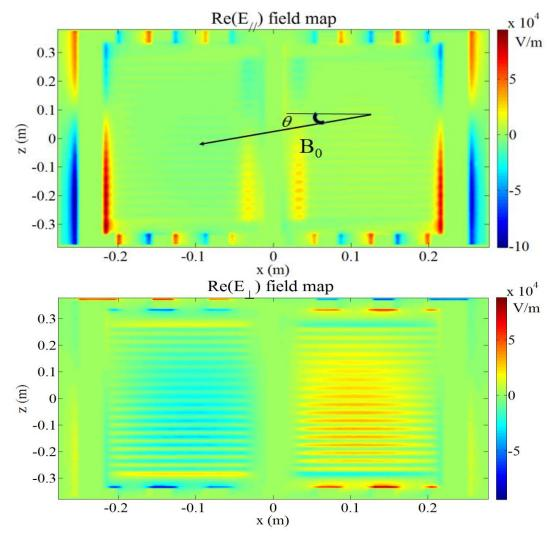
*Figure 5.16. 2D field map generated at the Faraday screen of the 3D RAPLICASOL code; Up: the real part of the parallel component; Bottom: the real part of the perpendicular component (the one perpendicular to the radial direction).*
