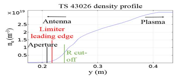
Figure 5.14. Radial density profile and its relative location in the code, data from TS shot 43026
