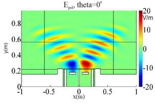
Figure 3.9. Real part of the poloidal electric field, theta=0°, mesh 2, density 3, dipole phasing
