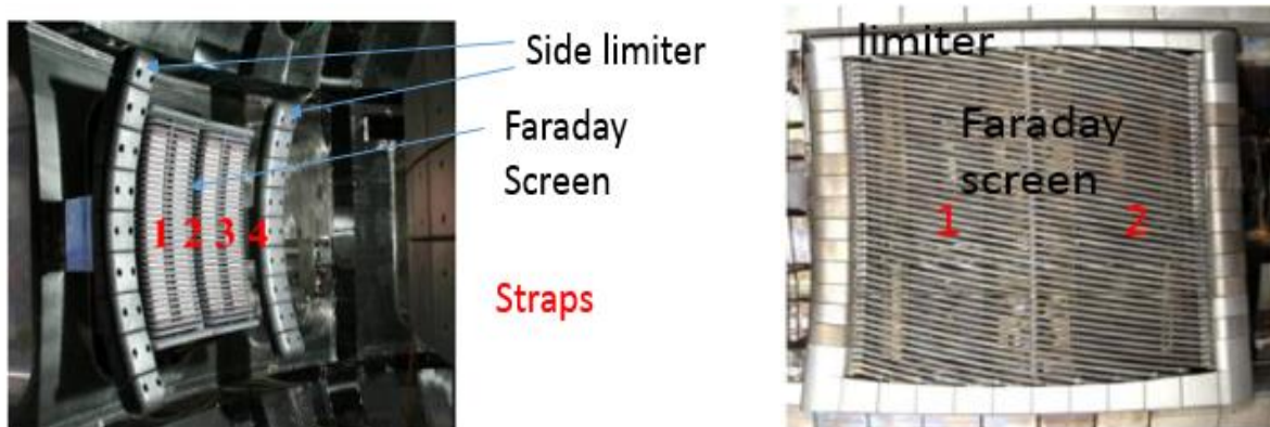
Figure 1.9. 4 straps ICRH antenna in the KSTAR Tokamak (left); 2 straps ICRH antenna in the ASDEX-Upgrade Tokamak (right)
