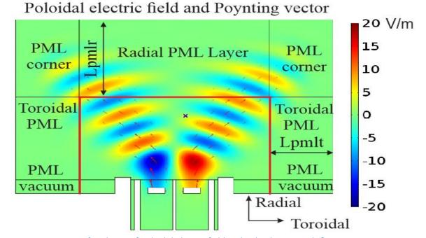
Figure 3.5. 2D map of real part of poloidal electric field in dipole phasing with  $\theta$ =0°. Arrows represent the Poynting Vector. Density 0 is used in the antenna box. Red lines are defined for the power measurement propose. Lpmlt=Lpmlr=0.4m.
