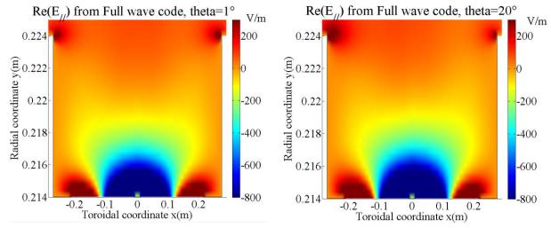
Figure 5.6. The real part of  $E_{II}$  from Full wave code with two magnetic tilt angles
