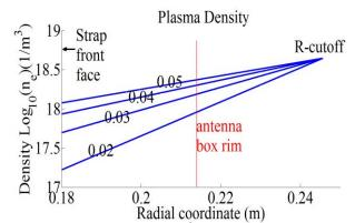
Figure 3.23. Test density profiles in the fast wave evanescence region, theta=0°. Labels indicate the exponential decay length L in meter
