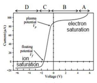
Figure 2.13. Probe I/V characteristic
