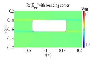
Figure 3.13. Toroidal electric field in the antenna strap region surrounded by rectangle in Figure 3.11, with hyperbolic cosine distribution of RF current over straps with rounded corners
