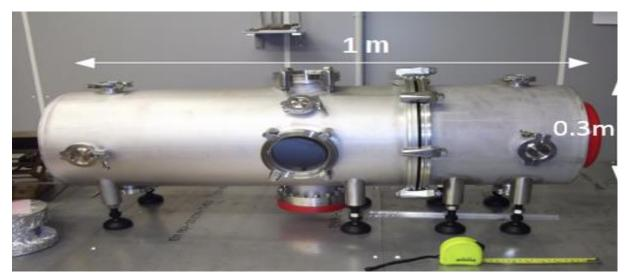
*Figure 1.14. A photograph of Aline vacuum chamber without magnetic field coils, cite from [Faudot 2015]*
