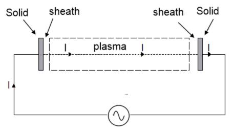
Figure 2.15. A draw of a current-driven symmetric double sheath
