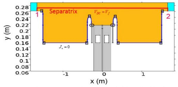
Figure 4.5. Simulation geometry in V<sub>RF</sub> and V<sub>DC</sub> modules. V<sub>RF</sub> solved along 1D sheath boundaries, whereas V<sub>DC</sub> solved in the 2D SOL domain. The orange color indicates the plasma region; Grey is the vacuum region. Rectangle and ellipse are the boundary points where the RF sheath boundary condition applied in the two approaches; The two identities are the DC sheath boundary condition imposed at the corresponding lines
