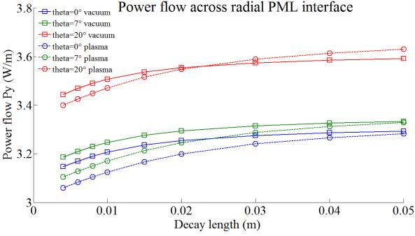
Figure 3.22. Radial power flow w.r.t decay length, case 1
