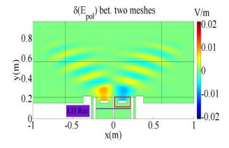
Figure 3.11. Differential field for the real part of poloidal electric field, i.e. Epol(mesh 1)-Epol(mesh 2). Horizontal line: location of LH resonance. Rectangle: box region shown in Figure 3.12
