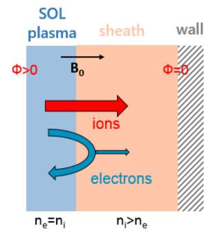
Figure 2.12. A diagram of DC sheath formation
