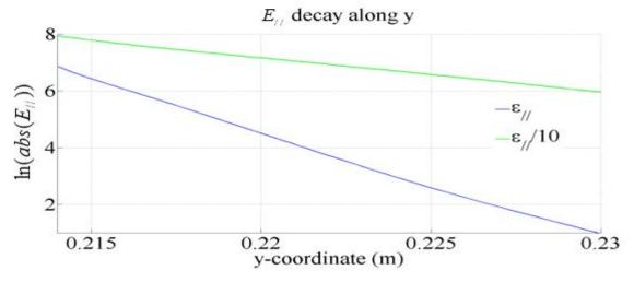
Figure 5.3.  $E_{//}$  calculated along a vertical line(x=-0.1m) in the slow wave code
