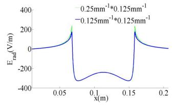
Figure 3.15. Toroidal distribution of Re(E<sub>rad</sub>) on the front face of the right strap, under two very dense symmetric meshes, other conditions are the same with Figure 3.14
