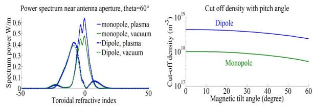
Figure 3.18. Power spectrum at large tilt angle theta=60°, plasma density 3 is used for blue curves
