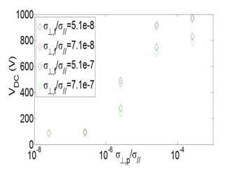
Figure 5.11. Dependence of the V<sub>DC</sub> at the leading edge of the left side limiter on perpendicular conductivities
