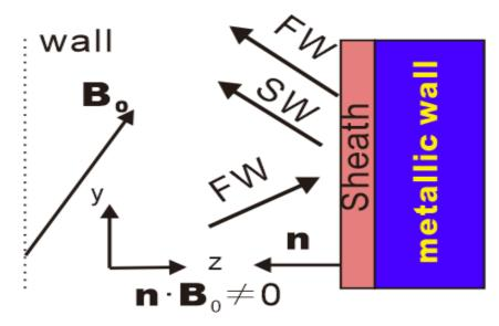
Figure 2.19. Mode conversion mechanism under tilted magnetic configuration
