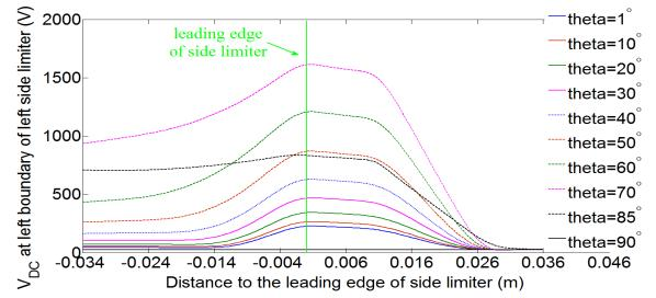
Figure 5.9. V<sub>DC</sub> at the green line of the left figure of Figure 5.15, w.r.t the magnetic tilt angle. Excitation is done by imposing 1000A current on each strap
