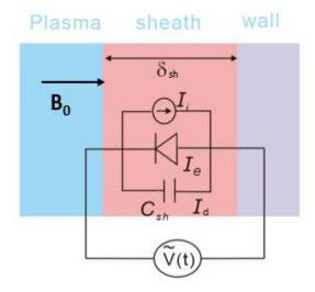
Figure 2.14. Equivalent circuit of RF sheath
