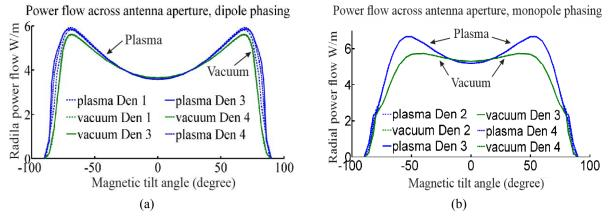
*Figures 3.17*. Radial power flow across the antenna mouth versus the magnetic field tilt angle, (a) dipole phasing with density profiles 1, 3 and 4. (b) Monopole phasing with density profiles 2, 3 and 4. Blue curves indicating plasma-filled antenna box. Green curves show simulations with vacuum in the antenna box.
