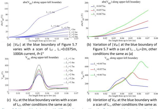
Figure 5.8.  $V_{RF}$  and  $V_{DC}$  behavior with different dimensional lengths; Data were picked up along the blue boundary of Figure 5.7. A constant density  $9 \times 10^{18} m^{-3}$  at SOL region,  $f_0 = w_0/2\pi = 48MHz$ ,  $B_0(y=0.214m)=2.3T$ ,  $\theta = 1^o$
