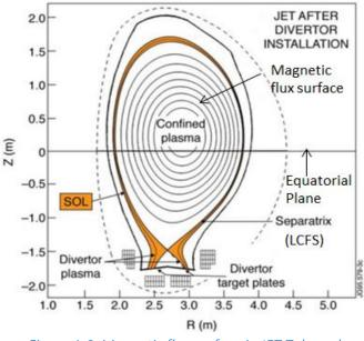
Figure 1.6. Magnetic flux surface in JET Tokamak
