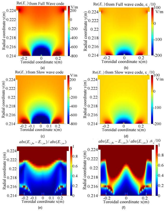
Figure 5.4. Comparison of  $E_{//}$ . Left: normal parameters Right:  $\mathcal{E}_{x}/10$
