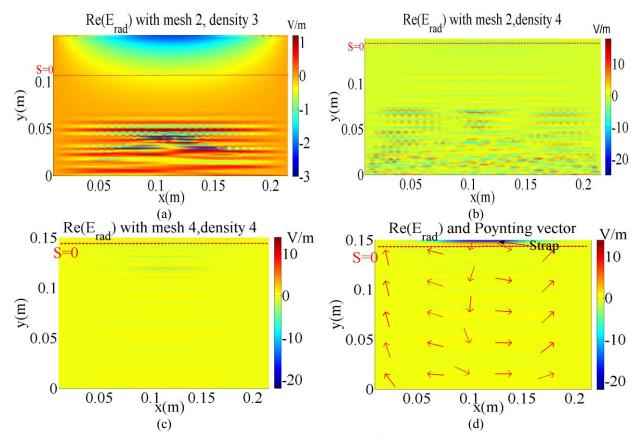
**Figures 3.16.** (a)-(b). Real part of the radial electric field with different density profiles, but the same mesh. Dipole phasing, theta=0°. (c). the same simulation as (b) but with mesh 4. (d) Radial electric field, using density 4, the same mesh size as mesh 4 but with square grid, instead of triangle. Red arrows indicate the normalized real part of the Poynting vector
