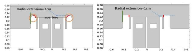
Figure 5.15. Two realistic geometry used in the simulation of this section. Left: the curved part (enclosed by the orange circle) at the top of side limiters is kept but being shifted downwards; The green vertical line is where the V<sub>DC</sub> data is extracted in Figure 5.17; The two red curves are where the heat flux is examined in Figure 5.20. Right: the curvature part at the top of the side limiters is removed
