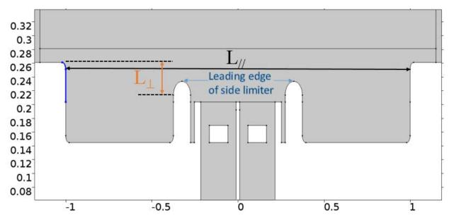
Figure 5.7. The characteristic length  $L_{//}$  and  $L_{\perp}$  are shown in the geometry; Blue boundary is where  $V_{RF}$  and  $V_{DC}$  are examined in Figure 5.8
