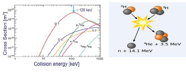
Figure 1.1. Nuclear fusion cross sections of different fusion reactions
