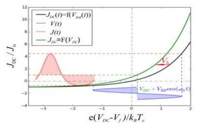
Figure 2.16. An illustration of DC sheath rectification
