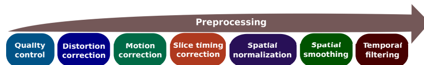
Figure 1.2: Preprocessing of fMRI data: Illustration of the complex pipeline necessary to extract useful information from the fMRI BOLD signal.
