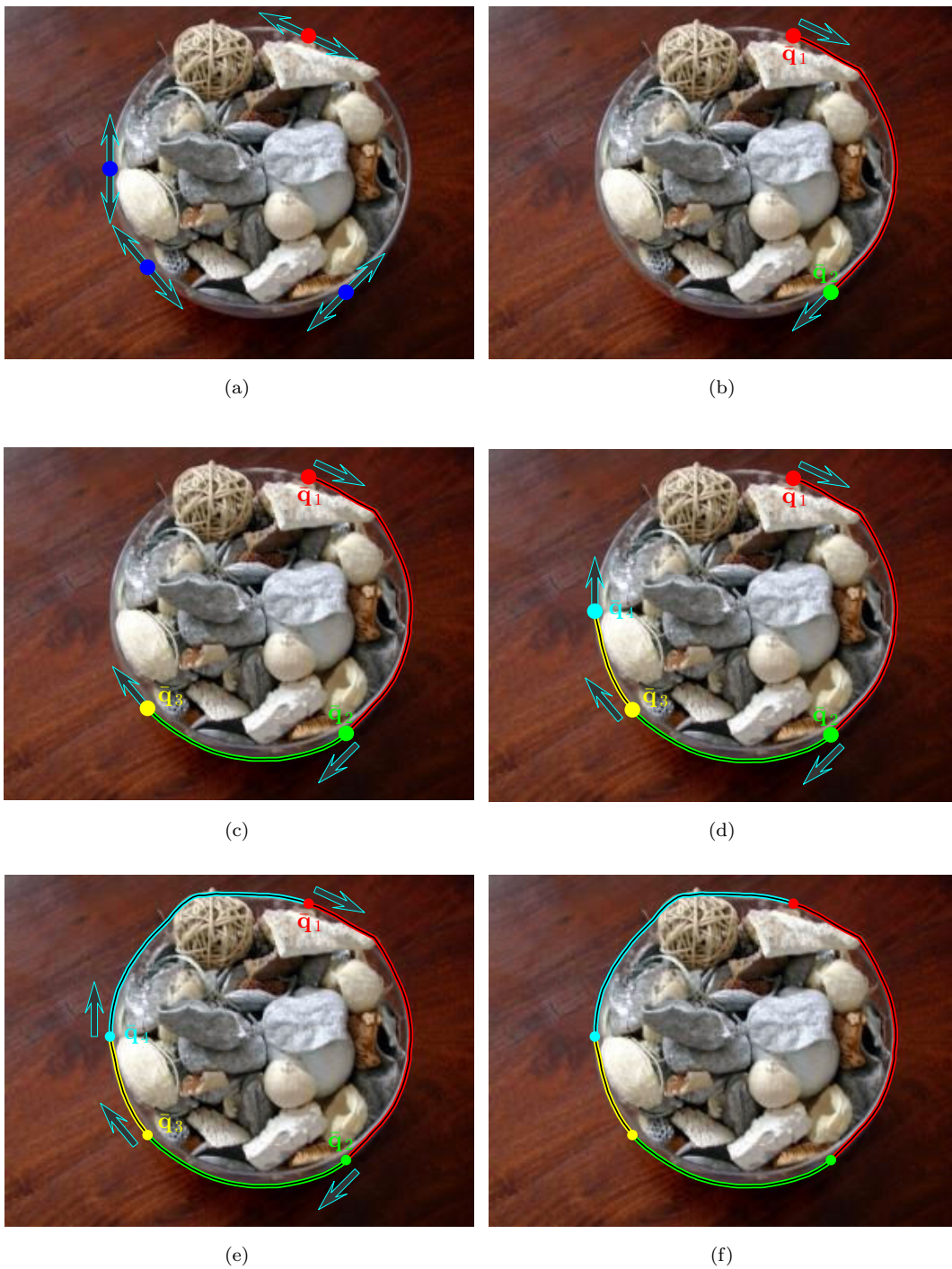
FIGURE 5.4: Steps for the closed contour detection procedure. (a) original image and all vertices in \mathcal{D} denoted by dots and arrows. (b) The first pairs of successive vertices ( \bar{q}_1, \bar{q}_2 ) is detected. (c) The third vertex \bar{q}_3 is detected. (d) The final vertex \bar{q}_4 is detected and the closed contour detection procedure is stopped. (e) Geodesic joining \bar{q}_4 and \bar{q}_1 is tracked. (f) The final closed contour is obtained.
