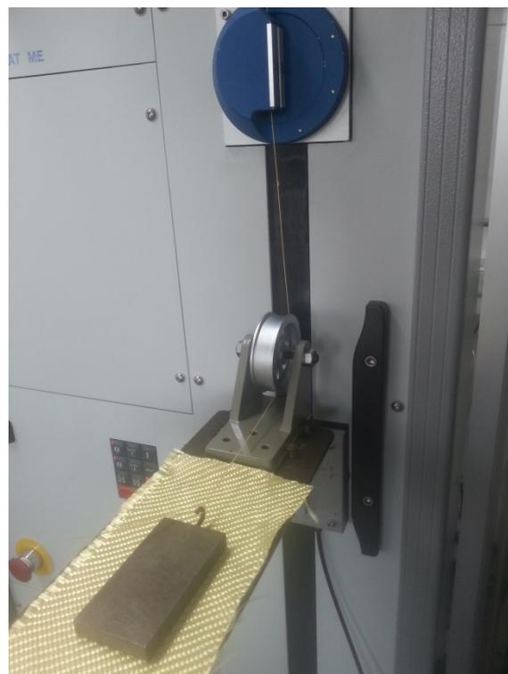
**Figure 2-29: Friction measurement device**
