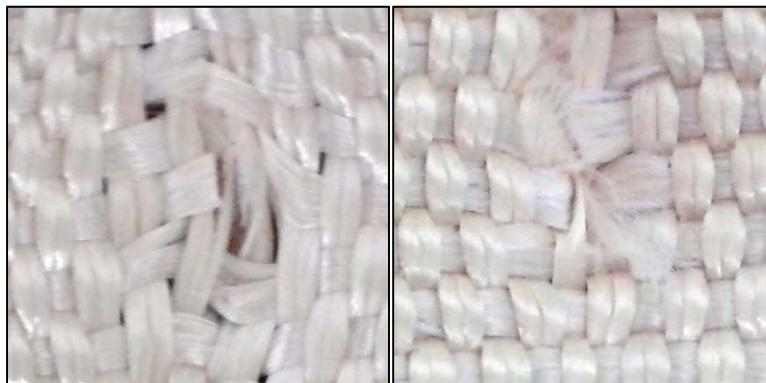
Figure 3-24: Aramid and Aramid/wool blend
