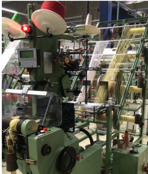
Figure 3-22: Narrow weaving machine NFREQ
