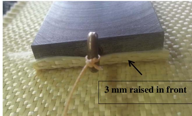
**Figure 2-28: Fixed fabric on the sled**
