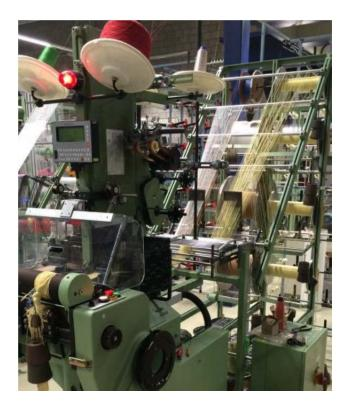
Figure 3-22: Narrow weaving machine NFREQ
