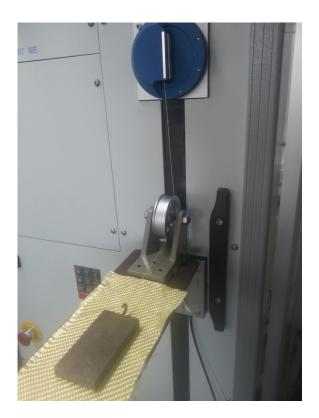
Figure 2-29: Friction measurement device
