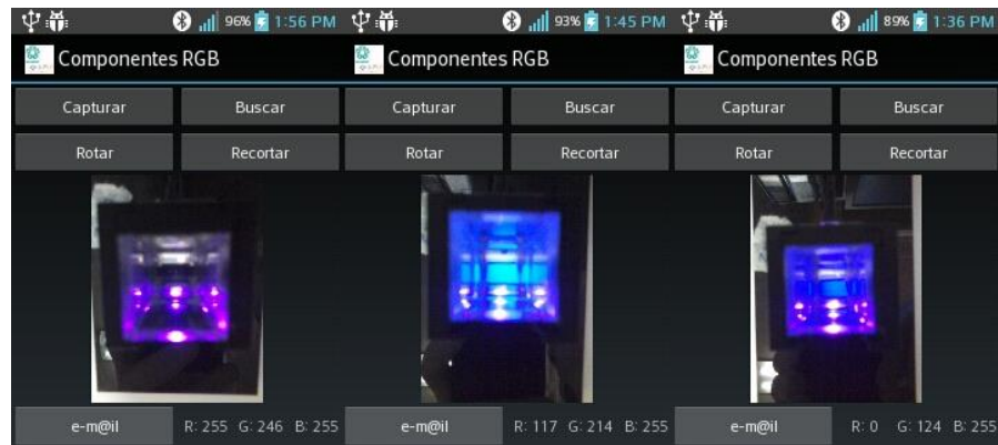
Fig. 87 Employing APP to capture an image and get its RGB components.
