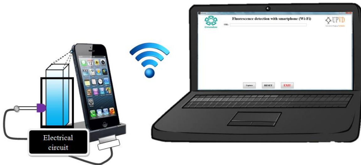
Fig. 30 Fluorescence analyzer developed based on smartphone camera
