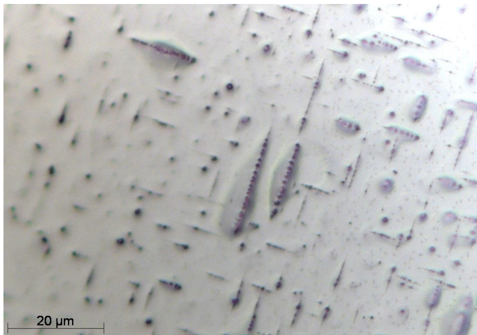
FIGURE 5.12: Precipitates formed at the surface of Al(100) after an excessive coverage of iridium (undetermined).
