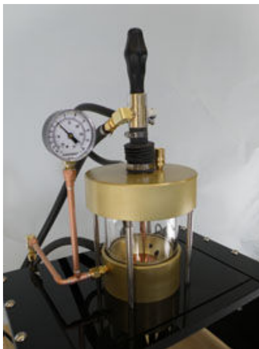
FIGURE 2.1: Picture of the chamber of a SA-200 laboratory arc-melter from the Materials Research Furnaces, Inc.
