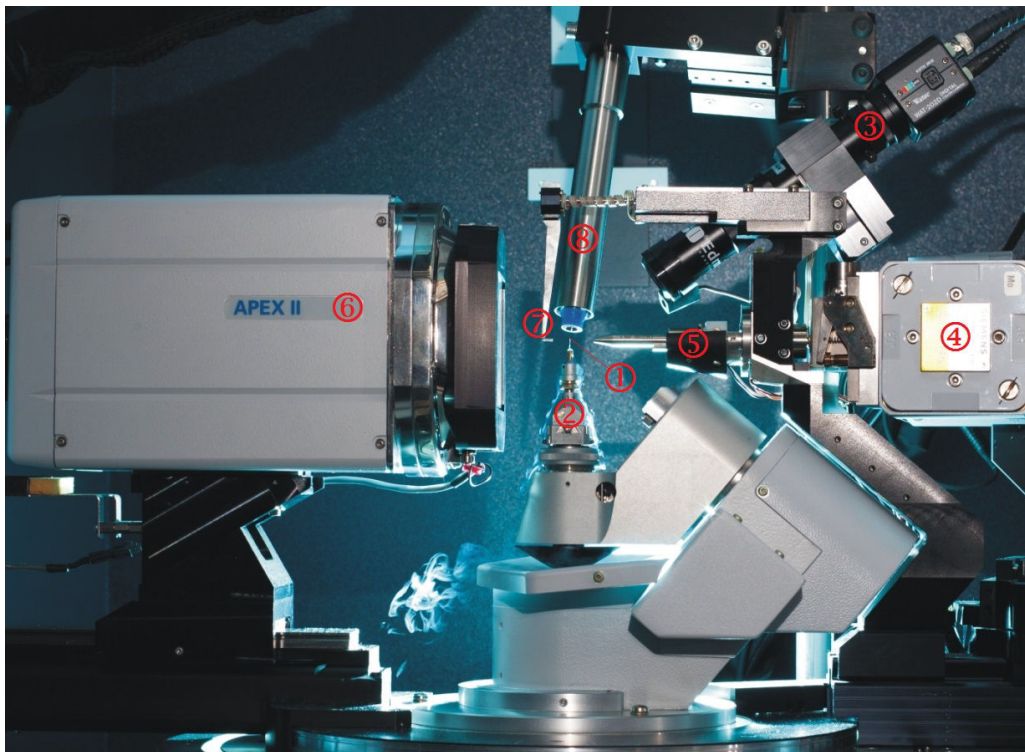
FIGURE 2.4: A four-circle single crystal X-ray diffractometer [34], see text for the description of the elements.
