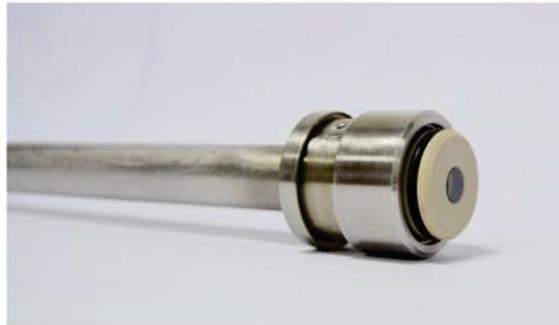
Figure 95: Main component of the beta sensor (top) and the complete design of the beta sensor with its mechanical part (bottom)
