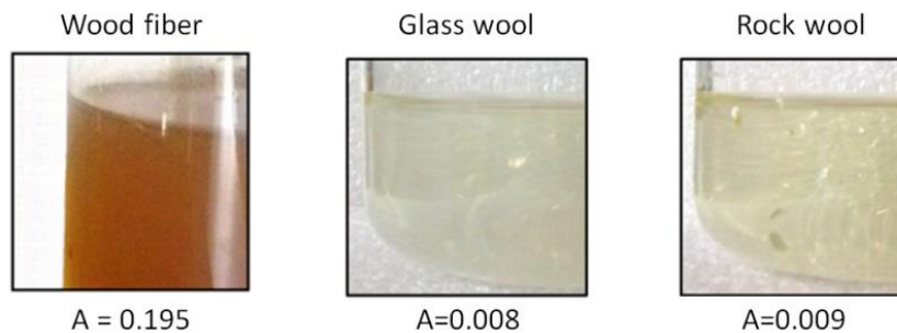
Figure 5.5 – Water coloring and absorbance measurements after immersing insulation materials
