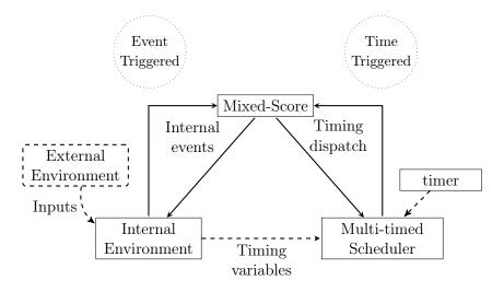
Figure 5.4: Architecture of the Antescofo reactive engine
