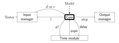
Figure 3.11: VM architecture scheme: given a IRTM as input, the VM simulates the model following the standard semantics.
