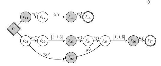
Figure 3.8: IRTM example: This model comes from the TAIO example depicted in Figure 2.9, replacing the input (resp. output) actions by emissions (resp. receptions) of symbols and signals.
