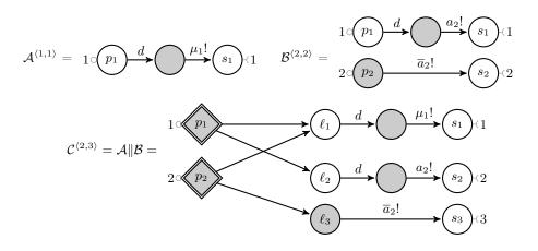
Figure 4.10: Parallel composition of two FSMs.
