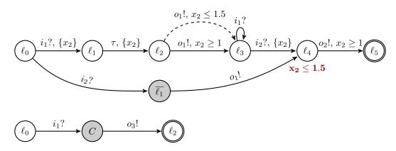
Figure 2.9: An example of a network of three TAIOs. The three models are composed in parallel and communicate with input/output actions.
