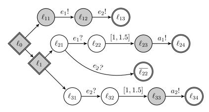
Figure 3.2: IRTM principle: A IRTM is a set of Finite State Machines (FSM) activated dynamically and has one initial location ( $\ell_0$ ). The model is mostly deterministic and specifies explicitly time progression through a simulation.
