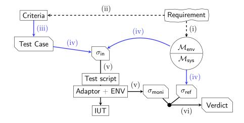
Figure 2.11: The Model-Based Testing Workflow
