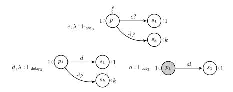
Figure 4.22: FSMs constructed by  $\vdash_{seq_3}$  and the new  $\vdash_{seq_0}$ .
