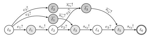
Figure 5.21: Proxy Uppaal TA transformed to prevent from (deadlock).
