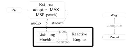
Figure 5.24: Testing the whole Antescofo system.
