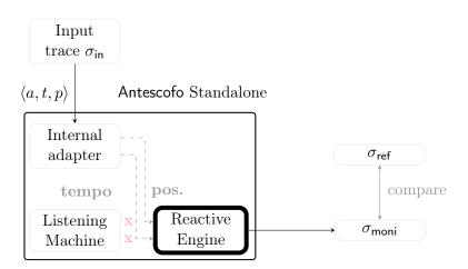
Figure 5.22: Testing the reactive engine.
