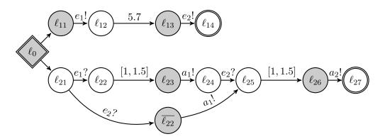
Figure 3.6: IRTM example: This model comes from the TAIO example depicted in Figure 2.8, replacing the input (resp. output) actions by emissions (resp. receptions) of symbols and signals.
