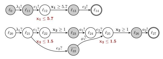
Figure 3.9: TIOLTS network example: Translated from the IRTM example depicted in Figure 2.9. Gray locations are urgent and when omitted, the guard is true ( $\top$ ) and the action is the internal action  $\tau$ . The constructed TAIOs are *real-time* TAIOs and reset their local clock  $x_i$  in every transition. Therefore, for all transitions and for  $i \in \{1, 2\}, \mathcal{U} = \{x_i\}$ .
