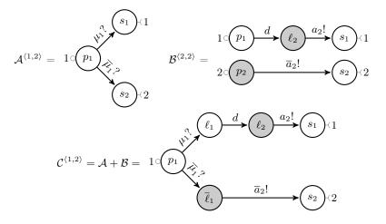
Figure 4.11: Sequential composition of two FSMs.
