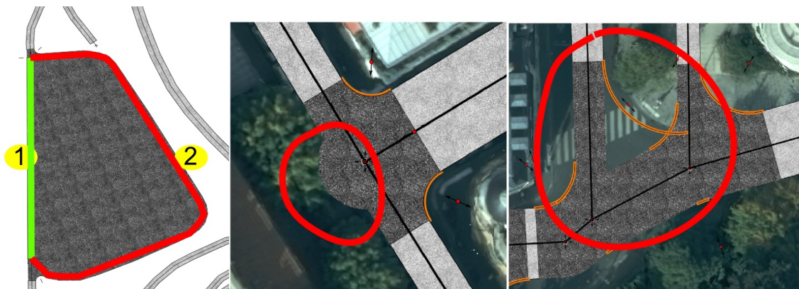
Figure 79: Various cases of failure from more severe to less severe (1 , 2 , 3). 1 : loop, 2 : bad buffer use, 3 : radius too big for network.
