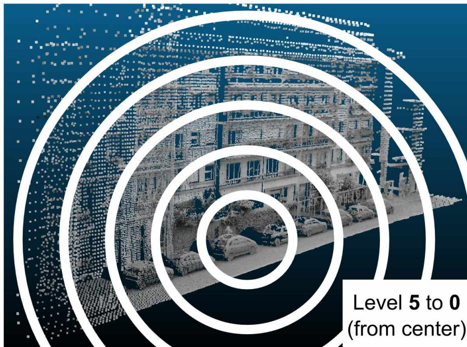
Figure 150: Schematic example of LOD depending on distance to camera
