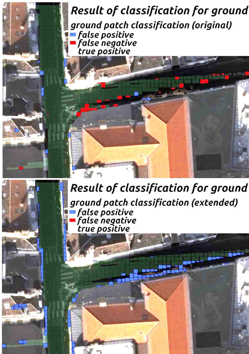
Figure 163: Map of patch clustering result for ground. The classical result finds few extra patches that are not ground (blue), and misses some ground patches (red). Recall is increased by adding to the ground class all patches that are less than 2 meters in X,Y and 0.5 meter in Z around the found patches. Extra patches are much more numerous, but all the ground patches are found.
