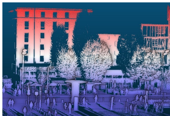
Figure 15: On this street Lidar point cloud, trees are clearly masking building facades, creating occlusion.
