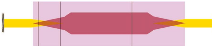
Figure I-19: Schematic view of a Fabry-Pérot cavity with cleaved facets in the silicon waveguide. Image from [62].
