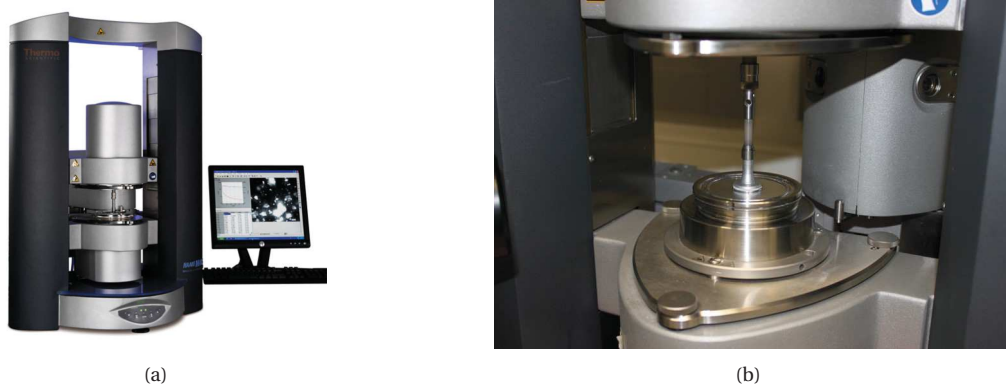
Figure 2.9 – Dynamic shear rheometer HAAKE TM MARS TM from ThermoFisher Scientific: (a) image of the complete device; (b) zoom on the area of interest during an experiment.
