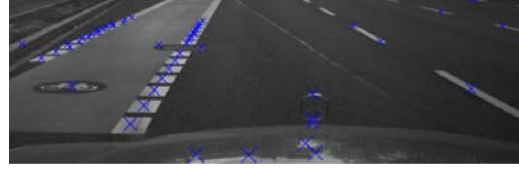
(b) This image depicts the centroids of the clusters which are used for point pattern matching with the iterative closest point algorithm.
