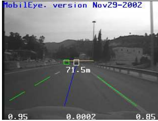
(a) Front view with lane and object detection for longitudinal control, lane keeping, collision mitigation, collision avoidance, etc. Image: [46].
