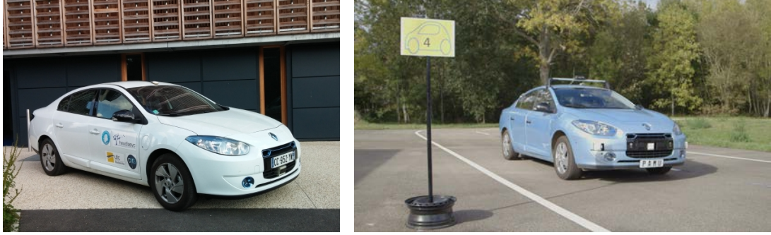
(a) Robotic car named IRIS of the Heudi- asyc laboratory (b) Autonomous valet parking vehicle from Renault PAMU (Urban Mobility Application Platform) project
