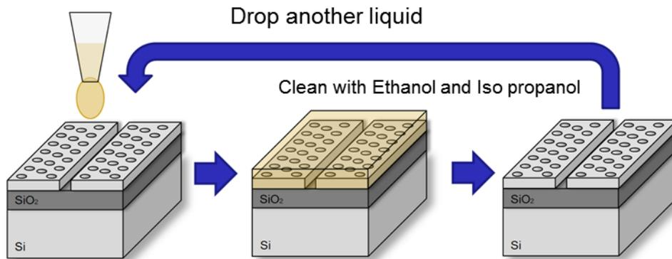
**Fig. 3.2.1** Schematic of the experimental method used to proceed to SOI sample top cladding cleaning and drop casting of optical index.
