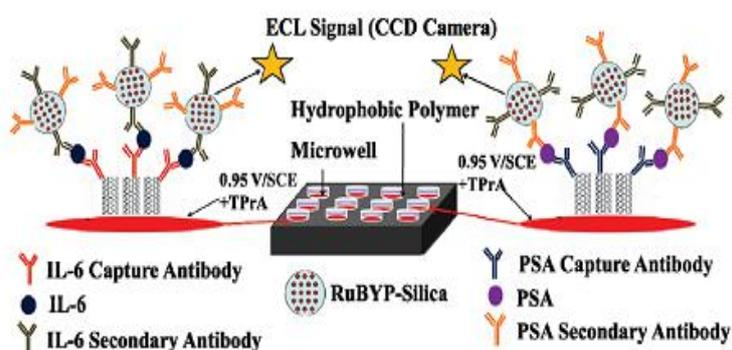
Figure 19. Schematic representation of ECL immunoarray based on the SWCNT forest
