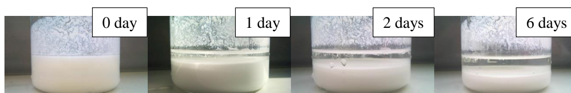
Fig 62 : Sedimentation evolution with aging duration for the “PANaF0.03 HAc 6d” sample.
