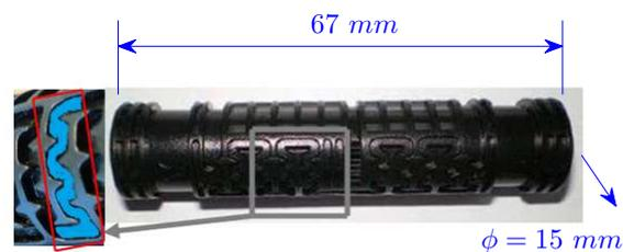
Figure II.1.3: Emitter studied (industrial geometry)
