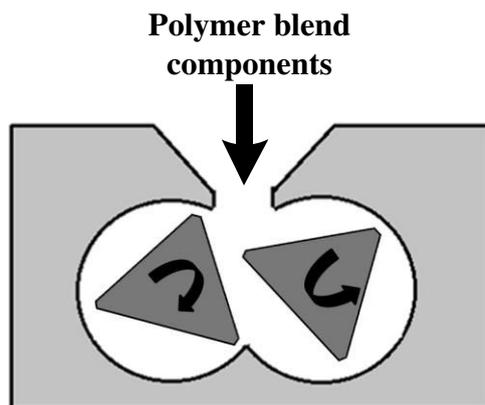
Figure 3.6 Scheme of a batch mixer.
