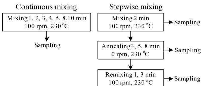
Figure 3.7 Mixing modes used for polymer blending.
