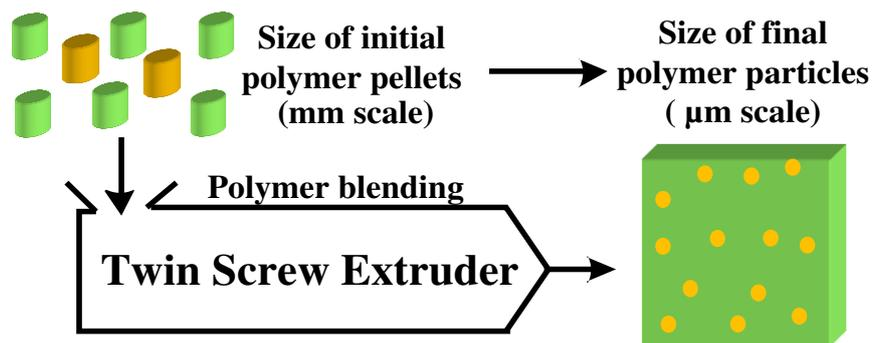
Figure 1.1 Scheme of a typical polymer blending process carried out in a continuous mixer of type twin screw extruder.
