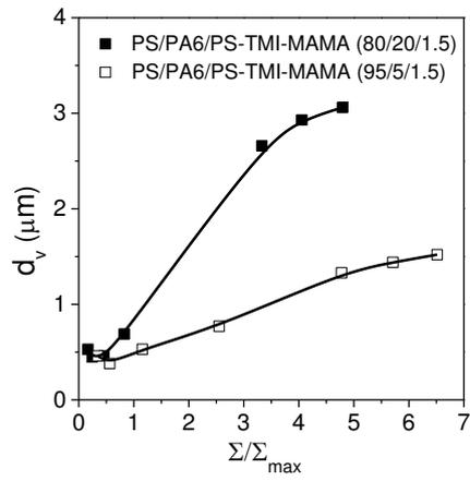
Figure 3.19 Diameter of the dispersed phase domains as a function of the relative interfacial coverage of the copolymer  $\Sigma/\Sigma_{max}$  for PS/PA6/PS-TMI-MAMA1 reactive blends.
