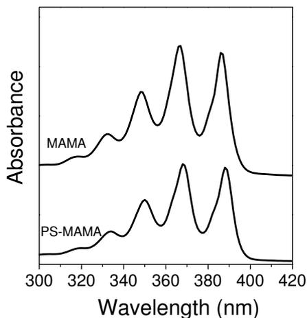
Figure 3.9 Ultraviolet absorption spectrum of MAMA and PS-MAMA1.
