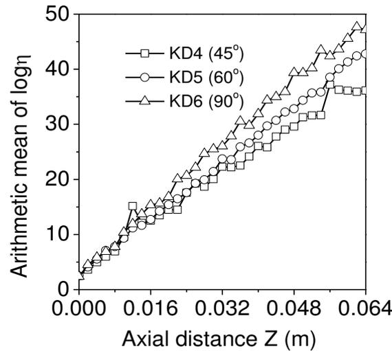
Figure 8.5 Axial evolution of mean log of the area stretch  $\eta$ ; Screw speed: 150 rpm, feed rate: 17.8 kg/h. <sup>[167]</sup>
