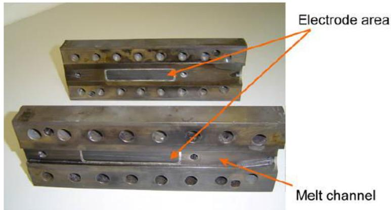
Figure 2.8 Configuration of the die of the extruder.
