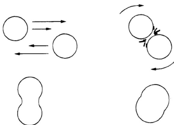
Figure 2.3 Scheme of coalescence of the dispersed phase.
