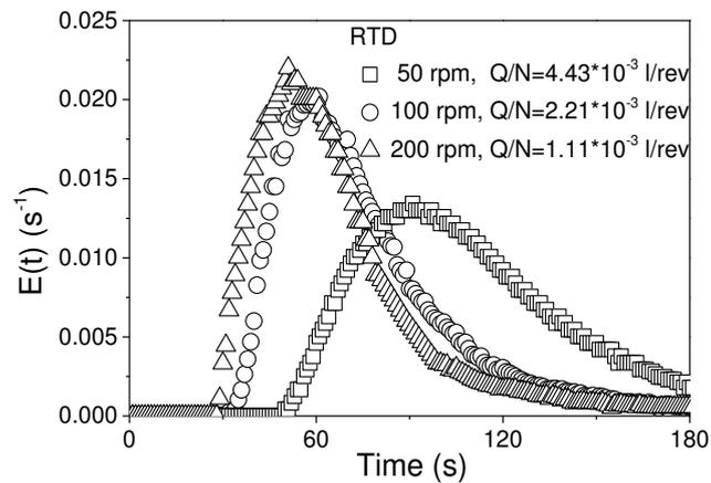
Figure 7.2 Effect of the screw speed on the RTD curves.
