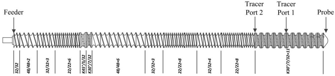
Figure 5.3 Screw configuration of the twin-screw extruder.
