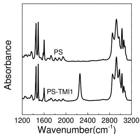
Figure 3.8 FTIR spectrums of PS and PS-TMI1.
