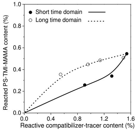
Figure 5.7 RCC-CC: reacted reactive compatibilizer-tracer content as a function of the reactive compatibilizer-tracer content in the PS/PA6 (80/20) blend (data from Figure 5.5).
