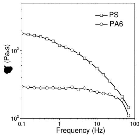
Figure 4.3 Complex viscosity vs frequency of PS and PA6 at 230°C.
