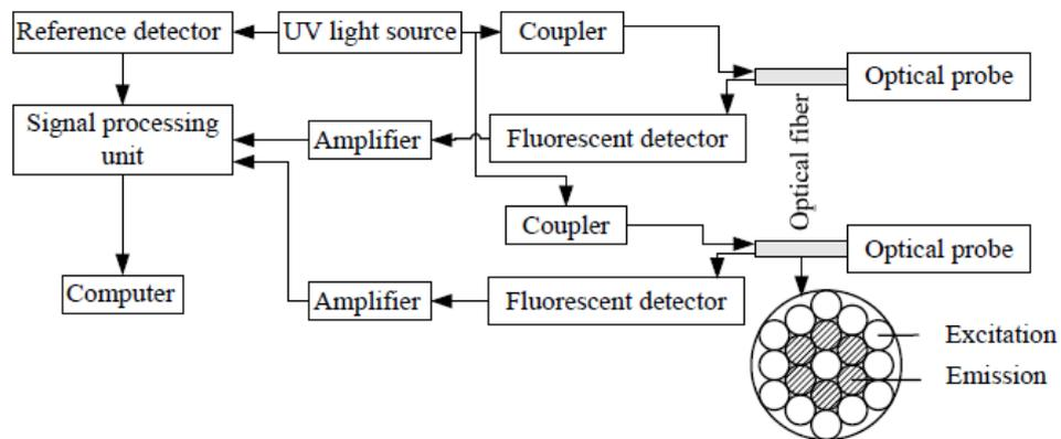
Figure 5.1 Diagram of the in-line fluorescent measuring system.
