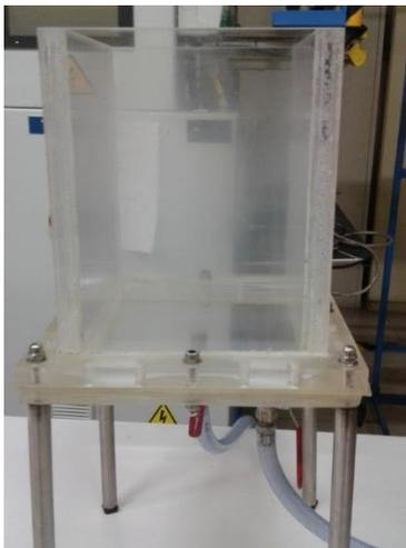
Figure 6.4 - Physical model used to perform the mass transfer experiments
