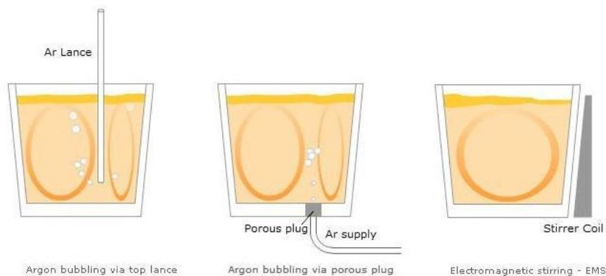
Figure 1.5 - Ladle treatments commonly used in secondary steelmaking processes [4].
