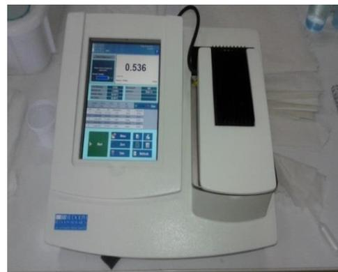
Figure 6.5 - Light Refractometer used to measure thymol concentration from samples in trials.
