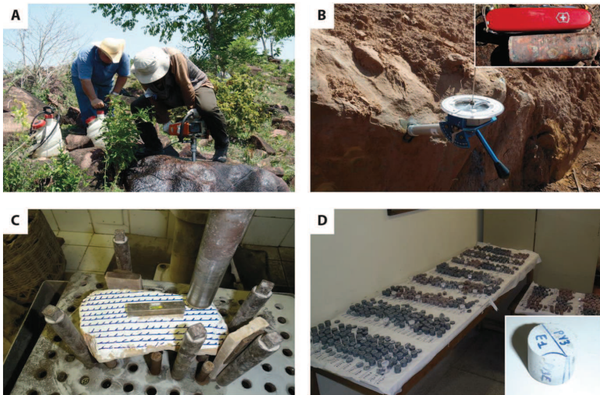
Figure 4.2: A: Sampling with a portable gasoline – powered drilling apparatus to drill a felsic dike (Tucumã). B: Sample orientation. C: Drilling of an oriented block in laboratory. D: Specimens in laboratory after preparation of cylindrical samples.
