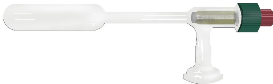
Figure 2.4. Pyrex ampule equipped with a valve used to analyze hydrated samples irradiated using electron beams and that used for annealing. Longneck ampules were used in order to keep the rubber seal attached to the valve clean and maintain the vessel leak proof.
