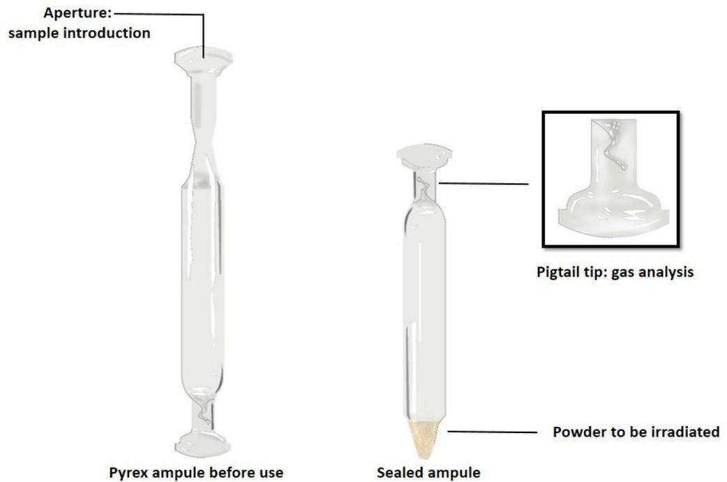
**Figure 2.5. Pyrex ampules equipped with a pigtail used to analyze dry electron beam irradiated samples and all Gamma irradiated samples. The aperture from one side facilitates the introduction of the sample and gas (left). Ampules are then sealed, powder is irradiated and gas is analyzed by breaking the pigtail (right).**
