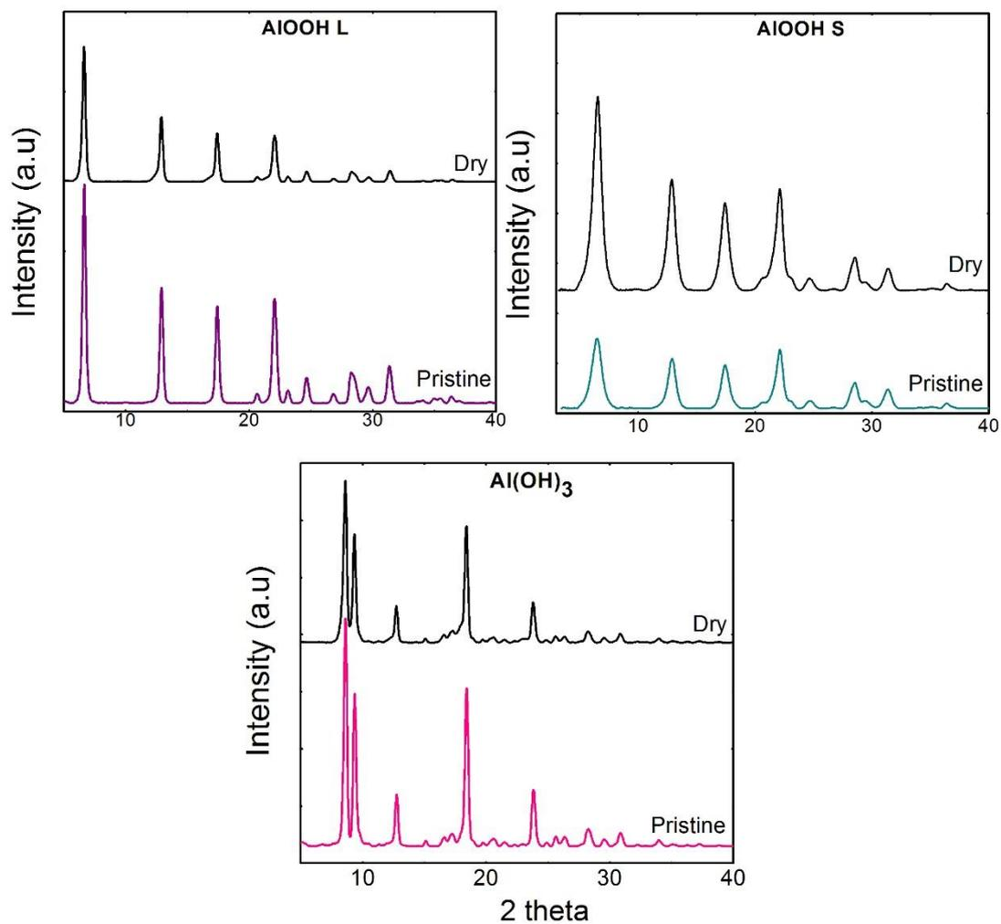
**Figure 3.2. DRX of AlOOH and Al(OH)<sub>3</sub> comparing pristine and dry samples.**
