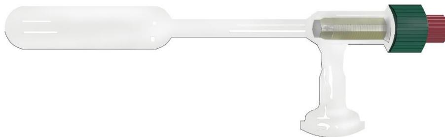
**Figure 2.4. Pyrex ampule equipped with a valve used to analyze hydrated samples irradiated using electron beams and that used for annealing. Longneck ampules were used in order to keep the rubber seal attached to the valve clean and maintain the vessel leak proof.**
