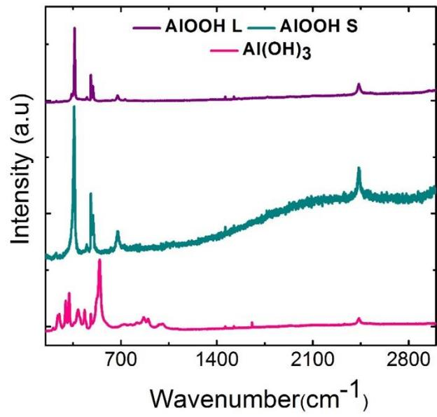
Figure 3.6. Raman spectra of Al(OH)<sub>3</sub> and AlOOH.
