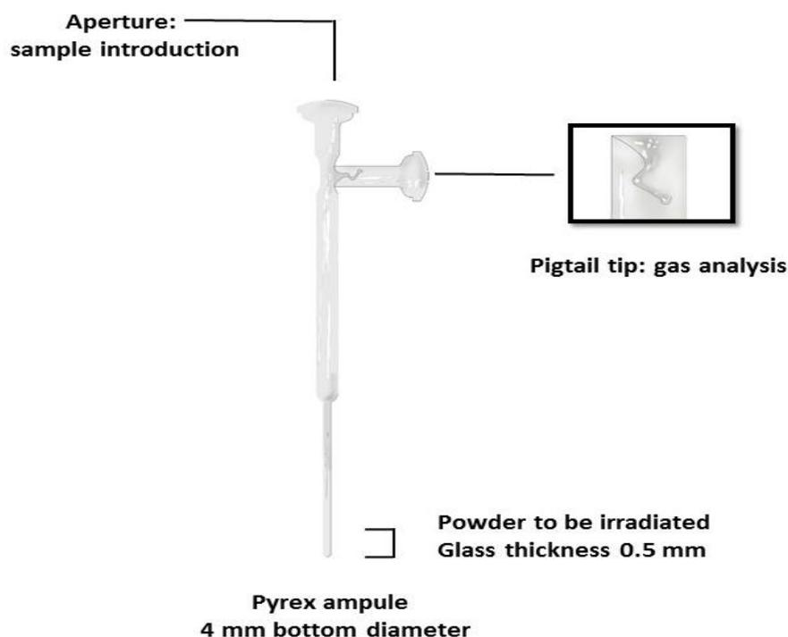
**Figure 2.6. Pyrex ampules equipped with a pigtail used to analyze samples irradiated using heavy ions. The aperture from one side facilitates the introduction of the sample and gas (left). The bottom is 4 mm diameter tube. Ampules are then sealed, powder is irradiated and gas is analyzed by breaking the pigtail (zoom on the right).**
