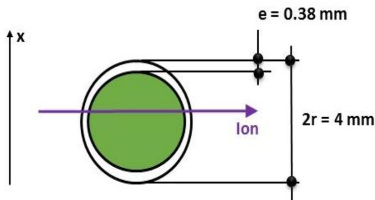
Figure 2.2. Used geometry to calculate the received dose. The diameter of the bottom of the ampule was 4 mm and 0.38 mm the glass thickness.
