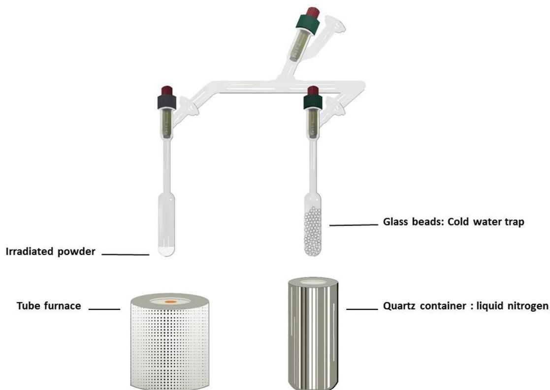
**Figure 2.9.** Annealing system consisting of the evacuated irradiated ampule (left) heated with a tube furnace until transition temperature is attained and connected to another ampule under vacuum (right). This latter is cooled using liquid nitrogen in order to trap water and adsorb it on the glass beads inside.
