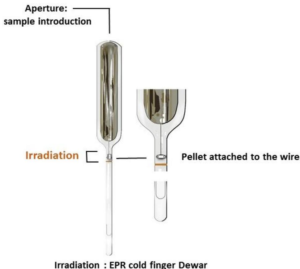
**Figure 2.7. EPR cold finger Dewar used to analyze irradiated pellets at low temperature. The sample is introduced attached to a metallic wire (left) and is then irradiated at the top of the thin quartz tube. After irradiation the pellet is released to the bottom of the Dewar in order to be analyzed by EPR.**
