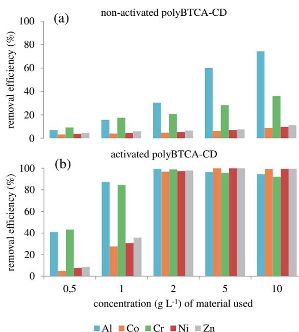
Figure 5: Adsorption capacity (%) of (a) the non-activated and (b) the activated (NaHCO<sub>3</sub> treatment) polyBTCA-CD at different doses for 5 metals (at 10 mg L<sup>-1</sup>).
