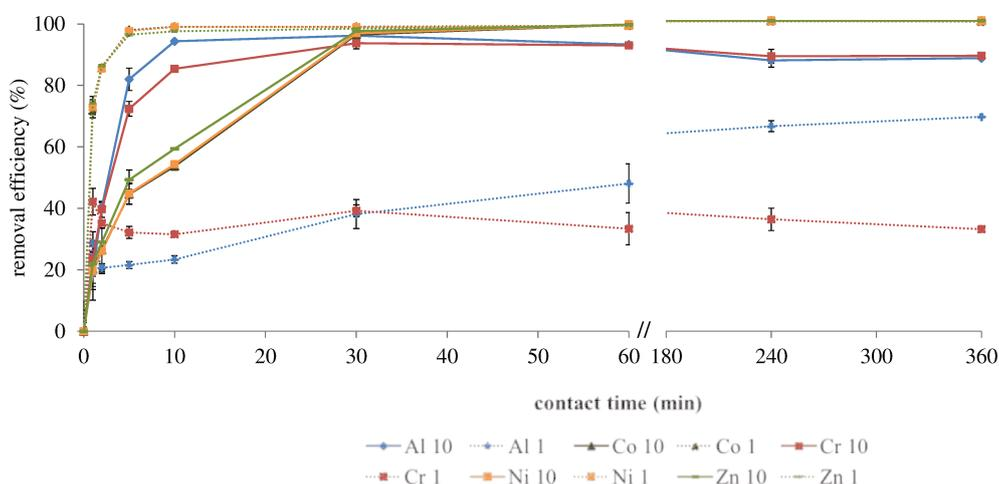
Figure 6: Adsorption kinetics for two solutions containing 5 metals at two concentrations (solution at 10 mg L<sup>-1</sup>: full lines; solution at 1 mg L<sup>-1</sup>: dashed lines) expressed as removal efficiency in % (n = 3).
