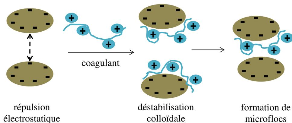
Figure 17. Principe de la coagulation.
