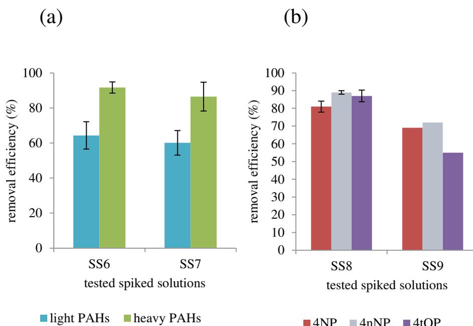
*Figure 7: Removal efficiency (%) after treatment by activated polyBTCA-CD (dose = 2 g L<sup>-1</sup>) for (a) two concentrations of PAHs: low for SS6 and high for SS7 (n=3) and (b) two concentrations of APs: low for SS8 (n = 3) and high for SS9 (n = 1).*
