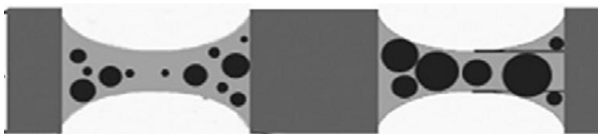
Figure II-17. Particles Size Segregation according to Carbon Film Thickness (Klang et al., 2012).
