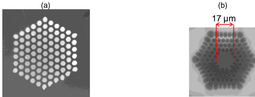
Figure III-17: (a) Micrograph of the holey cane used to manufacture the adiabatic converter. (b) Micrograph of the output end facet of the manufactured converter.
