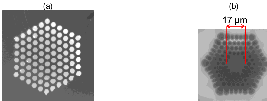
Figure III-17: (a) Micrograph of the holey cane used to manufacture the adiabatic converter. (b) Micrograph of the output end facet of the manufactured converter.
