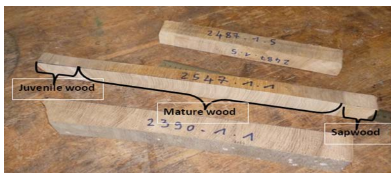
Figure 1. Photography showing European oak trees radii for sawdust sampling (only tree 2390 and 2547 were studied)
