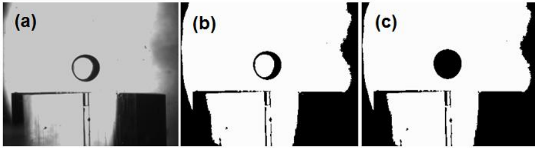
Figure 2.17: Steps for image analysis, with images from the first setup: (a) original image; (b) binary image; (c) border filling and analysis.
