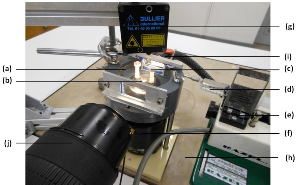
Figure 2.1: Photograph of the single drop formation setup: (a) continuous phase; (b) capillary tube; (c) screw; (d) syringe; (e) syringe pump; (f) vibrating exciter; (g) laser sensor; (h) anti-vibration table (i) light source; (j) macro lens mounted on high speed camera.
