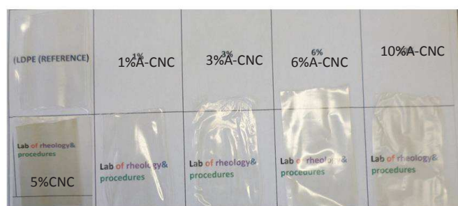
Fig. 11 Appearance of extruded CNC/LLDPE and A-CNC/LLDPE nanocomposite films.
