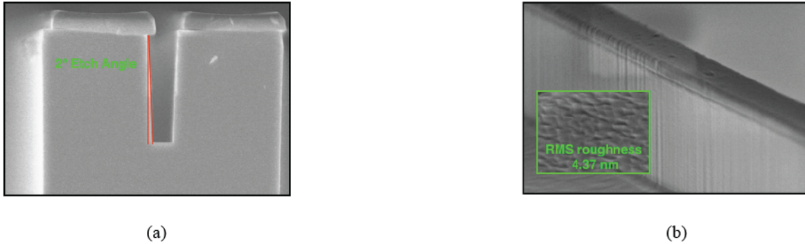
Fig. 3.9. SEM image of an InP test sample etched with the \text{Cl}_2\text{-H}_2\text{-O}_2 plasma (a) Directional coupler gap of 300 nm with an etch angle of 2° (c) Surface roughness induced by the etching amounting to an RMS value of 4.7 nm
