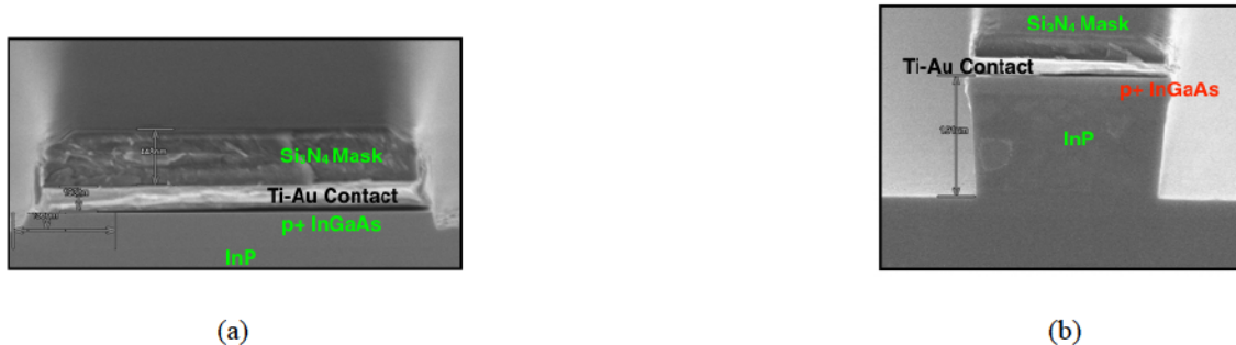
Fig. 3.15. SEM image of the sample (a) After IBE (b) After wet etching in 37% HCl
