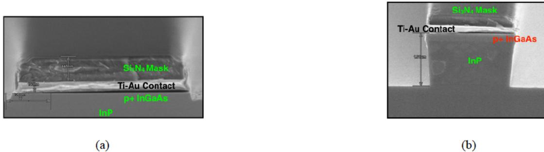
Fig. 3.15. SEM image of the sample (a) After IBE (b) After wet etching in 37% HCl
