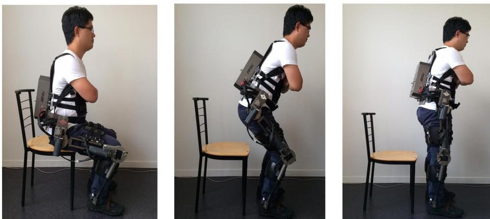
Figure 4.17 – The STS transfer task for experimental evaluation with the assistance of the E-ROWA exoskeleton.
