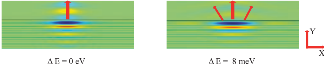
Figure 2.23: Simulated wave front for Tamm mode at \Delta E = 0 and \Delta E = 8 \text{ meV} . The cell dimensions are 2\mu\text{m} for Y and 10.2\mu\text{m} for X.
