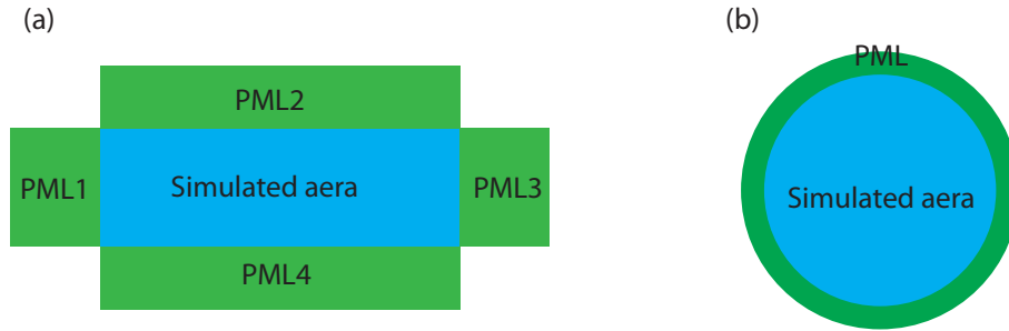
Figure 2.18: Schematic representation of different configuration of PMLs
