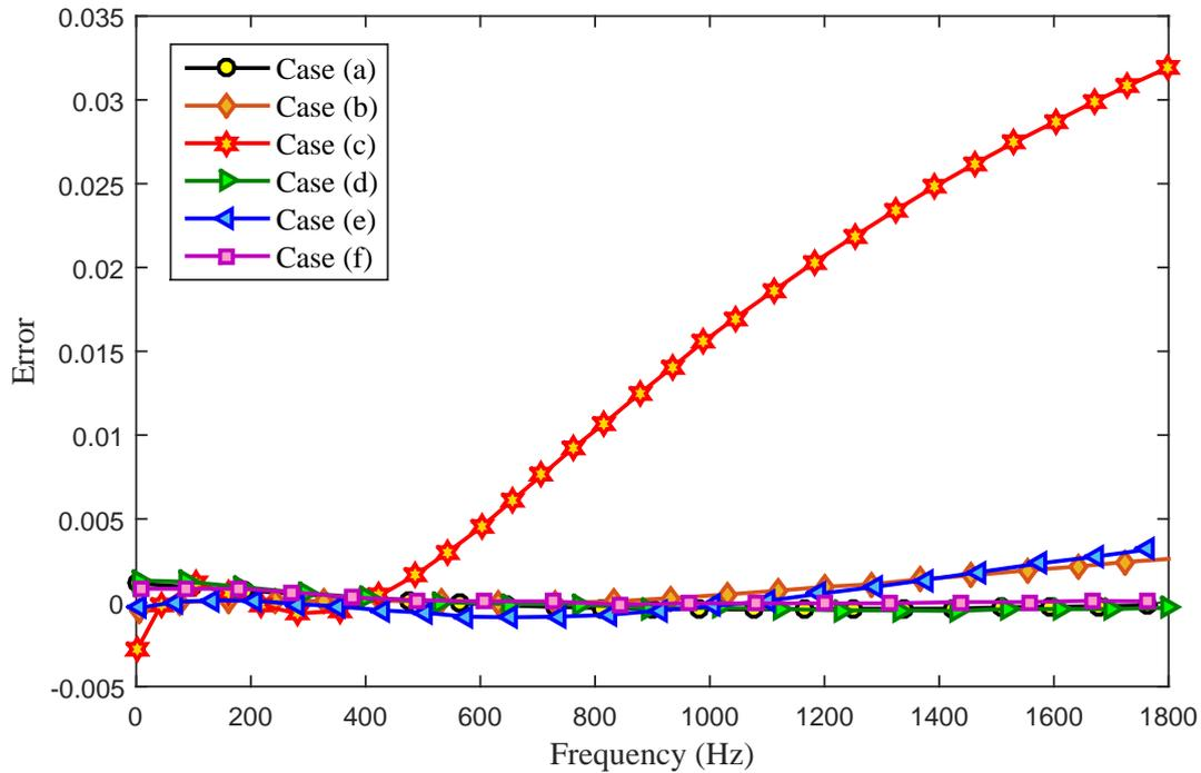
Figure 4.6: Difference between WFEM solutions and approximated wavenumbers.
