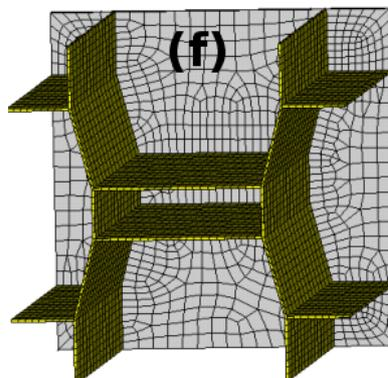
Figure 4.3: 3D Finite element model of the octagonal construction.
