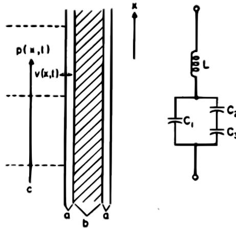
Figure 1.5: Equivalent electric circuit of the total impedance [77].
