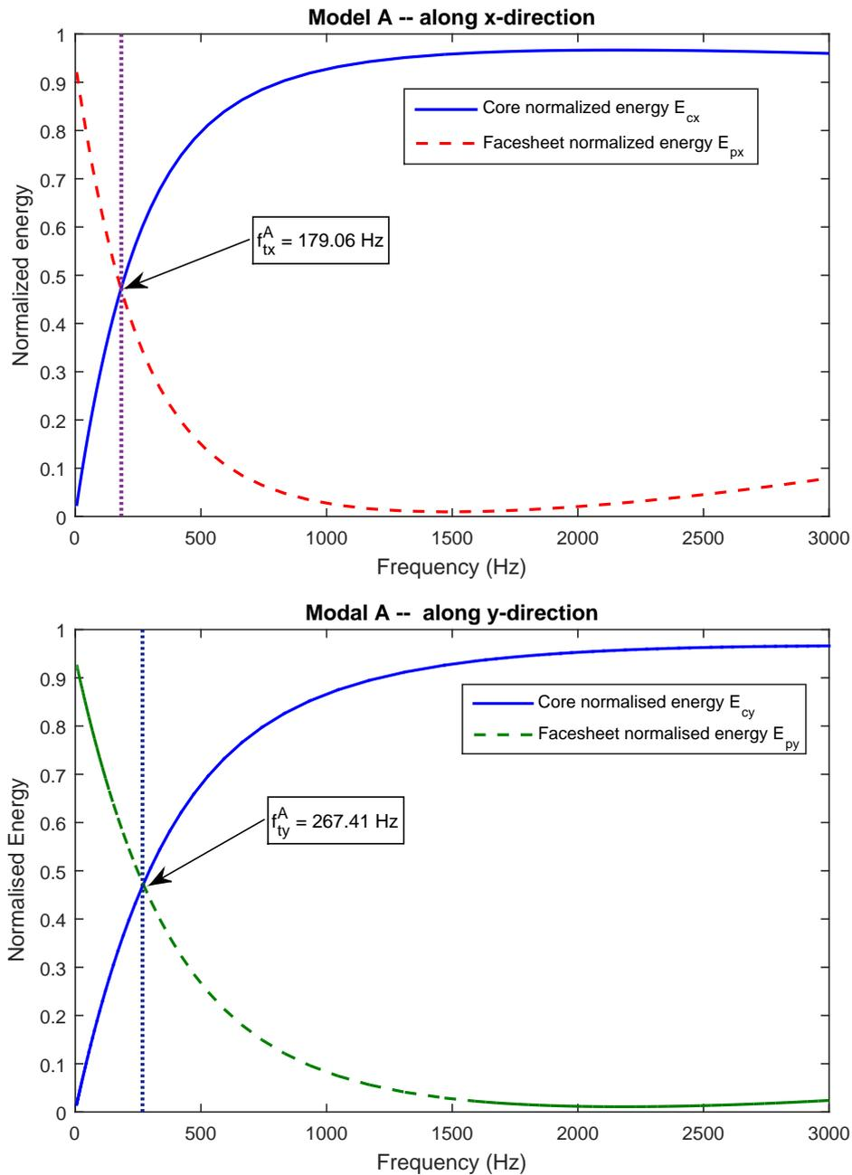
Figure 3.9: Strain energies of the honeycomb sandwich models A.
