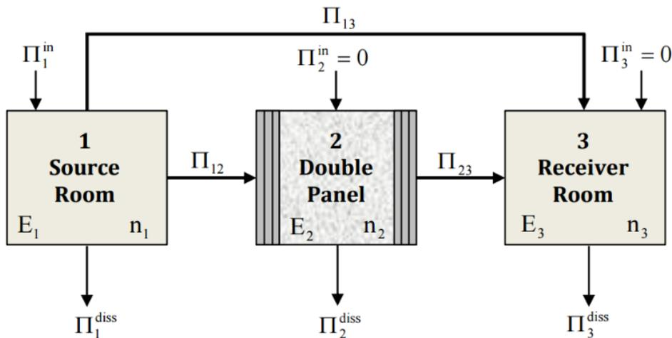
Figure 1.12: Power flow between the three sub-systems of a double composite panel quoted from [133].
