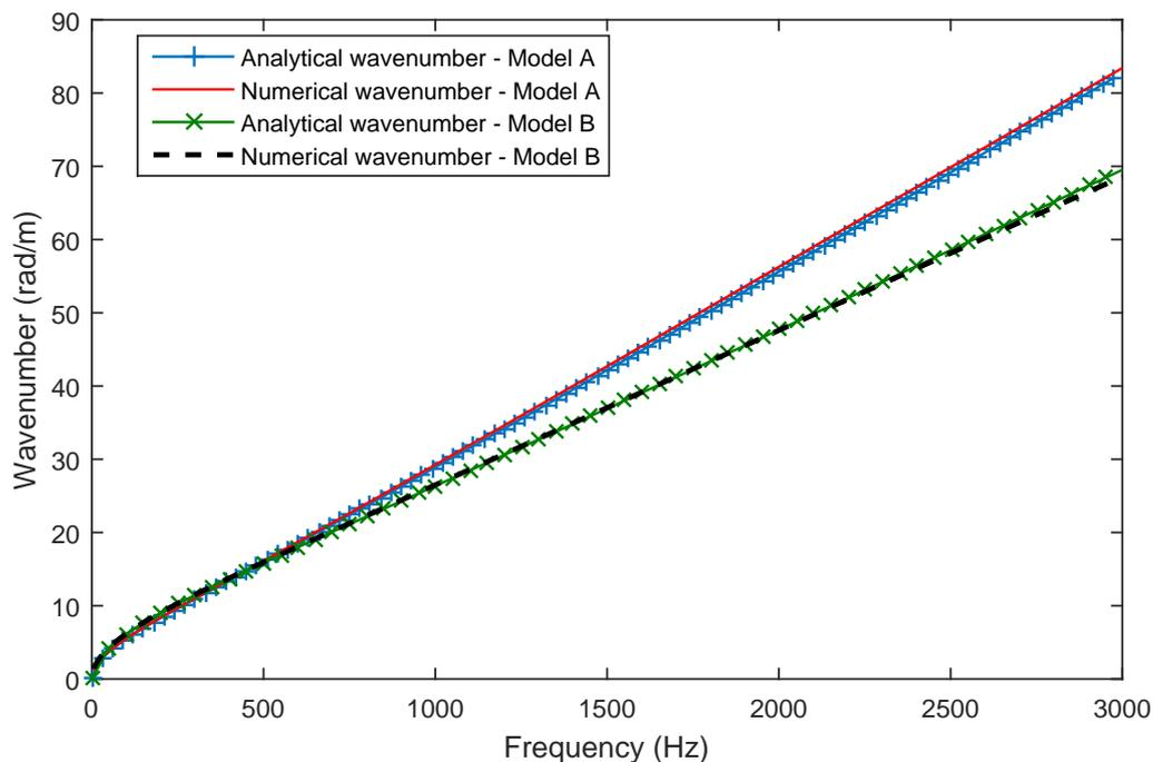
Figure 3.4: Comparison of the numerical and analytical wavenumbers.
