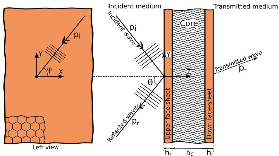
Figure 5.1: Transmitted and reflected plane wave at an infinite sandwich panel
