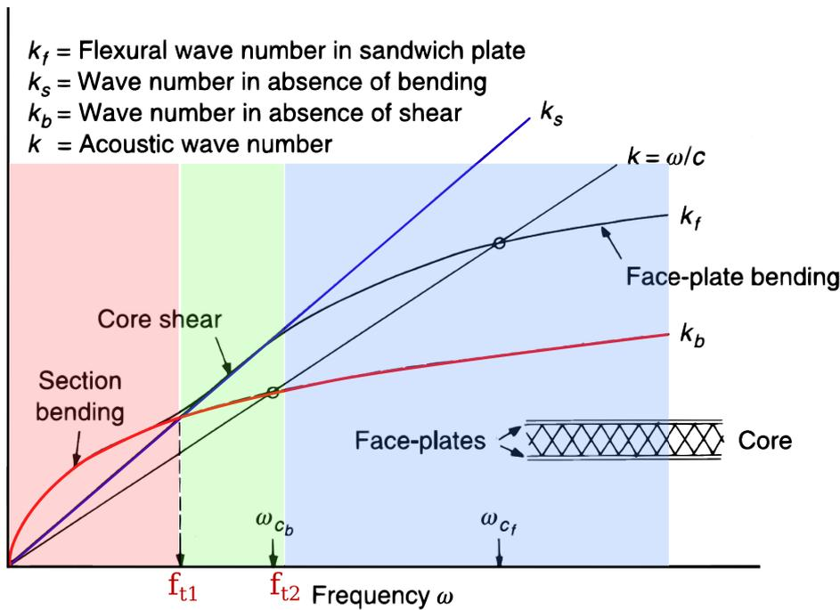
Figure 1.9: Typical dispersion curves for a sandwich panel [50].
