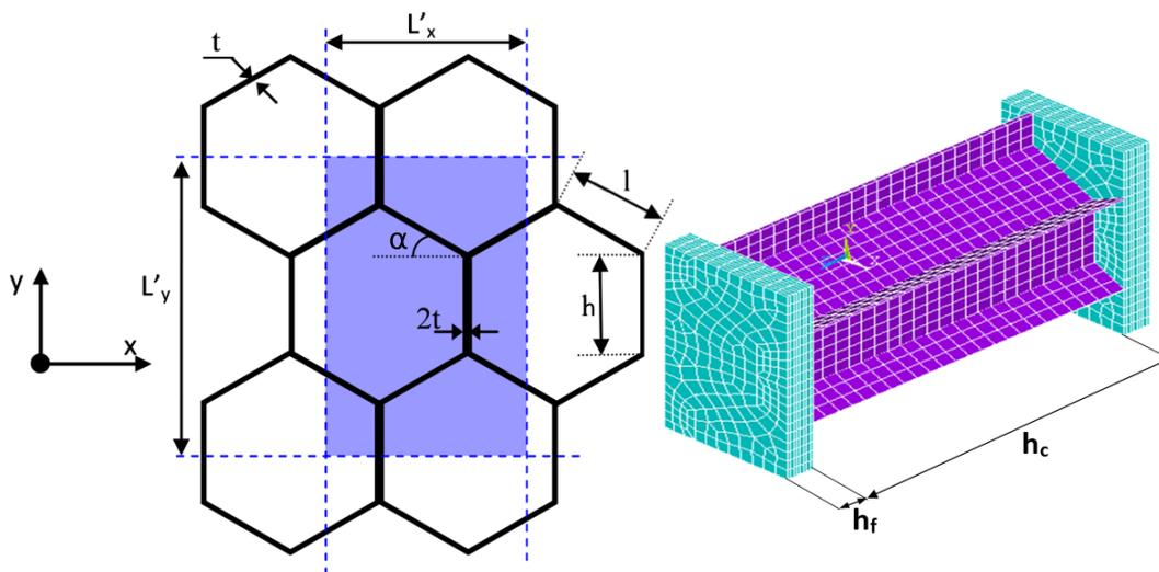
Figure 3.3: Geometric parameters of the unit honeycomb cell.
