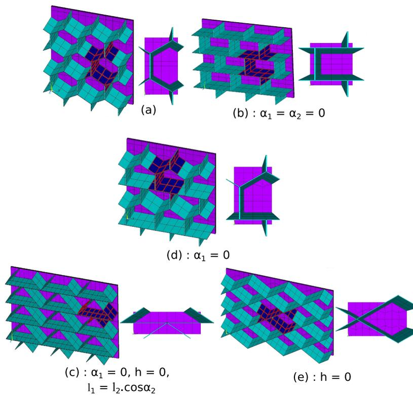
Figure 5.13: Studied core forms of the sandwich panels
