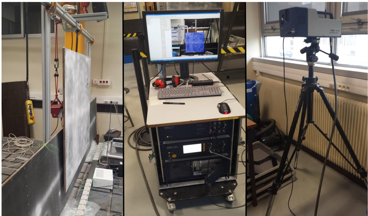
Figure 6.2: Testbed for the measurement of the displacement field of the sandwich panels.
