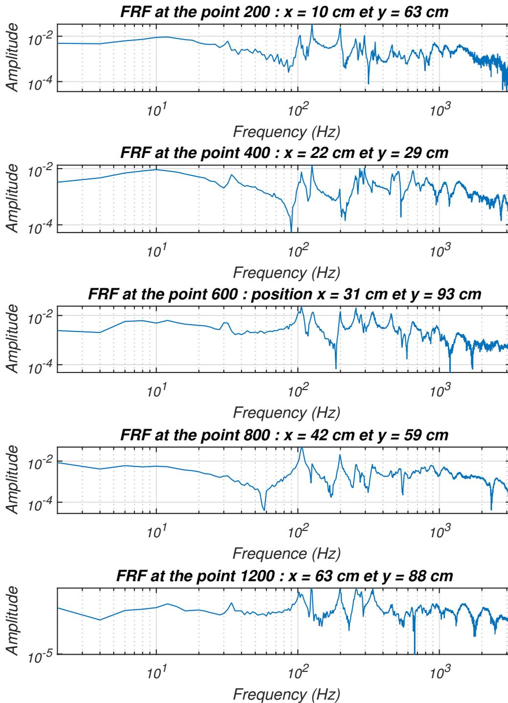
Figure A.2: Spatial FRF at different point for the panel A.
