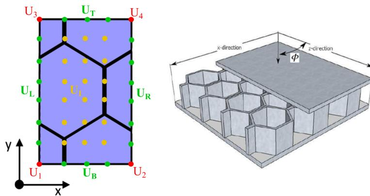
Figure 2.2: Nodes definition of the rectangular unit cell in the 2D WFE method.
