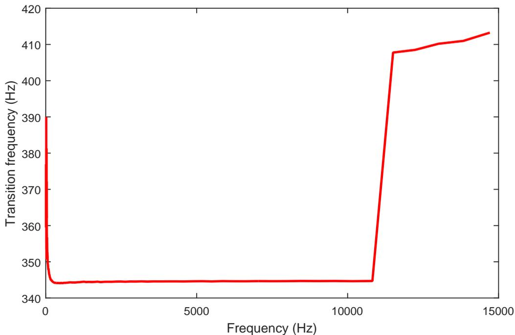
Figure 3.2: Effect of the selected frequency range on the predicted transition frequency.
