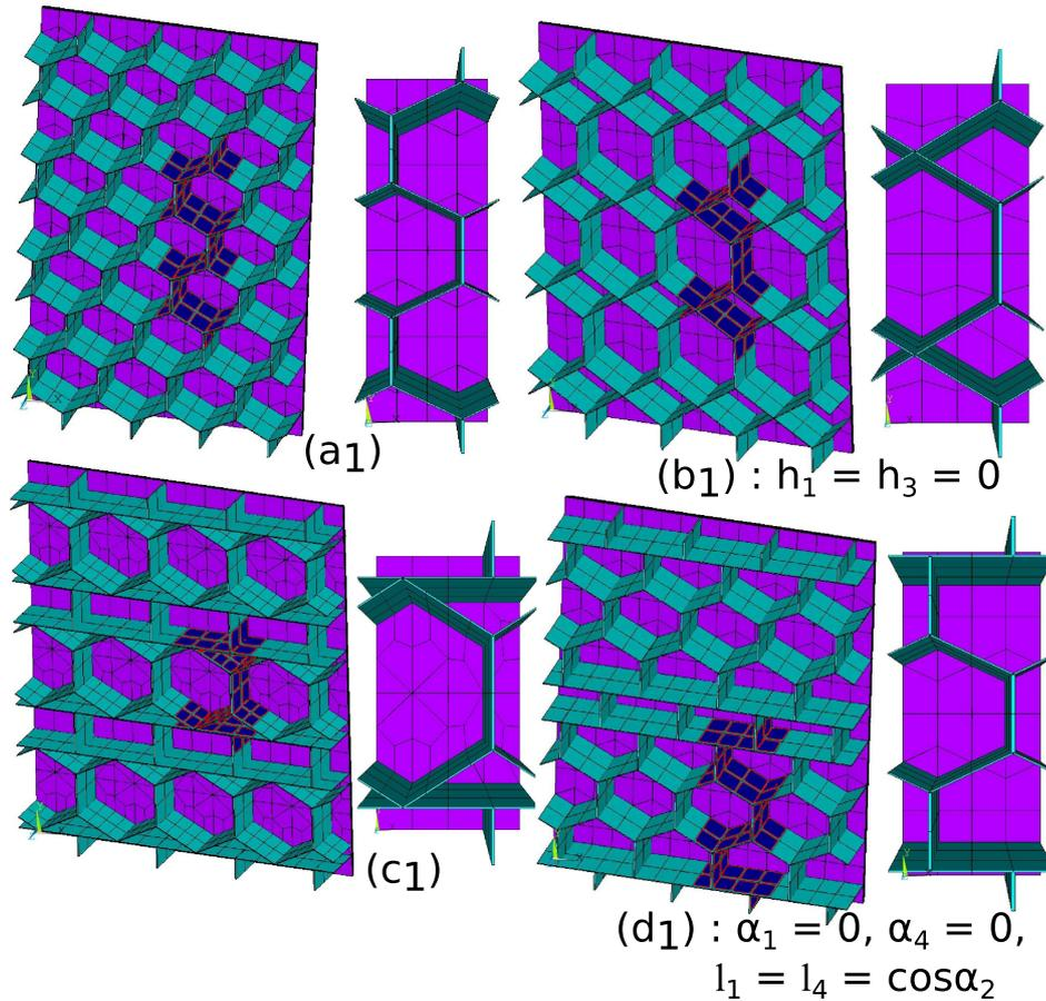
Figure 5.16: Studied core forms of the sandwich panels
