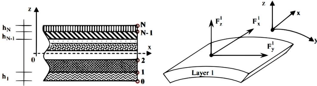
Figure 1.8: The interlayer forces considered in the DLM.
