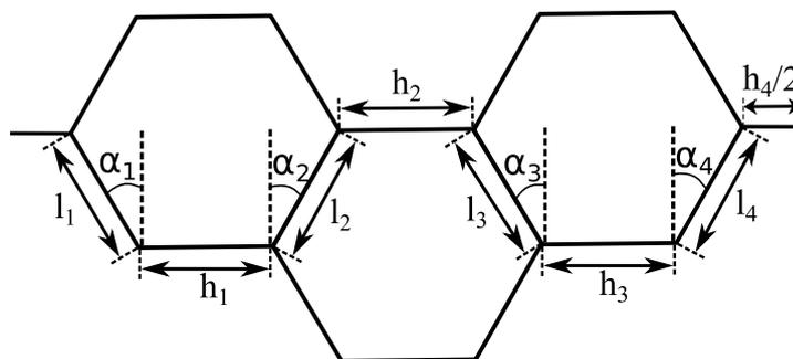
Figure 5.15: Studied core forms of the sandwich panels
