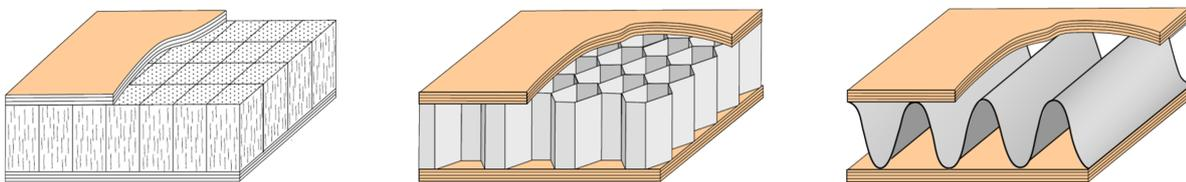
Figure 1.1: Different core configurations of a sandwich panel
