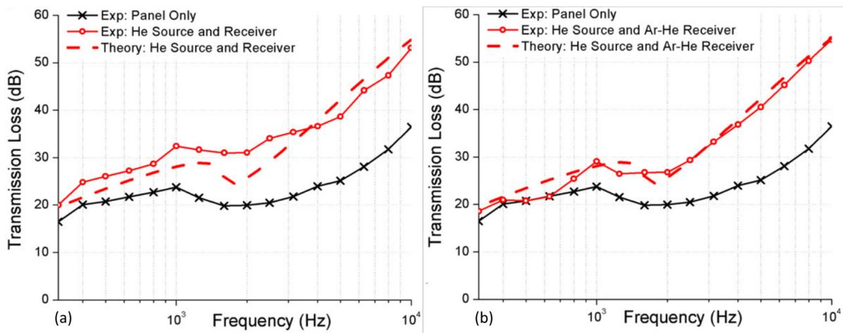
Figure 1.23: (a) Panel with helium layers on the source and receiver sides; (b) Panel with helium on the source side and argon and helium on the receiver side of the panel [103].
