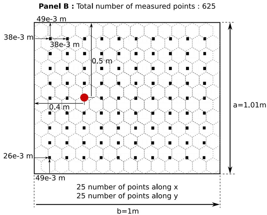
Figure 6.3: Mesh of the panels A and B.
