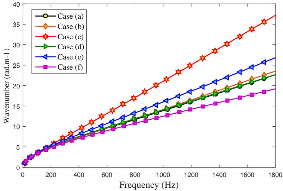
Figure 4.4: Flexural wavenumbers for the five core configurations.
