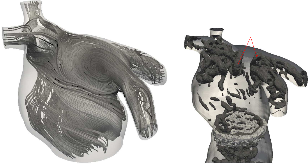
Figure 5.9: Left: streamlines in the atrium at 0.75T_a . Right, isosurface of Q-criterion ( 5\frac{u^2}{R^2} ) showing the structures present in the instantaneous field at 0.51T_a . Vortex rings are indicated by the two red arrows.
