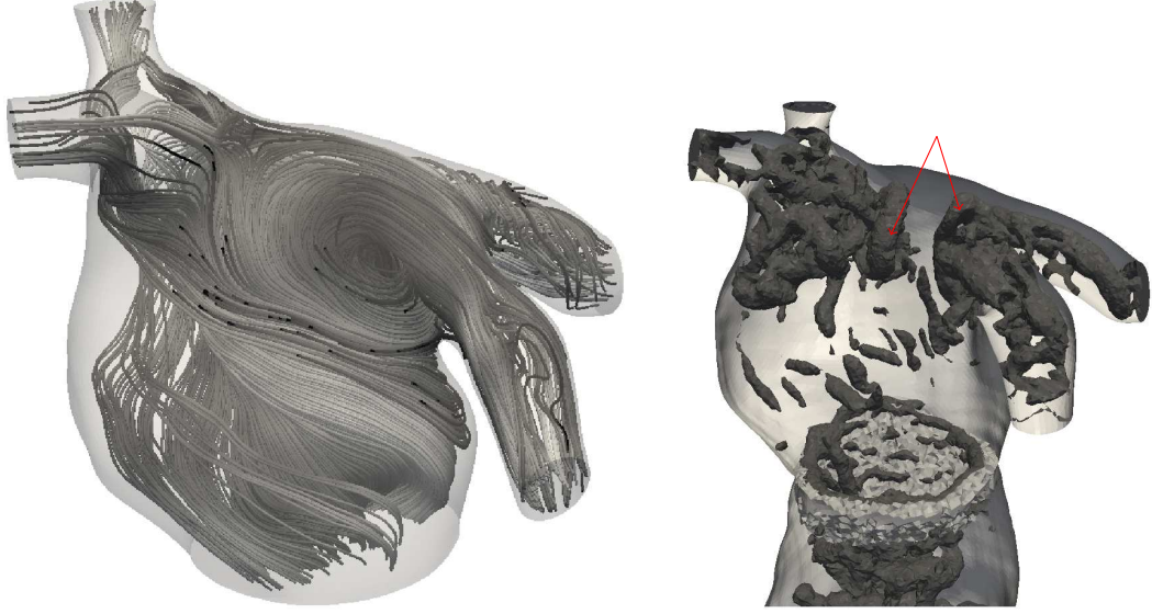
Figure 5.9: Left: streamlines in the atrium at 0.75T_a . Right, isosurface of Q-criterion ( 5\frac{u_a^2}{R_a^2} ) showing the structures present in the instantaneous field at 0.51T_a . Vortex rings are indicated by the two red arrows.
