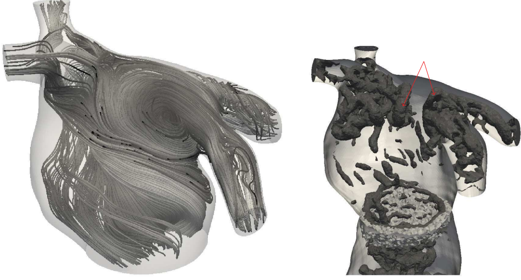
Figure 5.9: Left: streamlines in the atrium at 0.75T_a . Right, isosurface of Q-criterion ( 5 \frac{u_a^2}{R_q^2} ) showing the structures present in the instantaneous field at 0.51T_a . Vortex rings are indicated by the two red arrows.
