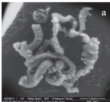
**Figure 3: SEM image of exfoliated graphite made of natural graphite by using formyl acid and microwave: Worm-like graphite under ESEM (Quanta 200F) [18].**
