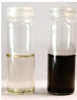
Figure 120: Suspensions of GO (left) and GO-APTMS (right) in toluene at a concentration of 0.1 mg/mL.
