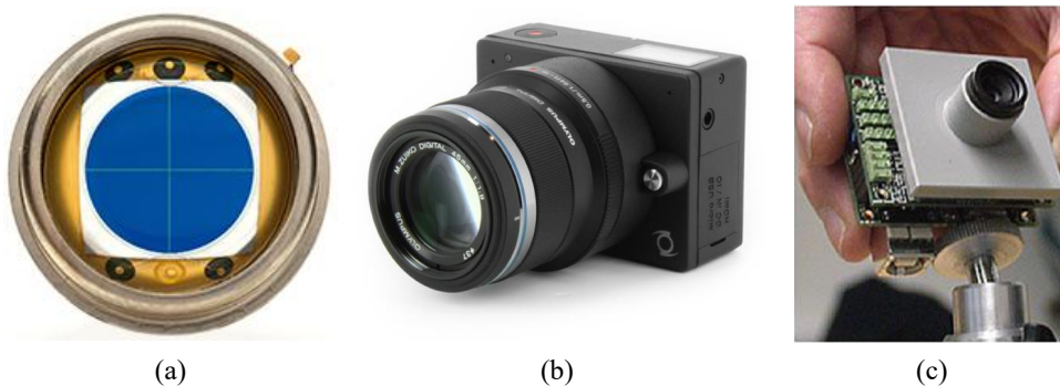
Figure 1.12: Photos of high-speed tracking instruments. (a) A photo of quadrant photodiodes (image from FirstSensor). (b) A photo of high-speed camera (image from E1 Camera). (c) A silicon retina prototype (ETHZ, Switzerland).
