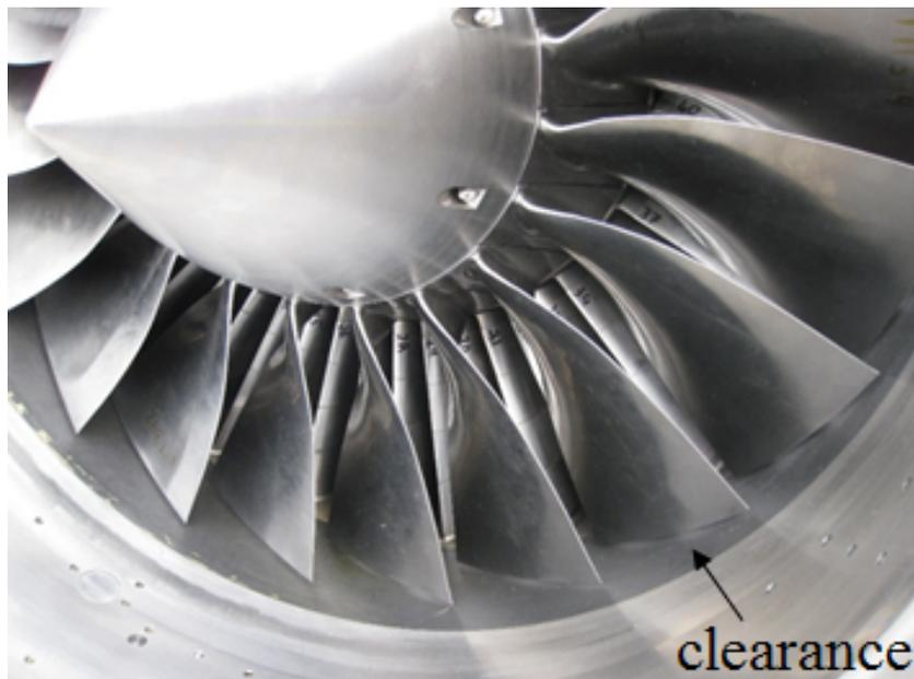
Fig. 1.1 Tip clearance in turbomachines.
