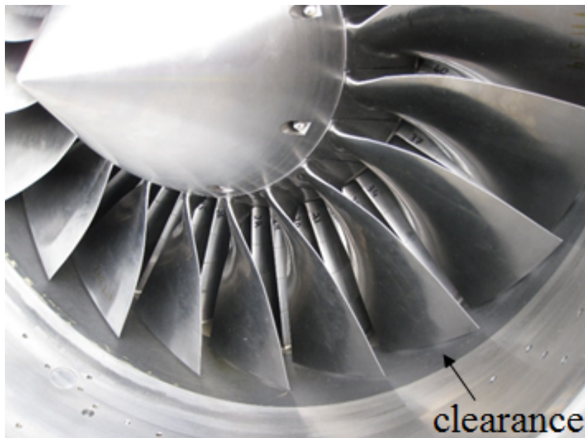
Fig. 1.1 Tip clearance in turbomachines.
