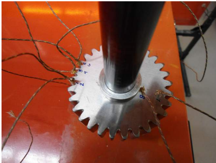
FIGURE A.6 – Placement des thermocouples.
