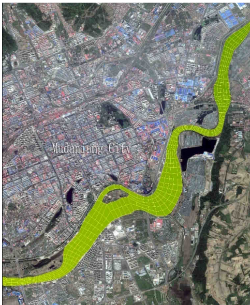
Figure 3-18. Grid division for urban section of the Mudan River trunk stream (part).
