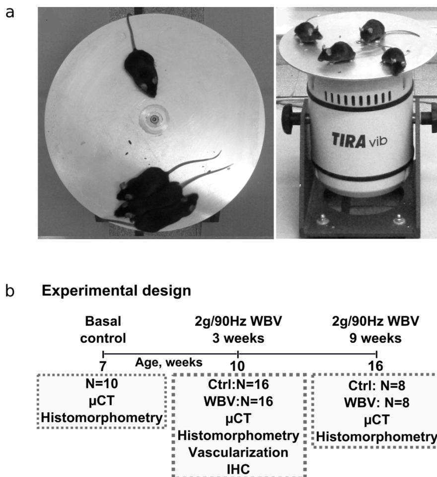
**Figure 1. Vibration device and a scheme of the experimental design.** a – descriptive photo of the vibration device during a vibration session; b - scheme of the experimental design, number of animals and performed analyses are listed for each group/experiment. Ctrl = control, WBV = whole body vibration.
