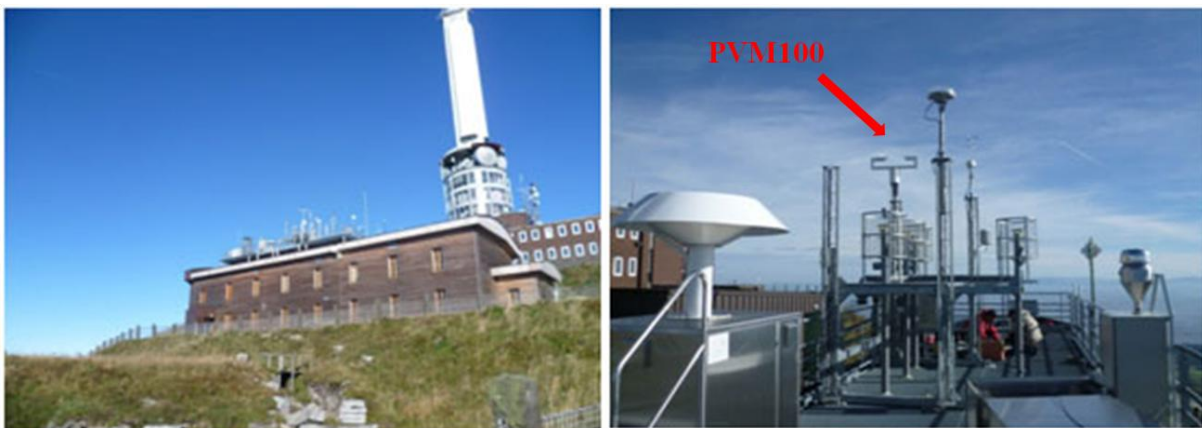
Figure 13: Puy de Dome atmospheric measurement station (left) and instruments set up on the roof (PVM100 in detail) (right).
