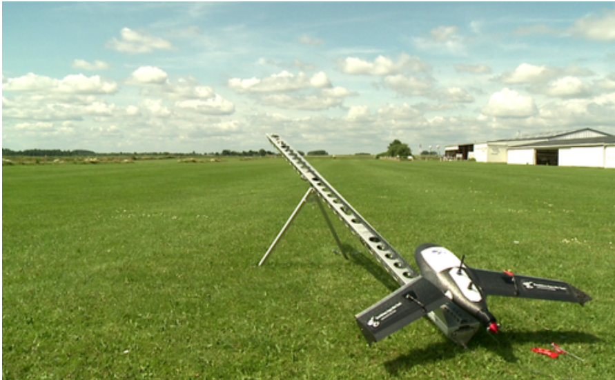
FIGURE 6: The small unmanned aerial system (UAS) Gatewing X100 on its launcher, ready for take-off.
