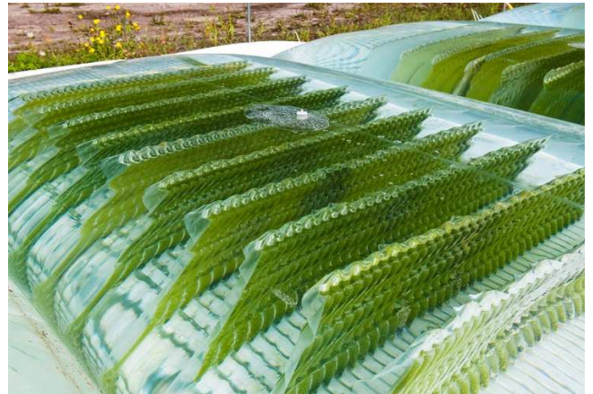
Figure 23 Flat panels immersed in water in Algae parc, Wageningen University, Netherlands. [60]
