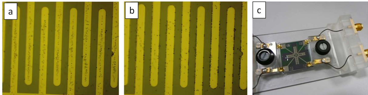
Figure 12 : Chlorella vulgaris cells in negative DEP at 50 kHz (a) and positive DEP at 100 kHz (b). Distance between the electrodes: 25 \mu\text{m} . (c) device used for the experiments. Electrodes in platinum, square chip in silicon (size: 2.5 x 2.5 \mu\text{m} )
