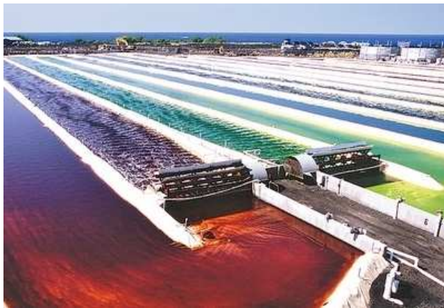
Figure 17: Dunaliella salina and Spirulina platensis cultivated in raceways, Cyanotech Hawaii[47]
