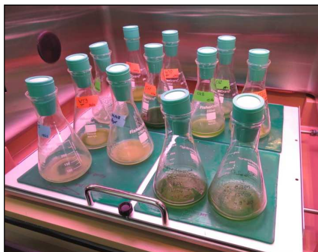
Figure 39: Maximum 50 mL of medium in 250 mL Erlenmeyer flasks. Culture at 24 \pm 1^\circ\text{C} , 20-40 \mu\text{mol} \cdot \text{m}^{-2} \cdot \text{s}^{-1} , 1.5 % CO 2 .
