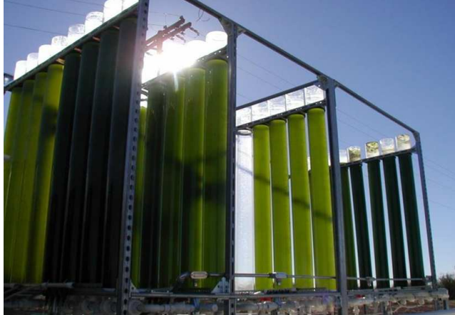
Figure 20 Vertical photobioreactors for microalgae cultivation [57]
