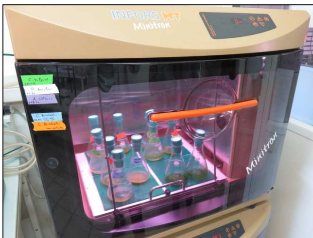
Figure 38: Minitron HT incubator used to grow algae
