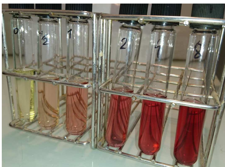
Figure 57: SPV colorations obtained for algae in 7 days of stress concentrated by a factor from 0.5 to 8 (from the left to the right).
