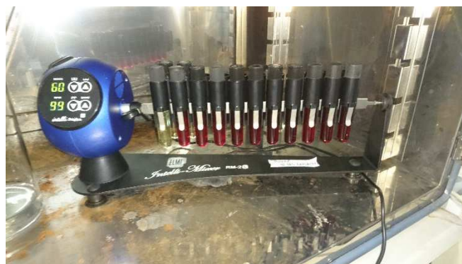
Figure 67: Mixing device (ELMI Intelli-Mixer, Mode 60, 99 Rpm) in a oven at 37°.
