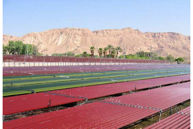
Figure 21 Haematococcus pluvialis cultivation via horizontal tubular reactors in Israel [58] for astaxantin production (red pigment)
