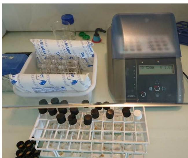
Figure 66: Tube heater (WTW CR3200) and ice cooling
