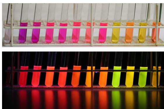
Figure 30: Nile red under visible and ultraviolet (366 nm) light un different solvents. From left to right: 1. water, 2. methanol, 3. ethanol, 4. acetonitrile, 5. dimethylformamide, 6. acetone, 7. ethyl acetate, 8. dichloromethane, 9. n-hexane, 10. methyl-tert-butylether, 11. cyclohexane, 12. toluene.
