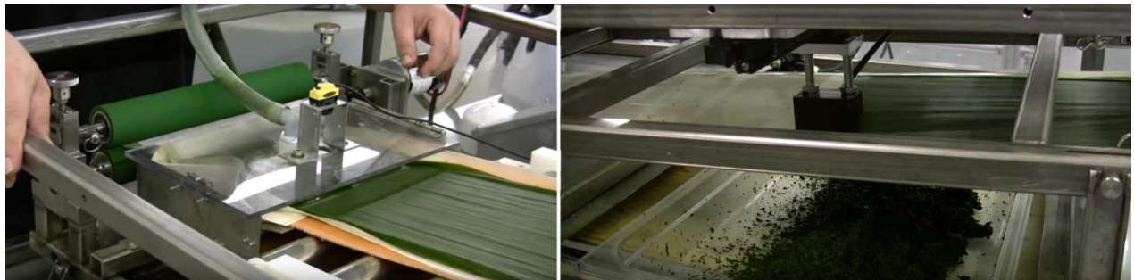
Figure 27: Solid liquid Separation pilot model dewatering microalgae from Algaeventure systems (roller drying)
