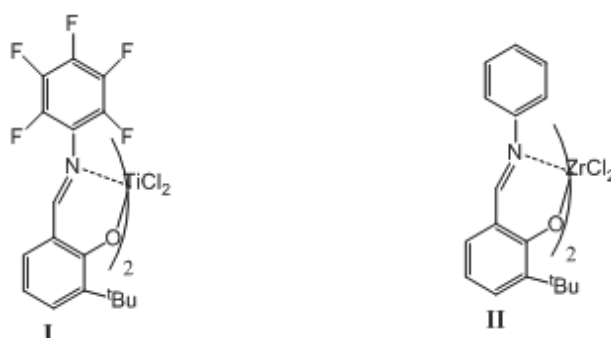
Figure 17. Bis(Phenoxy-imine) based complexes : species I [ N -(3- tert -butylsalicylidene)-2,3,4,5,6 pentafluoroanilinato] titanium dichloride ; species II [ N -(3- tert -butylsalicylidene)phenylaminato] zirconium dichloride
