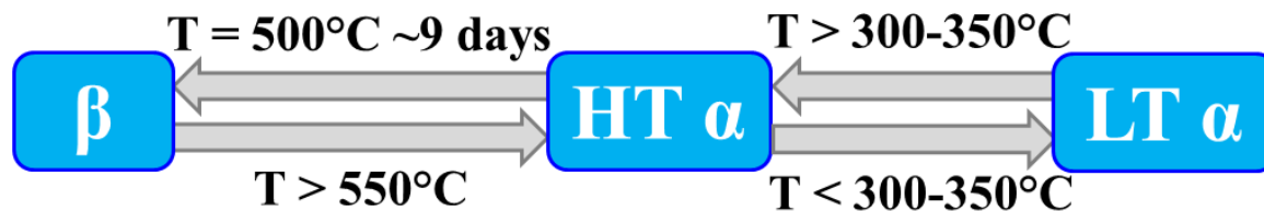
Figure 48: Schematic representation of the synthetic relationship different polymorphs of \text{Li}_6\text{CuB}_4\text{O}_{10} .
