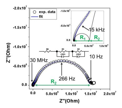
Figure 92: Representative AC complex impedance spectra of Bi<sub>4</sub>B<sub>2</sub>O<sub>9</sub> measured at 384°C in air. The semi circles corresponding to the bulk- and grain boundary resistance are schematically drawn as grey lines, and the real resistance values are indicated with green arrows.
