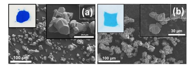
Figure 38: Representative SEM images of (a)  $\alpha$ -  $Li_6CuB_4O_{10}$  and (b)  $\beta$ -  $Li_6CuB_4O_{10}$ . Insets show a magnified view on the crystallites and a colored picture of the as-prepared powder.
