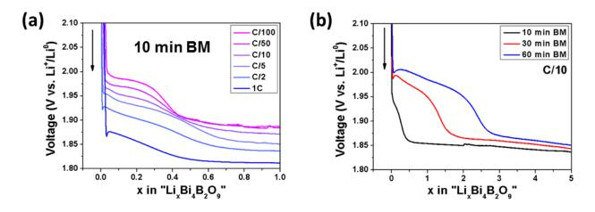
Figure 90: Initial discharge of  $Bi_4B_2O_9$  carbon composite. In (a) the influence of different C-rates is shown for a milling time of 10 min, whereas in (b) the impact of the milling time is presented.
