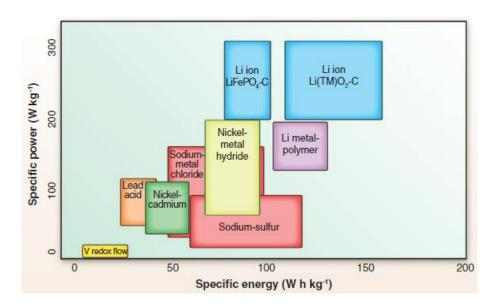
*Figure 6:* Comparison of different battery technologies in terms of their gravimetric and volumetric energy density.<sup>5</sup>
