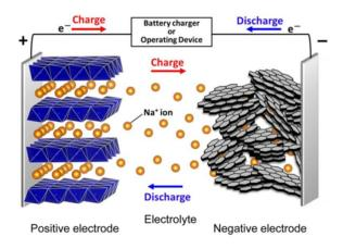
Figure 8: Schematic illustration of a Na-ion battery. 31
