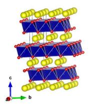
Figure 10: Schematic view of the crystal structures of layered LiCoO<sub>2</sub> with Li-, Co- and O atoms drawn in yellow, blue and red respectively.
