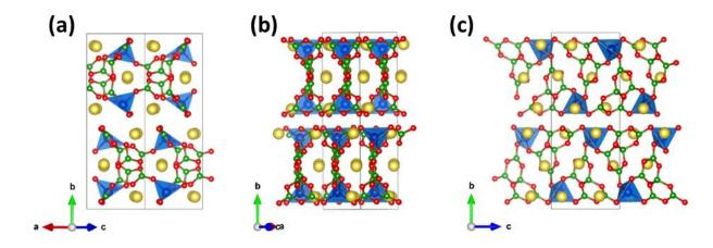
*Figure 66:* Structure of  $Na_3CoB_5O_{10}$  viewed along different crystallographic directions. Oxygen, boron, sodium and cobalt atoms indicated in red, green, yellow and blue respectively.
