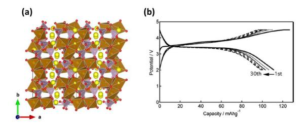
Figure 20: (a) Crystal structure of  $Li_2FeP_2O_7$  (Li in green,  $FeO_5$ ,  $FeO_6$  in brown and  $P_2O_7$  in purple) and (b) galvanostatic cycling vs. Li at a C/20 rate.<sup>86</sup>
