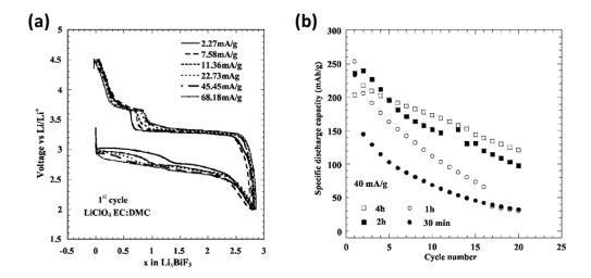
Figure 29: (a) Galvanostatic curve of  $BiF_3$  versus lithium for different current rates and (b) the capacity retention for ab  $BiF_3/C$  ball milled for different times composite with 20wt% carbon. <sup>121,125</sup>
