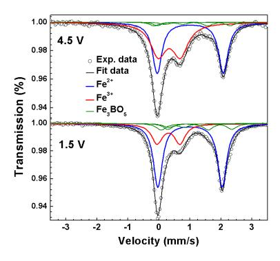
Figure 69: Room temperature ex situ Mössbauer spectra recorded for  $Na_3FeB_5O_{10}$  at 4.5 V (charged) and at 1.5 V (discharged).
