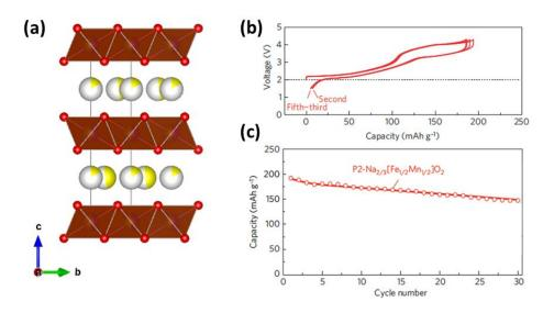
Figure 11: (a) Structure of the P2-Na<sub>2/3</sub>[ $Fe_{1/2}Mn_{1/2}$ ] $O_2$  its (b) galvanostatic cycling and the corresponding capacity retention.<sup>45</sup>
