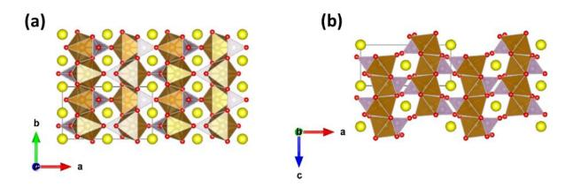
Figure 17: Structure of LiFePO<sub>4</sub> viewed along the (a) c- and the (b) b-axis. FeO<sub>6</sub> octahedras, PO<sub>4</sub> groups, oxygen and lithium atoms are represented in brown, purple, red and yellow.
