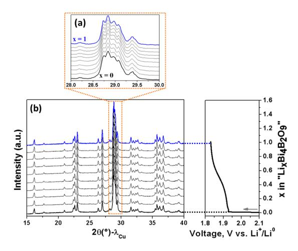
Figure 88: In situ XRD of the initial discharge of a  $Bi_4B_2O_9/Li$  half-cell cycled with a C/10 rate till a Li uptake of x = 1.0. XRD pattern were recorded each 0.1  $Li^+$ . A magnification of the main reflections is presented in (a) and an overview over the whole XRD pattern and the corresponding voltage-composition curve is shown in (b).
