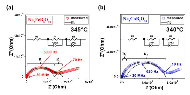
Figure 71: Representative complex impedance spectra of (a)  $Na_3FeB_5O_{10}$  and (b)  $Na_3CoB_5O_{10}$  recorded at 345 and 340°C respectively. The equivalent circuits are shown as inset, and the corresponding bulk  $(R_1)$  - and grain boundary  $(R_2)$  resistance are shown schematically as grey semicircles.
