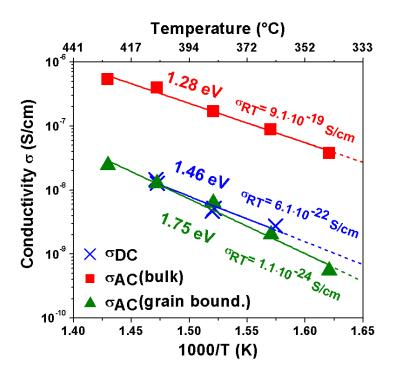
**Figure 94:** Arrhenius plot of the AC and DC conductivity of  $Bi_4B_2O_9$  derived in the temperature range from around 340 to 430°C during heating in air.
