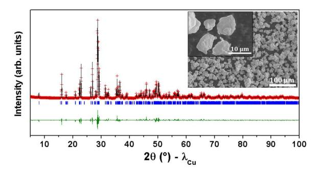
Figure 74: XRD pattern and Rietveld refinement of Bi<sub>4</sub>B<sub>2</sub>O<sub>9</sub>. Observed, calculated pattern and their difference are shown as red crosses, black- and green line respectively. Bragg reflections are indicated as vertical blue bars. The inset show a representative SEM image of the as synthesized compound with two different magnifications.
