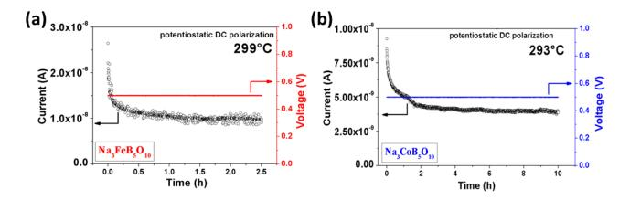
Figure 72: Representative potentiostatic DC polarization of (a)  $Na_3FeB_5O_{10}$  and (b)  $Na_3CoB_5O_{10}$  recorded at 299 and 293°C respectively.
