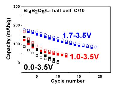
Figure 85: (Capacity retention of  $Bi_4B_2O_9$  mixed for 10 min with 5 wt% carbon and cycled with a C/10 rate in different potential window indicated in the plot. To have a better overview, the first discharge/charge capacities are excluded.
