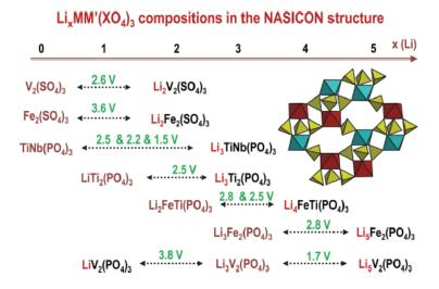
**Figure 16:** Different NASICON-type compounds with a  $Li_xMM'(XO_4)_3$  composition and different  $M^{(n+1)+}/M^{n+}$  redox couples.<sup>72</sup>
