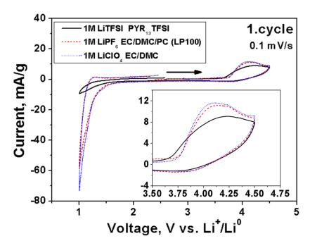
Figure 49: Cyclic voltammetry of  $\alpha$ -Li<sub>6</sub>CuB<sub>4</sub>O<sub>10</sub>/Li half cells in a potential window from 4.5 to 1.0 V during the first cycle.
