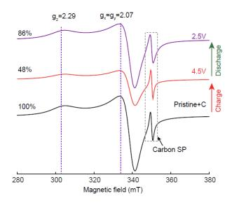
Figure 51: Room temperature EPR spectra of  $\alpha$ -Li<sub>6</sub>CuB<sub>4</sub>O<sub>10</sub> ball-milled with carbon at pristine (black), charged (4.5 V, red) and discharged (2.5 V, purple) states.
