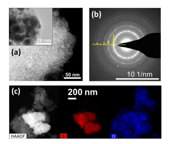
Figure 78:  $Bi_4B_2O_9/C$  sample discharged to 1.0 V. (a) Representative TEM image, (b) SAED pattern of the nanoparticles with the simulated diffraction profile of  $\alpha$ -Bi shown for comparison and (c) another TEM image and the corresponding EDX map of bismuth (red) and oxygen (blue).
