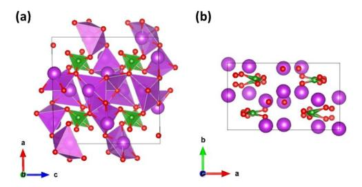
**Figure 75:** Crystal structure of  $Bi_4B_2O_9$  shown along the (a) b- and (b) c-axis. Bismuth atoms/polyhedral, boron and oxygen are shown in purple, green and red respectively.
