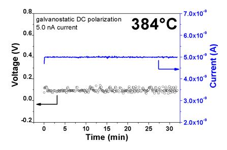
*Figure 93:* Representative galvanostatic DC polarization of  $Bi_4B_2O_9$ .
