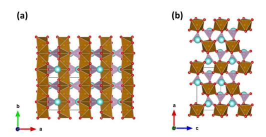
Figure 19: Structure of maricite NaFePO<sub>4</sub> along the (a) c- and (b) b-axis. FeO<sub>6</sub> octahedra, PO<sub>4</sub> tetrahedra, oxygen- and sodium-atoms are represented in brown, purple, red and blue respectively.
