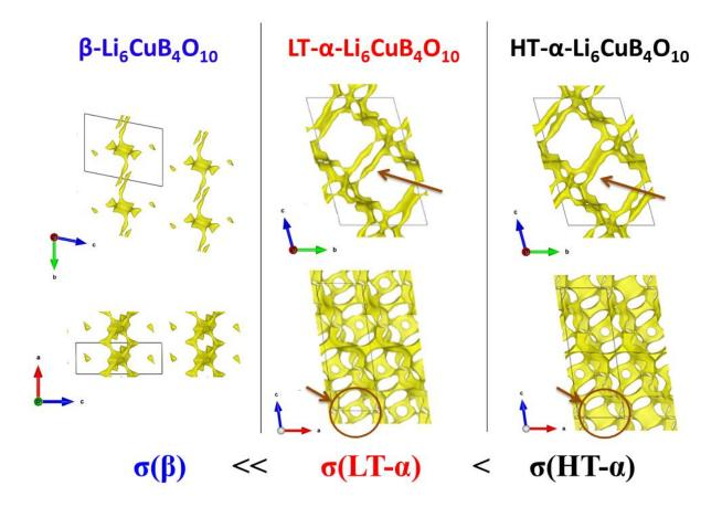
Figure 57: Bond valence energy landscape (BVEL) for the different polymorphs of  $Li_6CuB_4O_{10}$ , LT-and HT refers to the Low- and high-temperature form of  $\alpha$ - $Li_6CuB_4O_{10}$ . The energy values chosen for the plots are 1.0 eV above the minimum energy. Iso-energy yellow domains indicate paths for Li conduction. Slight differences in the Li conduction pathways between the LT and HT form of  $\alpha$ - $Li_6CuB_4O_{10}$  are marked with brown arrow and circles.
