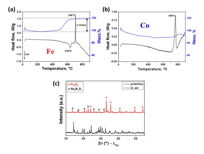
Figure 67: TGA-DSC curves of (a)  $Na_3FeB_5O_{10}$  and (c)  $Na_3CoB_5O_{10}$  recorded in air flow with a heating rate of 5°C/min. (c) XRD patterns of  $Na_3FeB_5O_{10}$  taken before and after annealing for 12h at 650°C in air.
