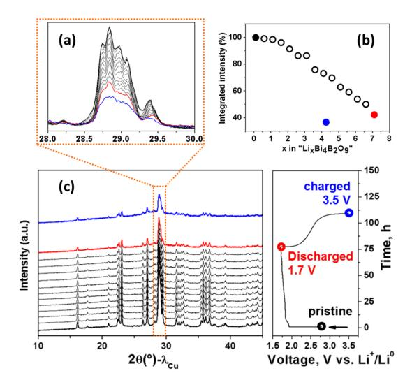
Figure 89: In situ XRD of the initial discharge/charge cycle of a Bi<sub>4</sub>B<sub>2</sub>O<sub>9</sub>/Li half-cell cycled with a C/10 rate in a potential window between 1.7 and 3.5 V. XRD pattern were recorded each 0.1 Li<sup>+</sup>, however for reasons of clarity only each 5<sup>th</sup> pattern is shown in (c). A magnification of the main reflections is presented in (a) and their integrated intensity of the main reflection is shown in (b).
