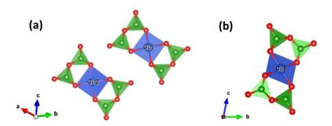
**Figure 41:** View of the  $[Cu(B_2O_5)_2]^6$  structural unit in (a)  $\alpha$ -Li<sub>6</sub>CuB<sub>4</sub>O<sub>10</sub> (Cu1 and Cu2) and (b)  $\beta$ -Li<sub>6</sub>CuB<sub>4</sub>O<sub>10</sub> (Cu1). Copper, boron and oxygen atoms are shown in blue, green and red respectively.
