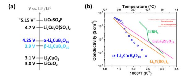
Figure 61: (a) Schematic illustration of the  $Cu^{3+}/Cu^{2+}$  redox potentials versus Li for different compounds including  $\alpha$ - and  $\beta$ -Li<sub>6</sub>CuB<sub>4</sub>O<sub>10</sub>. Note that the potential in quotation marks was derived from DFT calculations but never experimentally observed. (b) Comparison of the ionic conductivity of  $\alpha$ -Li<sub>6</sub>CuB<sub>4</sub>O<sub>10</sub> with different borate based materials and a Garnet type solid electrolyte.
