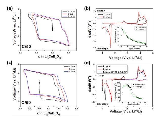
Figure 54: Voltage composition curve (a) and (c) and the corresponding derivative plot (b) and (d) for galvanostatic cycling of  $\alpha$ -Li<sub>6</sub>CuB<sub>4</sub>O<sub>10</sub> in a potential window from 4.5 to 1.0 V started either upon oxidation or reduction. The specific charge and discharge capacities versus cycle number are given in the insets of (b) and (d).
