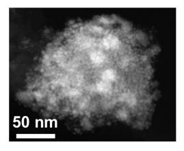
Figure 81: TEM image of a Bi<sub>4</sub>B<sub>2</sub>O<sub>9</sub>/C sample discharged to 1.0 V and recharged to 3.5 V.
