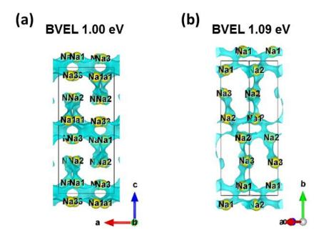
Figure 70: Bond valence energy landscape (BVEL) of (a)  $Na_3FeB_5O_{10}$  and (b)  $Na_3CoB_5O_{10}$ . The percolation energies are given in the figure. Iso-energy blue domains indicate paths for Na (yellow spheres) conduction.
