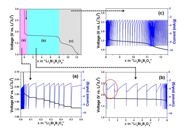
Figure 87: PITT measurement of  $Bi_4B_2O_9$  during the initial discharge down to 1.0 V. The red ellipses point out the chronoamperometry bell-shaped response.
