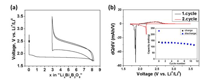
Figure 82: (a) Voltage-composition curves and (b) the corresponding derivative plots and capacity retention of a  $Bi_4B_2O_9/Li$  half-cell cycled between 1.7 and 3.5 V.
