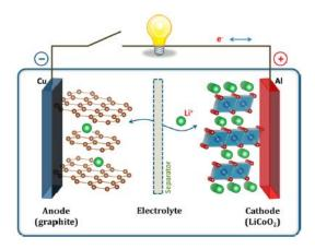
Figure 7: Schematic view of a Li-ion cell based on a LiCoO<sub>2</sub> cathode and a graphite anode.<sup>14</sup>
