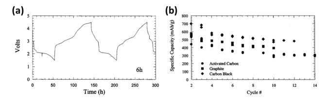
Figure 28: (a) Voltage versus time curve of a FeF<sub>3</sub>-activated carbon nanocomposite ball milled for 6h and (b) the corresponding capacity retention for different kind of carbon.  $^{120}$
