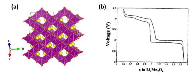
Figure 12: (a) Structure of the spinel  $LiMn_2O_4$  where  $MnO_6$  octahedra, lithium- and oxygen atoms are shown in purple, yellow and red respectively. (b) Voltage-composition curve of  $LixMn_2O_4$  for 0 < x < 2.<sup>50</sup>
