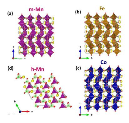
Figure 31: Crystal structures of LiMBO<sub>3</sub> for (a) M = Mn (monoclinic), (b) Fe, (c) Co and (d) Mn (hexagonal). Oxygen, lithium and boron atoms are shown in red, yellow and green respectively.
