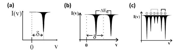
Figure 101: The energy changes are different in the source (S) and absorber (A) as a result of different electron densities at the source and absorber nuclei, the result is manifested as isomer shift in the Mössbauer spectrum.<sup>247</sup>
