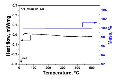
**Figure 76:** TGA-DSC curve of  $Bi_4B_2O_9$  recorded in air from RT to 500°C during heating under air flow.
