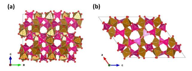
**Figure 14:** Crystal structure of the NASICON type compound  $Fe_2(MoO_4)_3$  along the (a) a- and (b) b-axis.  $FeO_6$  octahedra and  $MoO_4$  tetrahedra are shown in brown and purple respectively.
