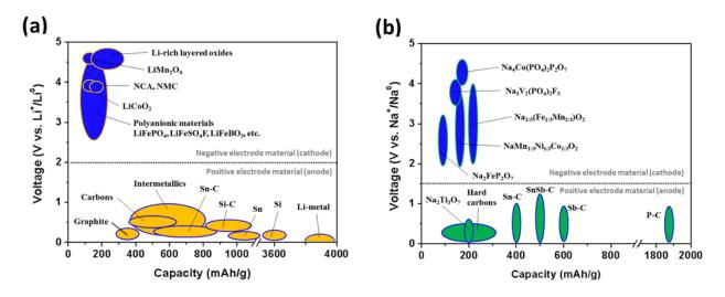
*Figure 9:* Overview of different positive and negative electrode materials for (a) Li-ion and (b) Na-ion batteries, with respect to their redox potential and theoretical capacity. 11,16,34
