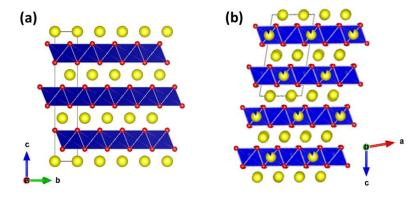
Figure 13: Layered structures of (a) LiMO<sub>2</sub> (M = Co, Ni, Mn) and (b) Li<sub>2</sub>MnO<sub>3</sub>.<sup>62</sup>
