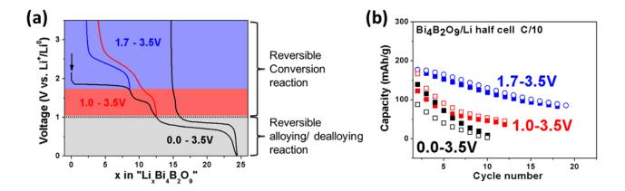
Figure 95: (a) Schematic illustration of the different voltage-composition curve of Bi<sub>4</sub>B<sub>2</sub>O<sub>9</sub> versus Li depending on the lower cutoff potential referring to the conversion- and alloying part of the electrochemical reaction versus Li. (b) Capacity retention depending on the voltage window applied for galvanostatic cycling.
