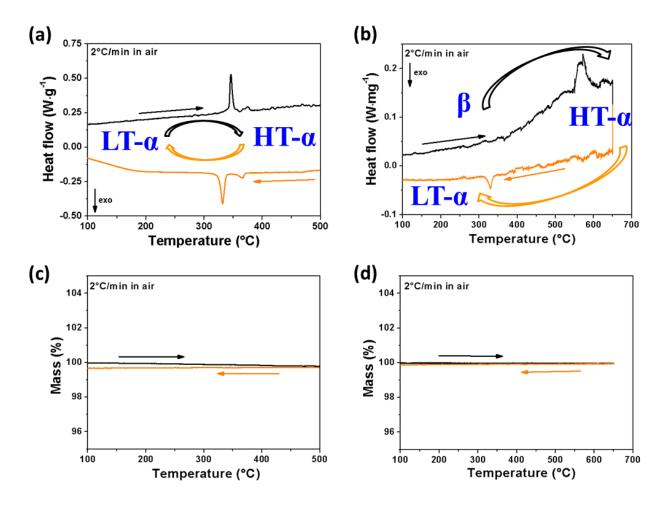
**Figure 43:** DSC and TGA curve for (a,c)  $\alpha$ - and (b,d)  $\beta$ -Li<sub>6</sub>CuB<sub>4</sub>O<sub>10</sub> respectively. The black- and the orange line are recorded during heating and cooling respectively. LT- and HT- refers to the low temperature- and high temperature form of  $\alpha$ -Li<sub>6</sub>CuB<sub>4</sub>O<sub>10</sub>.
