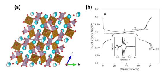
Figure 21: (a) Crystal structure of  $Na_2FeP_2O_7$  (Na in yellow,  $FeO_6$  in green and  $P_2O_7$  in purple. (b)
