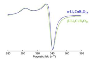
Figure 39: EPR spectra recorded at room temperature for both polymorphs of Li<sub>6</sub>CuB<sub>4</sub>O<sub>10</sub>.
