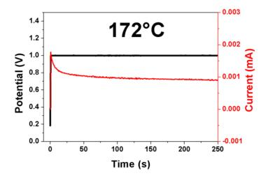
*Figure 59:* (a) DC polarization of a pellet of  $\alpha$ -Li<sub>6</sub>CuB<sub>4</sub>O<sub>10</sub> with 1.0 V at 172°C using Pt-electrodes.
