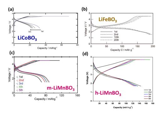
Figure 33: Galvanostatic charge-discharge curves for (a) LiCoBO3, <sup>140</sup> (b) LiFeBO3, <sup>139</sup> (c) m-LiMnBO3<sup>141</sup> and (d) h-LiMnBO3<sup>144</sup> cycled at a C/20 rate versus lithium.
