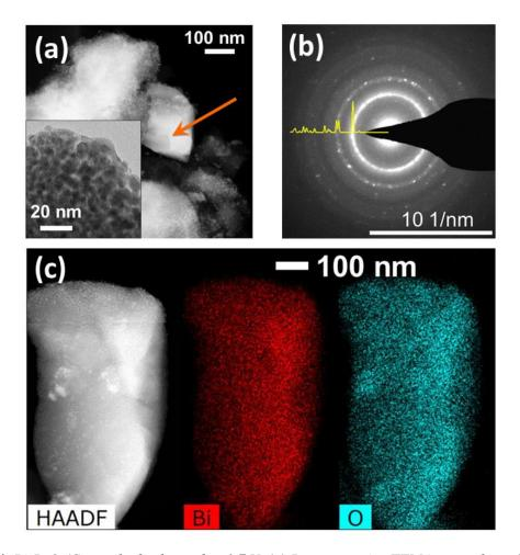
Figure 84: Bi<sub>4</sub>B<sub>2</sub>O<sub>9</sub>/C sample discharged to 1.7 V. (a) Representative TEM image where the orange arrow indicates large particle of not reacted Bi<sub>4</sub>B<sub>2</sub>O<sub>9</sub>. (b) SAED pattern of the nanoparticles with the simulated diffraction profile of α-Bi shown for comparison and (c) another TEM image and the corresponding EDX map of bismuth (red) and oxygen (cyan).
