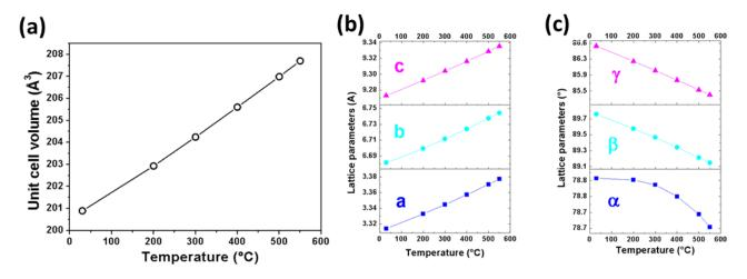
Figure 47: Change of the lattice parameters of β-Li<sub>6</sub>CuB<sub>4</sub>O<sub>10</sub> with temperature. (a) Shows the evolution of the unit cell volume, (b) unit cell edges and (c) the unit cell angles.
