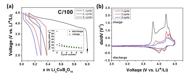
Figure 50: (a) Voltage-composition curve and (b) the corresponding derivative plot for  $\alpha$ -Li<sub>6</sub>CuB<sub>4</sub>O<sub>10</sub> vs. Li. Inset in (a) shows the capacity retention.
