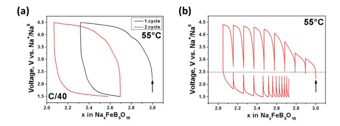
Figure 68: (a) Voltage-composition curve of  $Na_3FeB_5O_{10}$  versus Na cycled at a C/40 rate between 4.5 and 1.5 V vs.  $Na^+/Na^0$  at 55°C. (b) GITT measurement with 4 h current pulse and 12 h open circuit voltage (OCV) period during the first charge and discharge.
