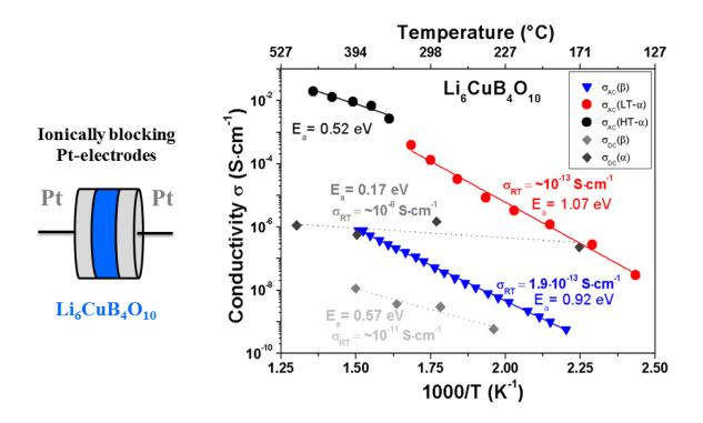
Figure 60: Arrhenius plot of the AC- and DC conductivity of  $\alpha$ - and  $\beta$ -Li<sub>6</sub>CuB<sub>4</sub>O<sub>10</sub> and a schematic view of the sample pellet between two ionically blocking Pt-electrodes used for AC- as well as for DC measurements.
