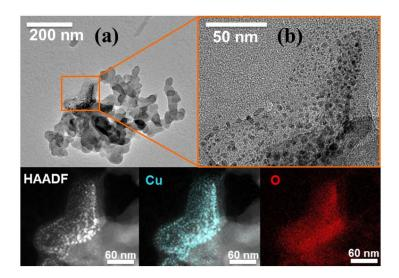
Figure 55: TEM image of  $\alpha$ -Li<sub>6</sub>CuB<sub>4</sub>O<sub>10</sub> carbon composite discharged to 1.0 V. (a) shows an overview of agglomerated particles whereas (b) highlights one particle where copper nanograins can be seen on the surface, as confirmed by the corresponding EDS mapping shown below for copper (pale blue) and oxygen (red).
