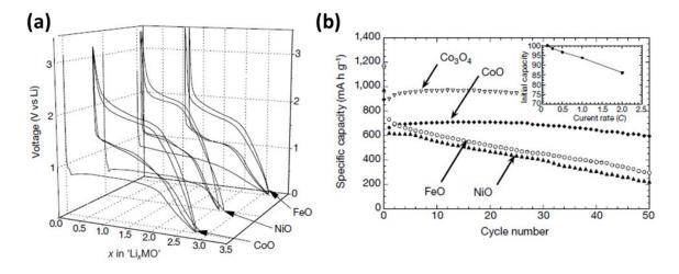
Figure 27: (a) Voltage composition curves for different TM oxides and (b) the corresponding capacity retention.  $Co_3O_4$  is shown to proof that not only divalent TM oxides can be applied. The inset show the rate capability of CoO.
