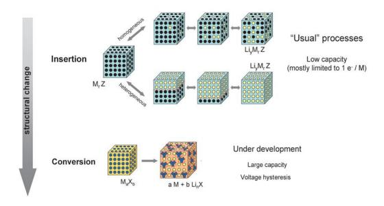
**Figure 26:** Schematic illustration of insertion and conversion type reaction investigated as electrode materials for Li- and Na-ion batteries. <sup>15</sup>
