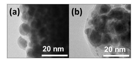
Figure 86: Typical HRTEM images of the active material discharged at (a) 1.7 V and (b) 1.0 V.
