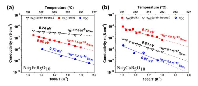
Figure 73: Arrhenius plot of the AC and DC conductivity of (a)  $Na_3FeB_5O_{10}$  and (b)  $Na_3CoB_5O_{10}$  derived in the temperature range from around 250 to 400°C during heating in argon flow.
