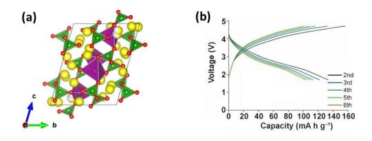
Figure 34: (a) Structure of  $Li_7Mn(BO_3)_3$  viewed along the a-axis. Oxygen, lithium boron and manganese are represented in red, yellow, green and purple respectively. (b) Galvanostatic charge-discharge curve for  $Li_7Mn(BO_3)_3$  between 4.7 and 1.7 V vs.  $Li^+/Li^0$  with 10 mA/g. <sup>153</sup>
