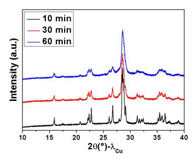
*Figure 91:* XRD pattern of  $Bi_4B_2O_9$  ball milled for different times with 5 wt% carbon.
