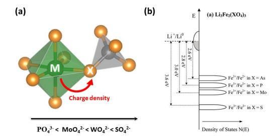
Figure 15: Schematic representation of the inductive effect. (a)  $MO_6$  octahedra connected over one bridging oxygen to the  $XO_4$  tetrahedra. (b) Depending on the electronegativity of the polyanionic group, the redox potential of the  $Fe^{3+}/Fe^{2+}$  can be shifted up from 2.8 to 3.6 V vs.  $Li^+/Li^{0.71}$
