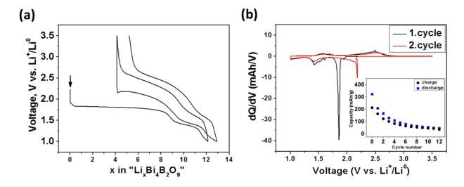
Figure 80: (a) Voltage-composition curves and (b) the corresponding derivative plots and capacity retention of a  $Bi_4B_2O_9/Li$  half-cell cycled between 1.0 and 3.5 V.
