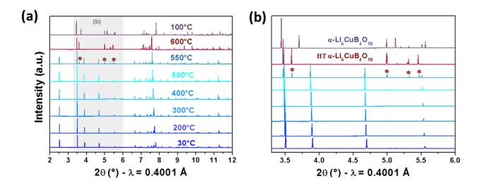
Figure 46: (a) In situ synchrotron XRD pattern for  $\beta$ -Li<sub>6</sub>CuB<sub>4</sub>O<sub>10</sub> during heating up to 600°C and after cooled down to room temperature with (b) a magnification of the grey shaded region marked in (a). The brown asterisks mark the appearance of reflections from the HT  $\alpha$ -Li<sub>6</sub>CuB<sub>4</sub>O<sub>10</sub> phase.
