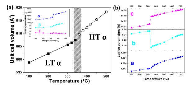
Figure 45: Change in lattice parameters as a function of temperature for α-Li<sub>6</sub>CuB<sub>4</sub>O<sub>10</sub> during heating as derived from in situ high temperature XRD. The grey shaded bar marks the temperature region where the structural transition from the LT- to the HT α-Li<sub>6</sub>CuB<sub>4</sub>O<sub>10</sub> occurs. (a) Volume of the unit cell and angles shown in the inset. (b) Variation of unit cell parameters.
