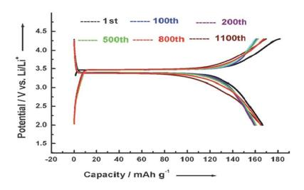
Figure 18: Voltage-composition curve for galvanostatic cycling of carbon coated LiFePO<sub>4</sub>. <sup>74</sup>
