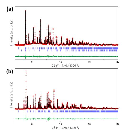
Figure 63: Synchrotron XRD pattern and the corresponding Rietveld refinement of (a)  $Na_3FeB_5O_{10}$  and (b)  $Na_3CoB_5O_{10}$ . The red crosses, black-, and green line represent the observed, calculated and difference patterns, respectively. The positions of the Bragg reflections are shown as vertical blue bars. For  $Na_3FeB_5O_{10}$ , the lower set of tick marks is  $Fe_3BO_5$  (~4 w%).
