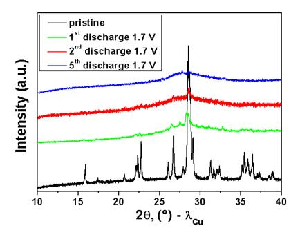
*Figure 83:* XRD pattern of  $Bi_4B_2O_9$  discharged to 1.7 V after the first, second and fifth cycle.
