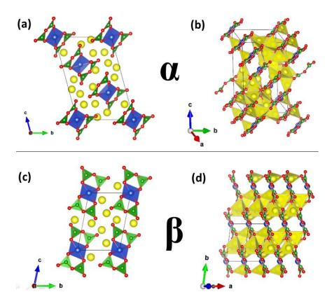
Figure 42: Structure of (a, b)  $\alpha$ - and (c, d)  $\beta$ -  $Li_6CuB_4O_{10}$  along different crystallographic directions. Copper, boron and oxygen are drawn in blue, green and red. Li, Cu, B and O atoms are drawn in yellow, blue, green and red respectively.
