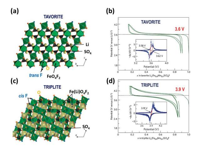
Figure 25 (a,c) Structure and (b,d) galvanostatic charge-discharge curves for tavorite- and triplite  $LiFeSO_4F$ . 111
