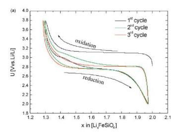
*Figure 23:* Voltage-composition curve of Li<sub>2</sub>FeSiO<sub>4</sub> versus lithium at a C/20 rate. <sup>100</sup>
