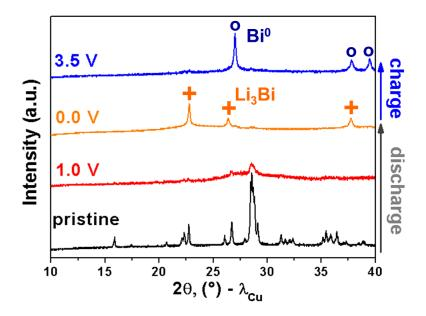
Figure 79: XRD pattern of  $Bi_4B_2O_9$  discharged to 1.0 and 0.0 V and after the subsequent charge to 3.5V.
