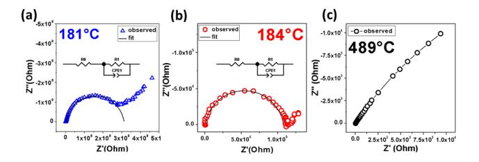
Figure 58: Complex AC impedance spectra for (a)  $\beta$ -, (b) LT  $\alpha$ - and (c) HT  $\alpha$ -Li<sub>6</sub>CuB<sub>4</sub>O<sub>10</sub>. The equivalent circuit shown as inset was used to fit the spectra, whereas in the case of (c) the interception with the x-axis was taken as R1.
