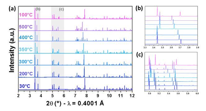
Figure 44: In situ synchrotron XRD pattern for  $\alpha$ -Li<sub>6</sub>CuB<sub>4</sub>O<sub>10</sub> during heating up to 500°C and after cooled down to 100°C. A global view is given in (a) while (b) and (c) highlight the grey marked areas.
