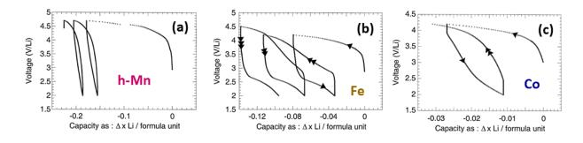
Figure 32: Voltage composition curve of LiMBO<sub>3</sub> cycled with different C-rates for (a) hexagonal-Mn, C/60, (b) Fe, C/250 and (c) Co, C/100.<sup>138</sup>
