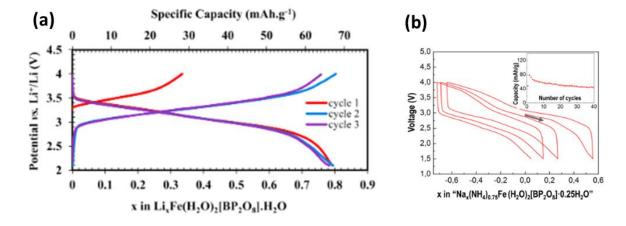
Figure 35: (a) Galvanostatic charge/ discharge curve of  $Li_{0.8}Fe(H_2O)_2[BP_2O_8] \cdot H_2O$  versus lithium and (b) voltage composition curve of  $(NH_4)_{0.75}Fe(H_2O)2[BP_2O_8] \cdot 0.25H_2O$  versus sodium.  $^{162,163}$
