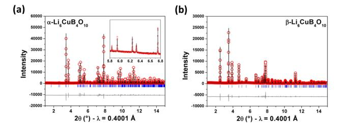
Figure 40: Rietveld refinement of the synchrotron XRD pattern of (a)  $\alpha$ - and (b)  $\beta$ - Li<sub>6</sub>CuB<sub>4</sub>O<sub>10</sub>. The red circles, black line and the bottom grey line represent the observed, calculated and difference pattern respectively. Bragg positions are marked with blue vertical thick bars.
