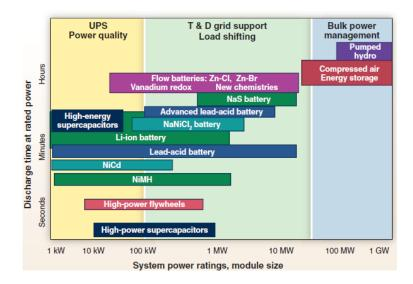
*Figure 3:* Comparison of discharge time and power rating for various electrochemical energy storage technologies.<sup>5</sup>
