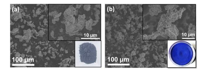
Figure 62: SEM images of (a)  $Na_3FeB_5O_{10}$  and (b)  $Na_3CoB_5O_{10}$ .
