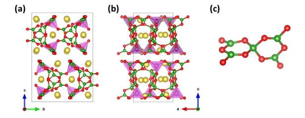
Figure 64: Structure of  $Na_3FeB_5O_{10}$  viewed along the a-axis (a) and the b-axis (b). Oxygen, boron, sodium and iron atoms indicated in red, green, yellow and pink respectively. (c) Pentaborate unit.
