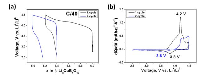
Figure 56: (a) Typical voltage composition curve and (b) the corresponding derivative plot of  $\beta$ - $Li_6CuB_4O_{10} \text{ vs. Li at a C/40 rate.}$
