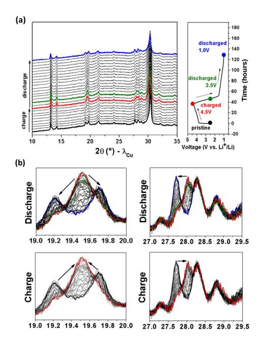
**Figure 53:** (a) In situ XRD patterns during charge and subsequent discharge in relation to the voltage versus time curve. (b) The reversible changes of the reflections indicated centered around 19.5 and 25.0°.
