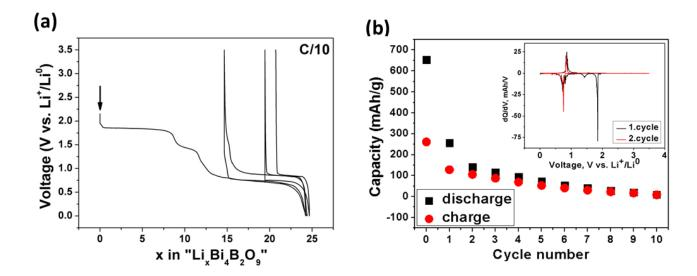
Figure 77: (a) Voltage-composition curve of  $Bi_4B_2O_9/Li$  half-cell and (b) the capacity retention and the corresponding derivative plot of voltage-composition curve is show as inset.
