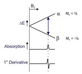
Figure 100: Energy levels for an electron with spin  $(S = \pm 1/2)$  in an applied magnetic field B, where it can adopt two different states  $(\alpha$  and  $\beta)$ , and the corresponding absorption spectrum and its first derivative.
