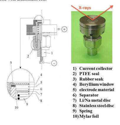
Figure 97: Schematic view of a modified Swagelok type 2 electrode cell used for I situ XRD experiments.
